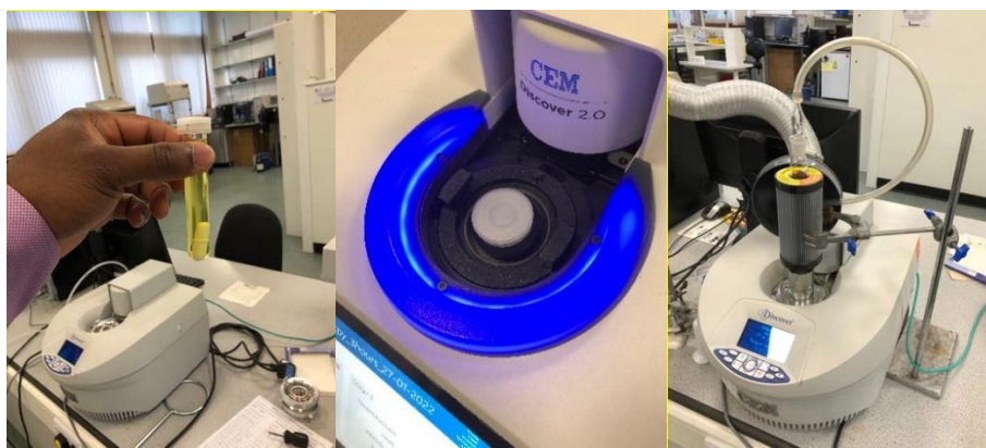
Figure 2.8 – Microwave setup showing a 10mL microwave vial with a magnetic stir bar inside. Content: [\text{Ir}(\text{N-N})_2(\text{CF}_3\text{SO}_3)_2]\text{CF}_3\text{SO}_3 , qtpy, and EtOH, where N–N = chelating diamine ligand bpy, phen, or dppz ( left ). The sealed reaction starting materials were pre-stirred for ca. 1-2minutes and then heated at 78^\circ\text{C} at a heating rate of 28^\circ\text{Cmin}^{-1} for ca. 9hours for bpy and phen compounds and ca. 12hours for dppz compound at atmospheric pressure ( middle ). A scaled-up version of the setup displaying a 50mL RBF equipped with a reflux condenser for the preparation of [\text{Ir}(\text{bpy})_2(\text{qtpy})](\text{CF}_3\text{SO}_3)_3 , [\text{Ir}(\text{phen})_2(\text{qtpy})](\text{CF}_3\text{SO}_3)_3 , and [\text{Ir}(\text{dppz})_2(\text{qtpy})](\text{CF}_3\text{SO}_3)_3 by microwave irradiation ( right ).
