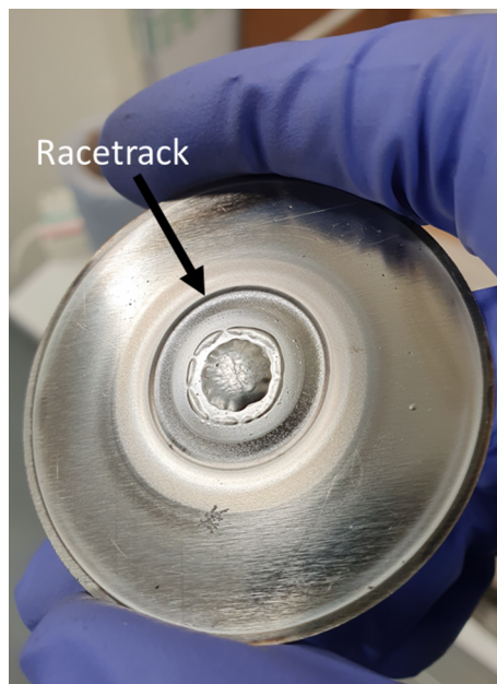
Figure 4.3: A used iron target with the racetrack labelled. The racetrack is formed from the sputtering of the material during NP production. A large amount of the target is not sputtered, i.e. wasted, during this process.
