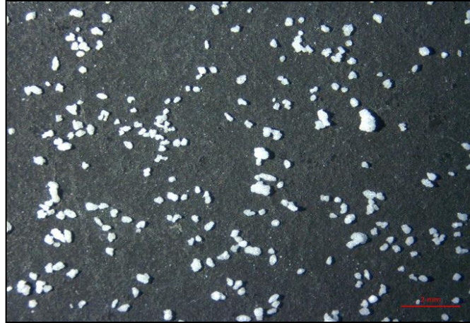
Figure A3. Unweathered HDPE particles under microscope. Particles were scattered on a slide, flattened by over-laying a piece of glass and images captured with a Zeiss PlanNeoFluar Microscope at 33.5 magnification. Microplastic particles which were treated (four hours per day over a period of five months) with UV radiation having 365 nm wavelength looks like the unweathered HDPE particles.
