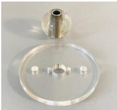
Figure 1.2. Commercial PDMS ball and disc used for tribology measurements.
