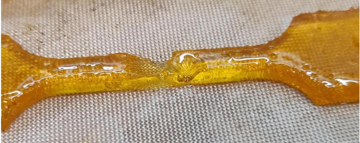
*Figure 31: Air bubbles in rapidly cured SFFT samples.*
