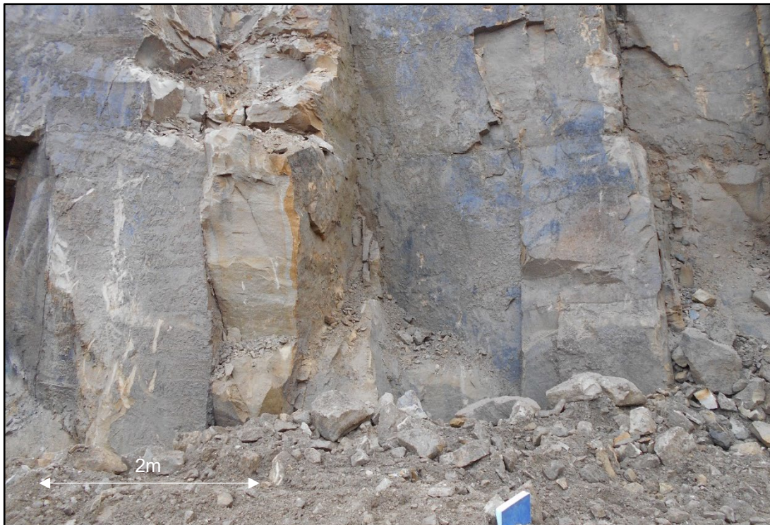
Figure C7: Orthogonal jointing in massive bedded sandstone of the Tyne Limestone Formation, Blaxter Quarry, Northumberland
