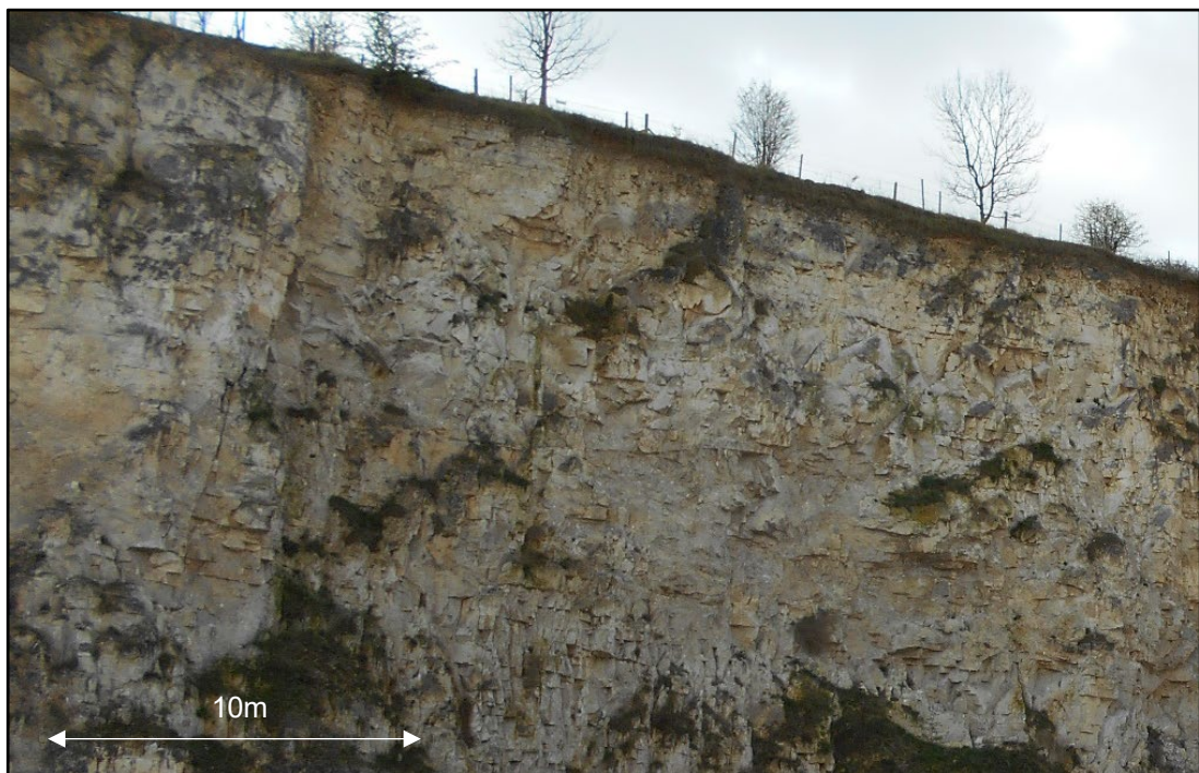
Figure C2: Heterogeneous jointing in a Magnesian Limestone quarry face at Newthorpe Quarry, Sherburn in Elmet, North Yorkshire.
