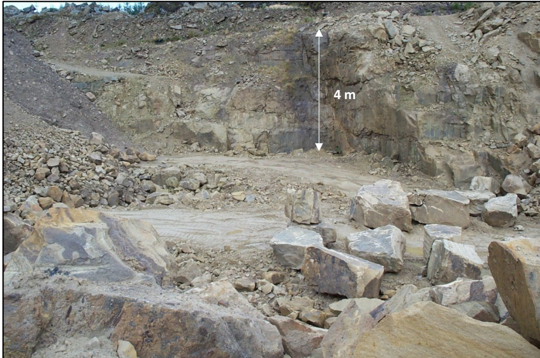
Figure 3.1: Exposed rock faces at Blaxter Quarry showing bedding planes and orthogonal jointing. Rock is extracted at the quarry by hydraulic excavator without requirement for blasting.
