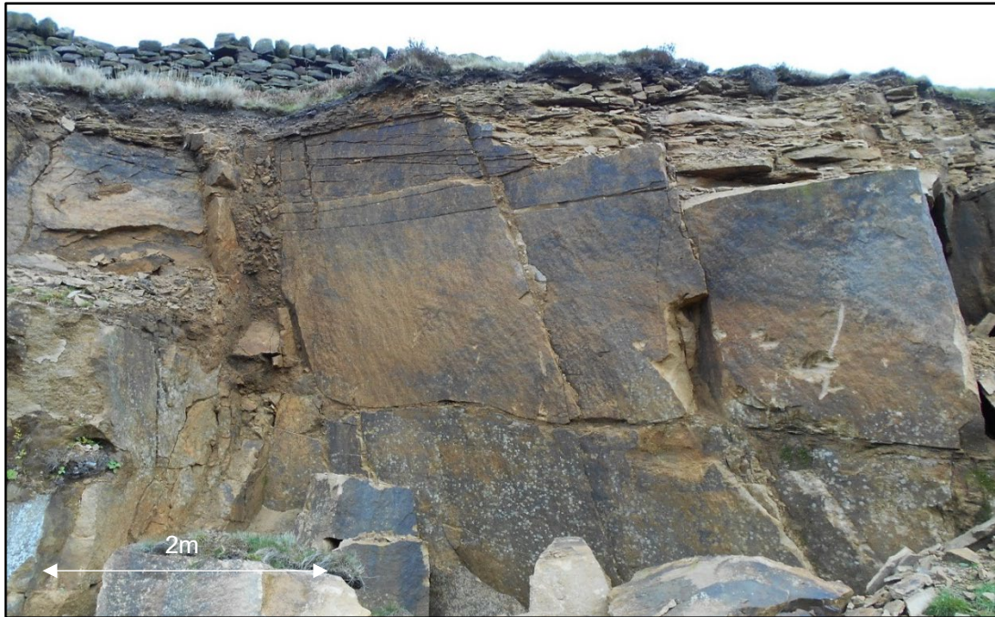
Figure C6: Orthogonal jointing in massive bedded Guiseley Grit sandstone at New Stones Quarry, Hebden Bridge, West Yorkshire, UK
