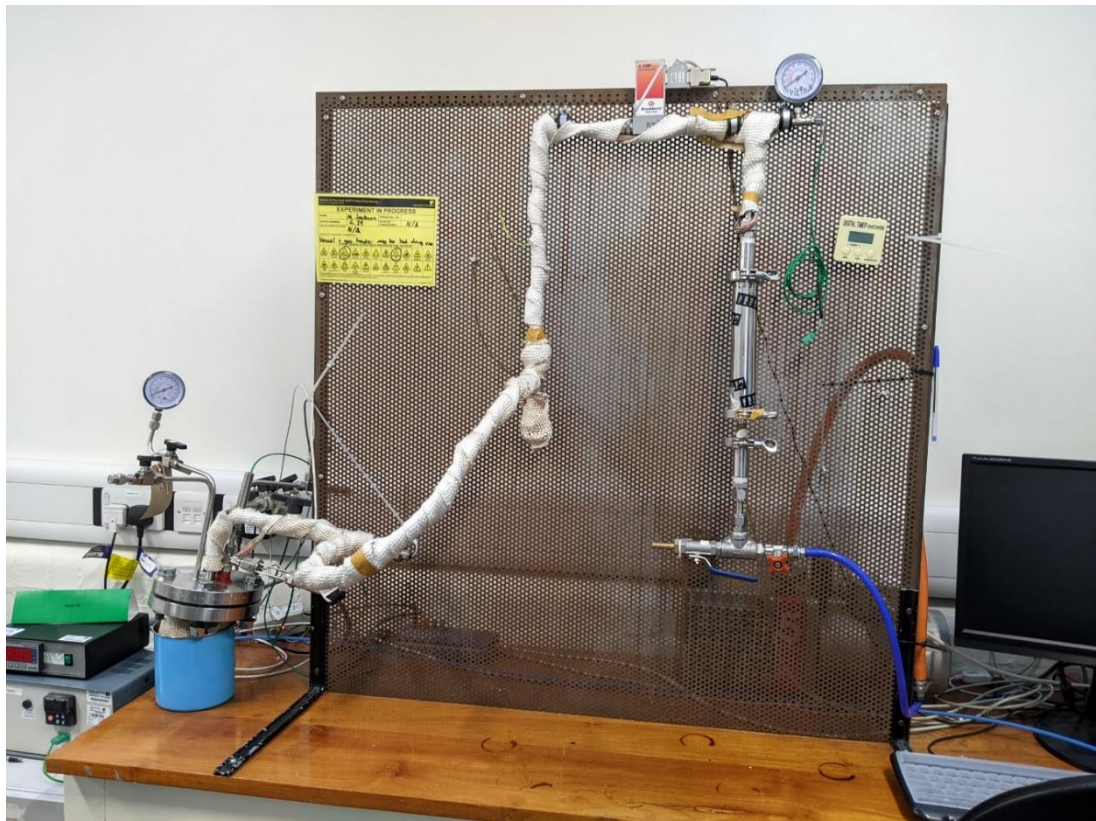
Figure 3-5. Image of drying rig following addition of rope heater (beneath lagging) and removal of unnecessary parts
