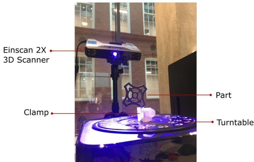
Fig. 7.2 Einscan 3D scanner set-up
