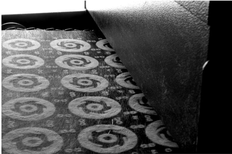
Fig. 2.16 Deposition of polymer powder in CBAM process [99]
