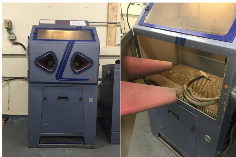
Fig. 3.15 Guyson Euroblast 4 sand blasting machine
