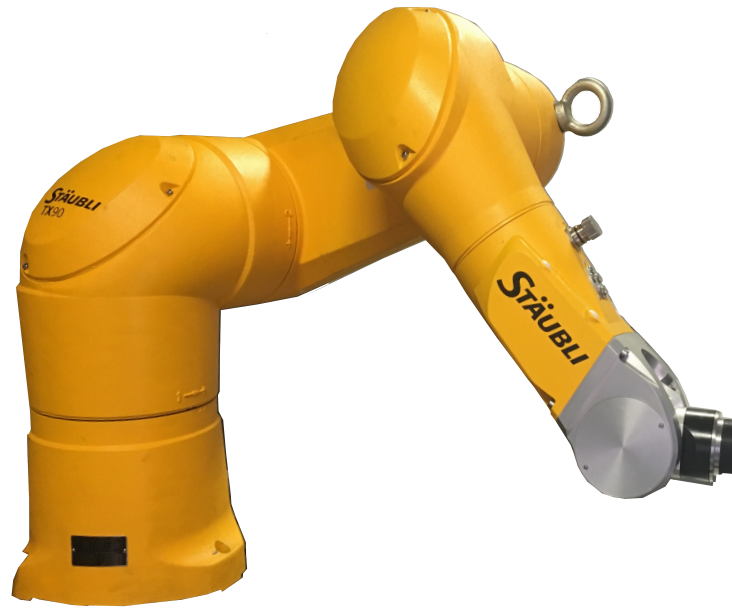
Fig. 4.6 STAUBLI TX-90 industrial robot
