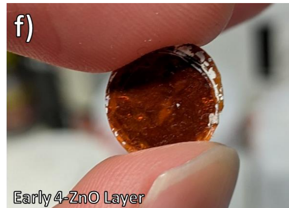
Figure 5.9: Images showing 1-, 2-, and 4-layer samples cold sintered at 200°C 250MPa and the transparency of the deposited ZnO layer. a&b) First successful transparent single layer sample. c) Single layer sample, with the top layer removed revealing a translucent sheet of ZnO on the Kapton. d) Single layer separated illustrating strong to the Kapton® which results in tearing before peeling. e-f) Early 2-, and 4-layer samples in which the transparency decreased with increasing number of layers
