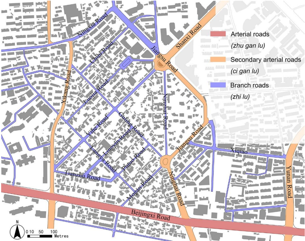
Figure 5.8 Three types of streets based on traffic hierarchy in Yihe Road community.
