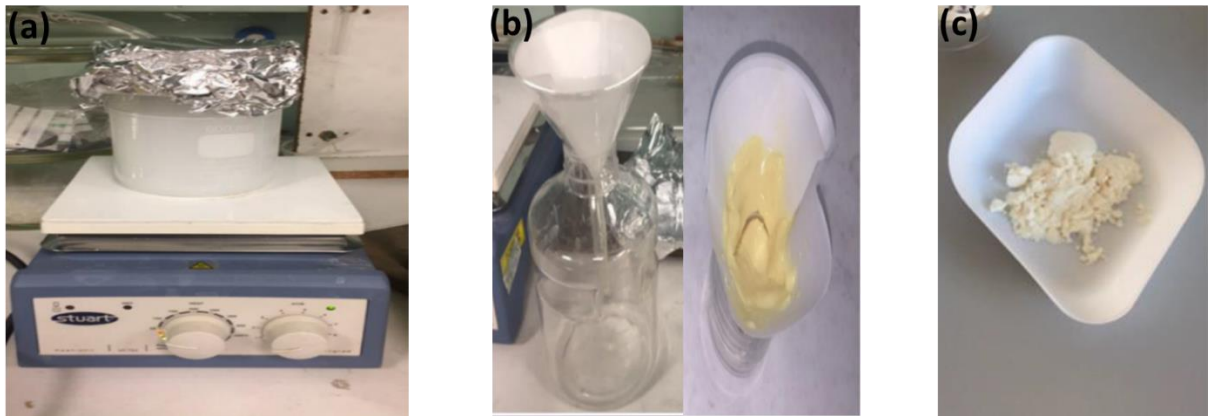
Figure 3.2: Experimental steps of preparing 10% mole \text{Fe}^{3+} doped brushite (DCPD-Fe) powder; (a): stirring process, (b): filtration process and (c): resultant powder after drying process.
