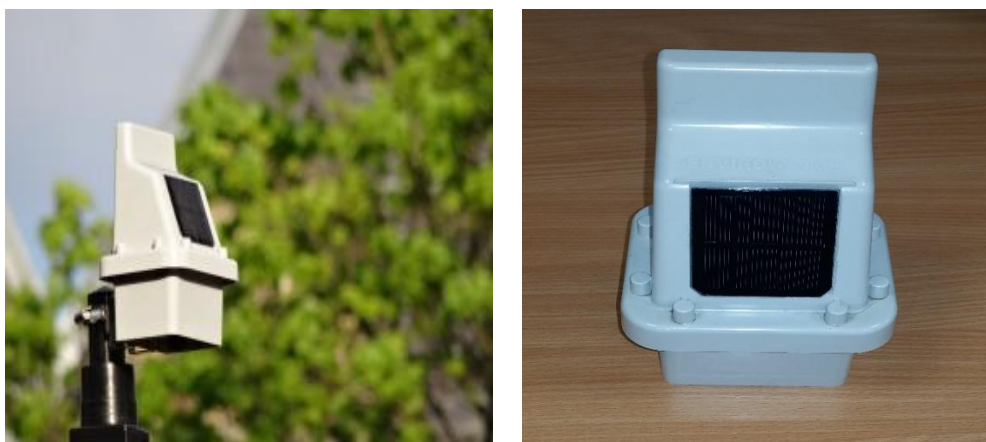
Fig. 3.1: Envirowatch E-MOTEs post-mounted (left) and showing the solar panel used for battery charging (right). Ten of these E-MOTEs were used for collecting data used in this study.
