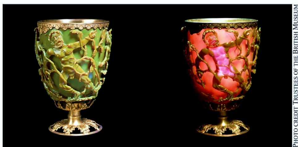
Figure 1.1.2 The Lycurgus cup is made of dichroic glass and presents differently coloured in front-lit (green) and back-lit (red) due to differences in the type of reflected and transmitted light caused by the Au-Ag alloy NPs in the glass. 12 (Copied from the ACS
