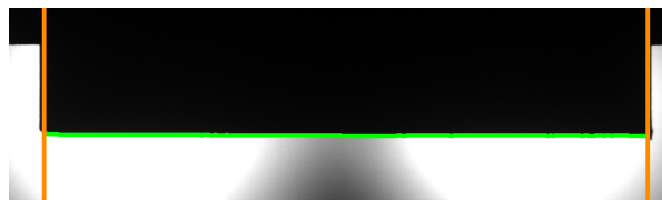
Fig. 4.14 The final blade profile in green overlaid on the cropped image with defined vertical limits shown in orange.
