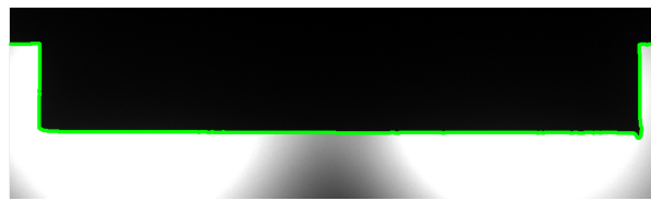
Fig. 4.12 The detected blade and disk edge using the “log” method overlaid on the cropped image after the small edges were removed.
