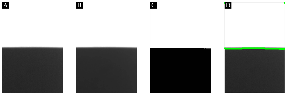
Fig. 4.26 a) The cropped image, b) the median filtered image, c) the binarised image, d) the edge detected using the “Prewitt” method overlaid on the cropped image.
