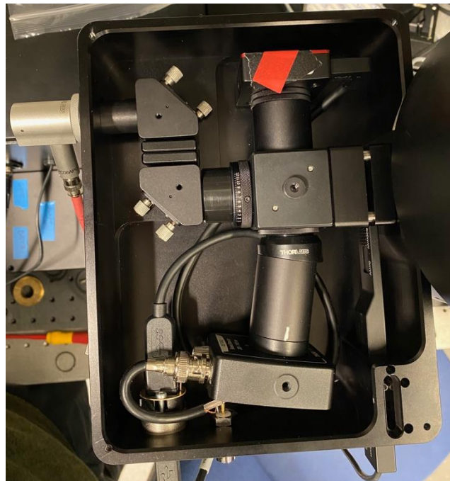
Figure 2.9. A photograph of the excitation module for the openFrame with all the optical components aligned inside the module.
