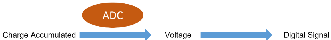
Figure 4.1. A general schematic of how digital values are obtained in detectors, including the factors; quantum efficiency, gain, dark noise and quantization noise.
