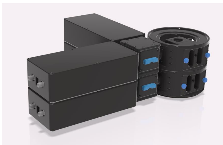
Figure 2.15. A diagram of the final two emission modules for the openFrame. This configuration can be used for polarisation studies.
