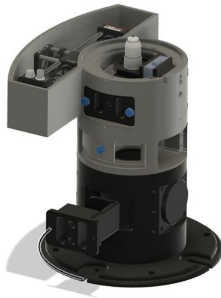
Figure 2.7. The openFrame by Cairn Research with an early draft excitation module on the top layer. The excitation module was designed to input and easily align laser light into the microscope.
