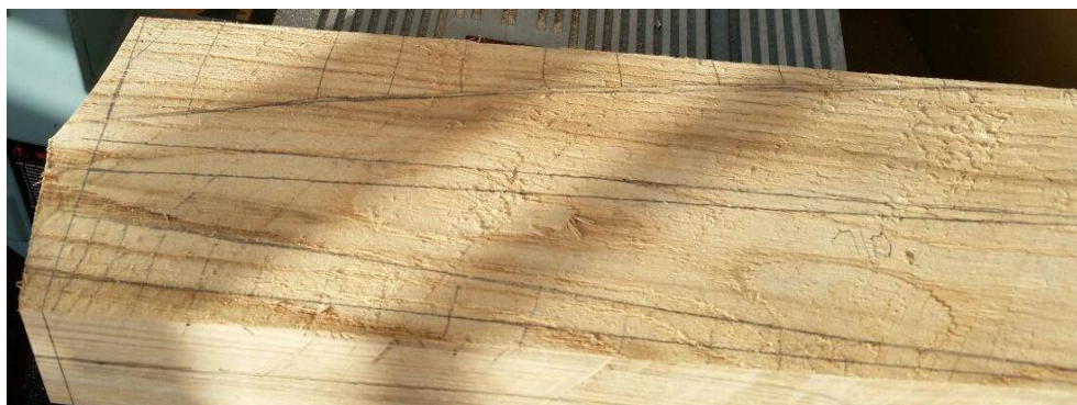
(Fig. 9.9 Rough outline of peg shape with hash lines marking what will be offcuts)
