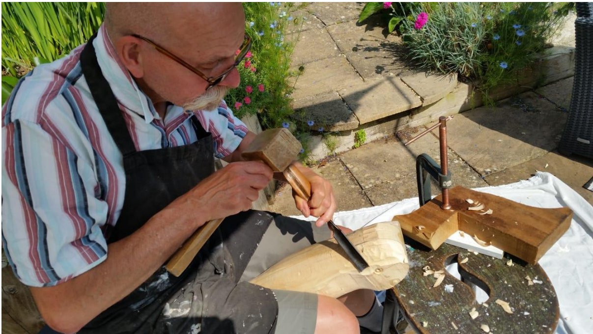
(Fig.10.16 specialist working the wood using a mortise chisel author's image)
