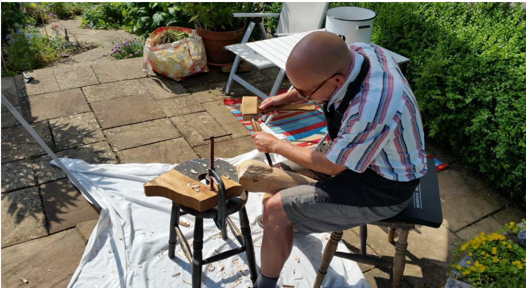
(Fig. 10.18 specialist working with a mortise chisel to create a kneecap)
