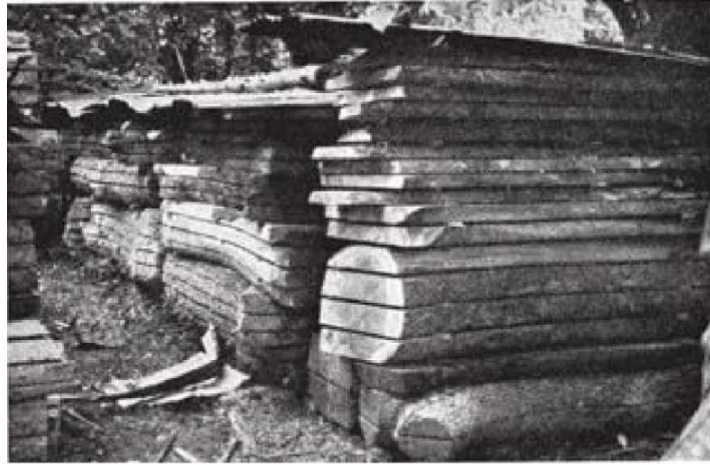
(Fig.. 4.5, Walter Rose's memoirs, drying cut timber 1936: 80)
