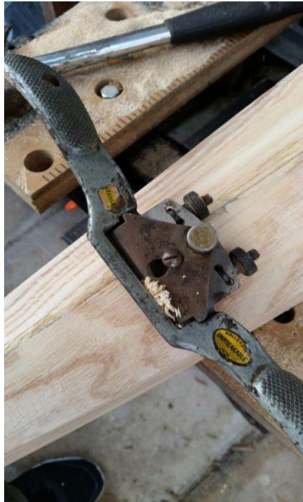
(Fig.9.11, hand plane shaving the excess wood away, author's own )
