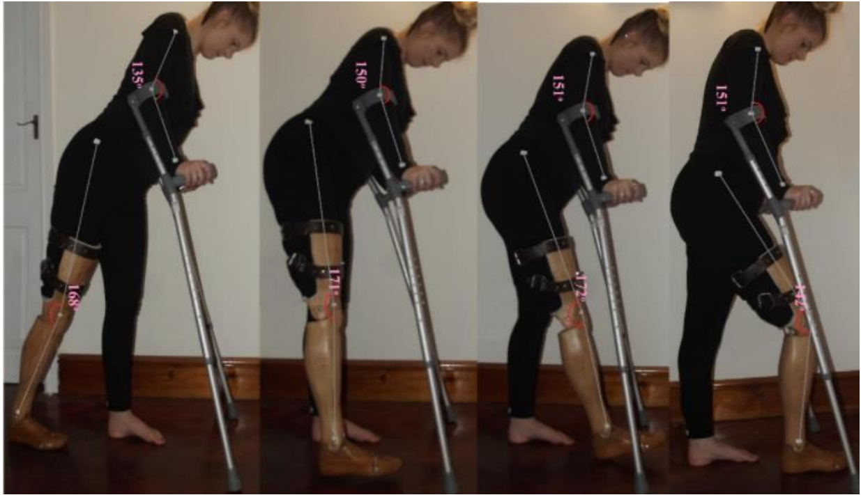
(Fig. 11.10 Lateral view of Anglesey Leg gait cycle)
