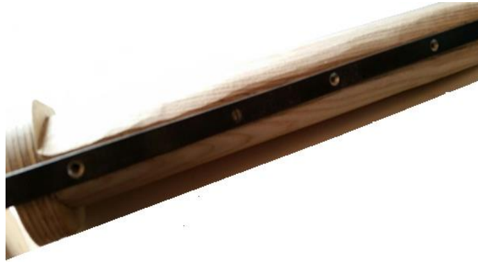
(Fig.9.22 The mild steel metal thigh support attached to the peg component, author's own )
