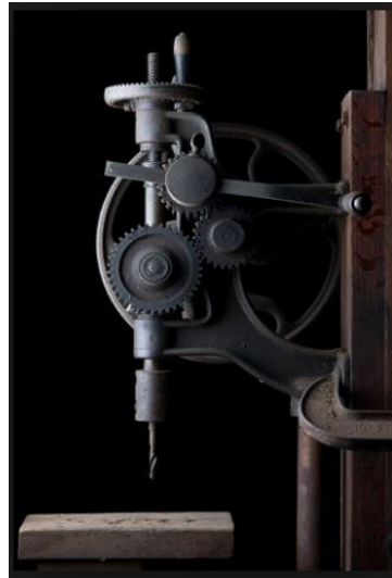
(Fig.. 4.8 nineteenth-century drill press, turned by hand to drill hole)
