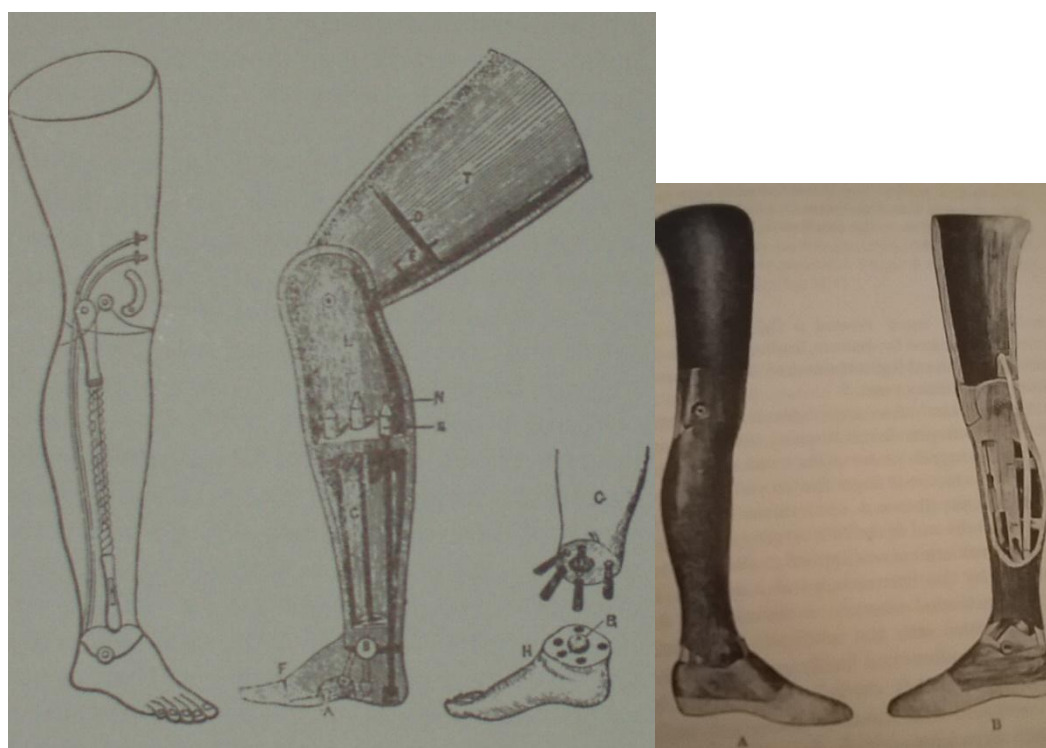
(Fig. 10.13 internal construction of Anglesey legs including springs, cords and joints, from Mihm et al 2002: 285)
