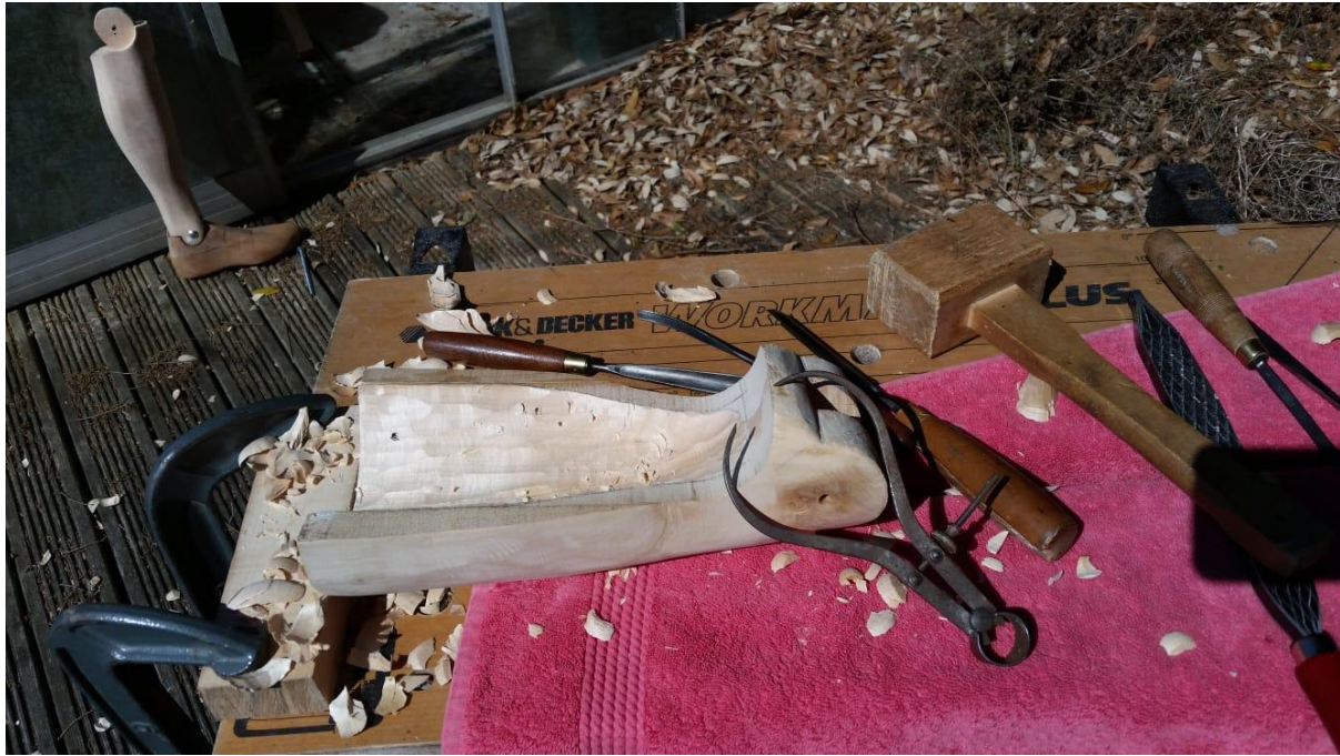
(Fig. 10.29 finished shape of the calf section's socket, author's own)
