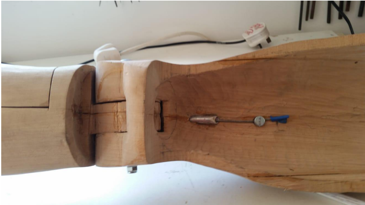
(Fig. 10.32 cap screw securing the cable to the inside of the socket, author's image)
