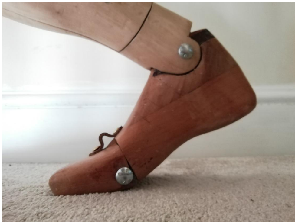
(Fig.10.40 toe off phase of gait cycle showing the bent ankle and toe section author's image)
