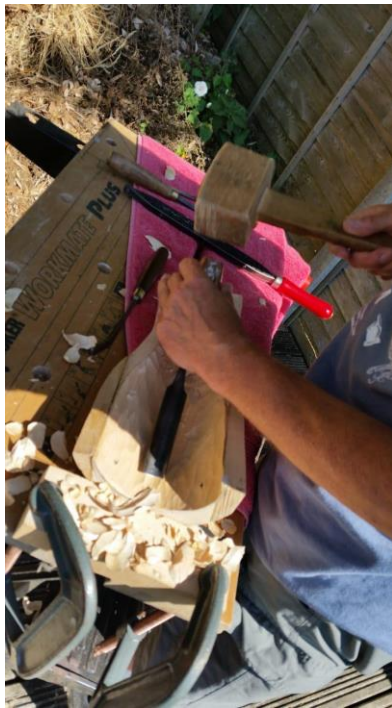
(Fig.10.28 showing the mortise chisel being used to hollow out the socket area to an appropriate thickness)
