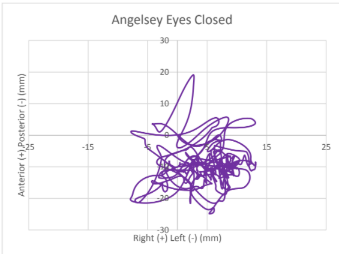
(Fig. 6.1 Force plate generated balance results for Anglesey leg, eyes open and eyes closed for 30 seconds each). (-5, -15, -25) represents more pressure being placed on the left side of the body compared to (+5, +15, +25) which represents more pressure on the right side of the body. Anterior (+) and Posterior (-) represent how far the body is leaning forwards or backwards.)
