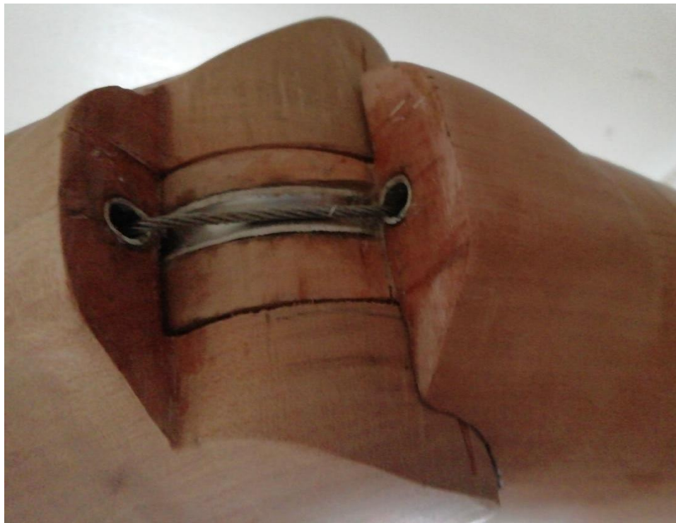
(Fig. 10.34 half-round metal channel and wire positioned through the knee joint, author's own)
