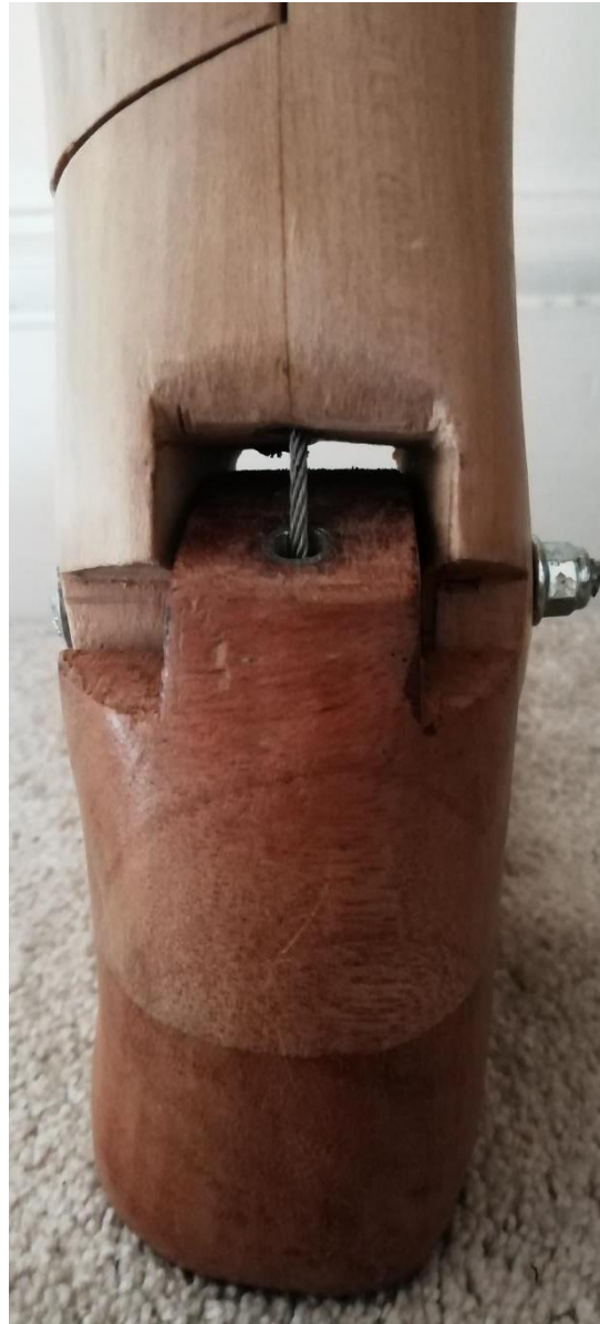
(Fig. 10.37 wire cable passing through the ankle joint into the calf joint visible during mid gait cycle bending of the ankle, author's own)
