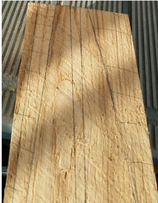
(Fig. 9.8 Rough outline of peg shape with hash lines marking what will be offcuts)
