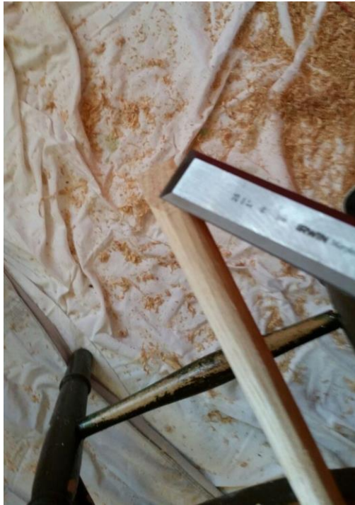
(Fig.9.15 trimming the tip of the lateral stabiliser with a chisel so it smoothly attaches to the leg component, author's own)
