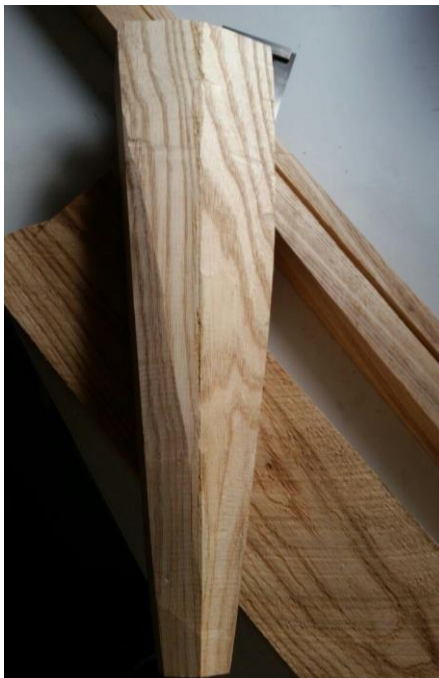
(Fig. 9.12 rudimentary shape of the peg component before edges have been smoothed, author's own )
