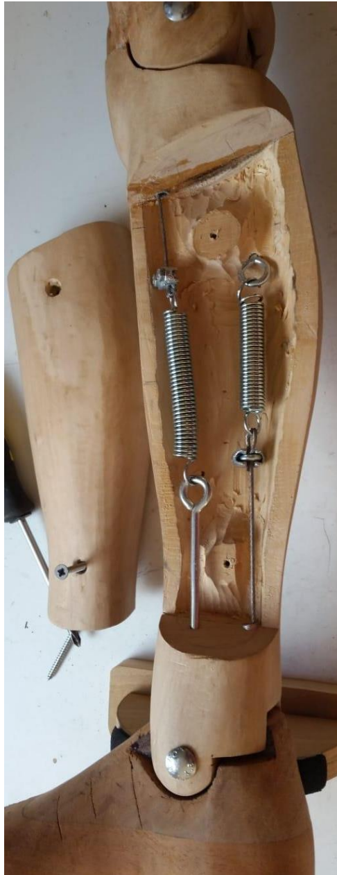
(Fig. 10.36 top left corner of calf section showing exit area of the wire and also spring positioning, author's image)
