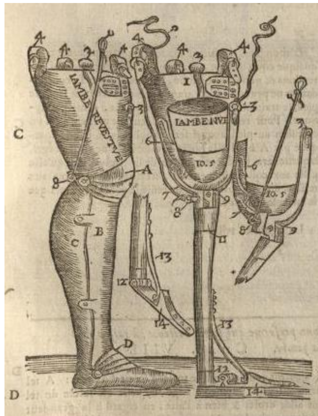
(Fig. 2.7 Paré's knee locking artificial leg, image courtesy of Herginou, 2013)
