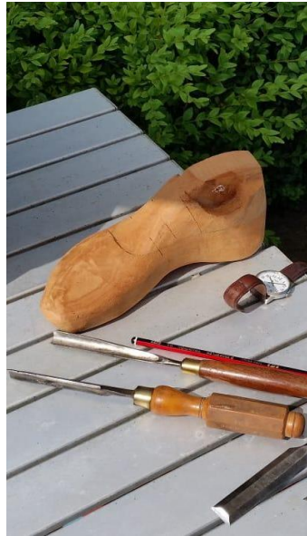
(Fig. 10.11 smooth and sanded foot shape ready for attachment to the calf section of the limb, author's own)
