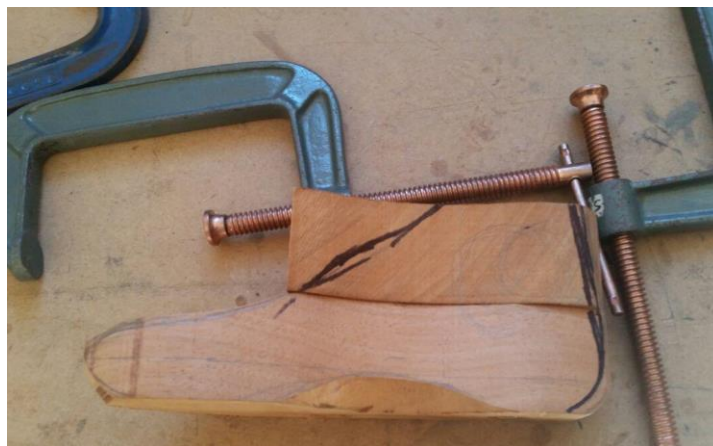
(Fig. 10.6 two blocks of wood secured with hide glue to make the beginnings of the foot piece that would attach to the ankle joint and calf section, author's own)
