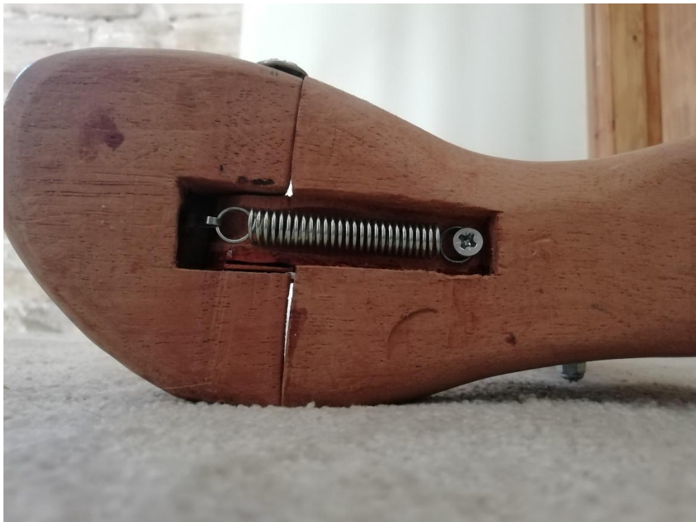
(Fig.10.38 spring element connecting toe section and heel section of the foot at base author's image)
