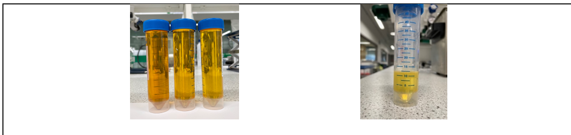
Figure 6.15 (Left). MHC produced in different temperatures 90, 60 and 40 °C and (right). MHC 40 °C after purification
