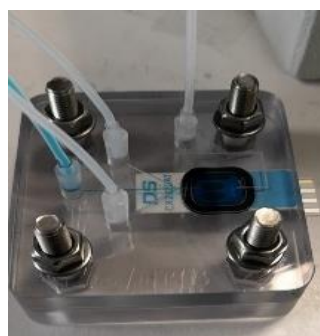
Figure 2.6: Photograph of microfluidic Chip 1 and design and photographs of microfluidic Chip 2. A , the chip was designed and fabricated as described in (Patinglag et al., 2020). B , the chip was made of PC fabricated using CNC machine milling. The sample chamber (7.5 mm wide, 9 mm long, and 0.2 mm depth) is connected with the inlet channels (7.5 mm wide, 22.5 mm long, 0.2 mm depth). An O-ring made of nitrile rubber with a 10.1 mm bore and 13.3 mm outer was employed. PTFE Teflon tubing (1.58mm od x 0.5mm id) were inserted into inlets and outlet through a 2.5 mL syringe luer adaptor and glued with Araldite.
