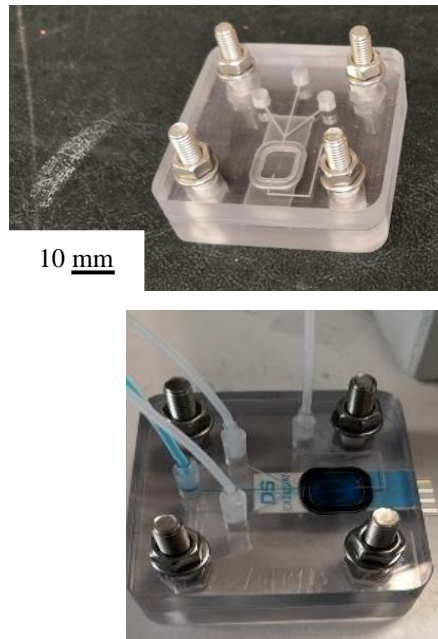
Figure 7.5: Replicate of Figure 2.6 for clarity. A , the chip was designed and fabricated as described in (Patinglag et al., 2020). B , the chip was made of PC fabricated using CNC machine milling. The sample chamber (7.5 mm wide, 9 mm long, and 0.2 mm depth) is connected with the inlet channels (7.5 mm wide, 22.5 mm long, 0.2 mm depth). An O-ring made of nitrile rubber with a 10.1 mm bore and 13.3 mm outer was employed. PTFE Teflon tubing (1.58mm od x 0.5mm id) were inserted into inlets and outlet through a 2.5 mL syringe luer adaptor and glued with Araldite.
