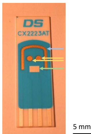
Figure 1.7: Metrohm DropSens CX2223AT screen-printed gold electrode. The chip contains two circular gold working electrodes, a gold counter electrode and a rectangular Ag/AgCl reference electrode, which are screen-printed onto a ceramic base. The blue material insulating the electrodes corresponds to the dielectric, preventing cross-connections. Four silver connectors at the bottom of the chip connect the chip to the potentiostat. Working (—blue—), counter (—yellow—) and reference electrode (—green—).
