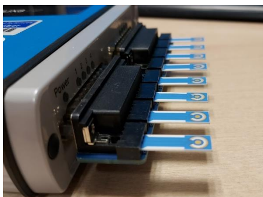
Figure 2.3: Palmsens workstation setup. A , Palmsens4 potentiostat, galvanostat and frequency response analyser (FRA) coupled to a multiplexer (MUX8-R2) with adaptors connected to 8 different Electrodes 3. The potentiostat was controlled through PStTrace 5.8 software. B , a closer image corresponding to the adapter and the set of 8 SPGEs.
