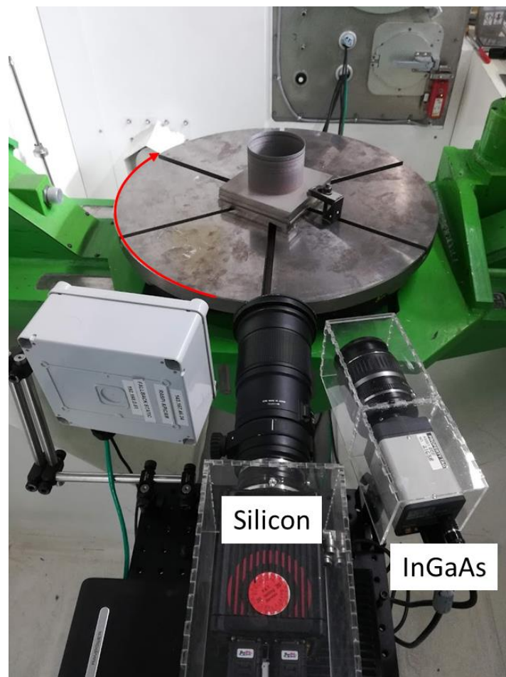
Figure 7-3: Setup of cylinder build; showing table rotation and camera setup
