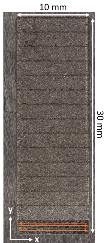
Figure 6-7: Example of a staircase printed with powder, hatching in the x direction as shown by orange arrows
