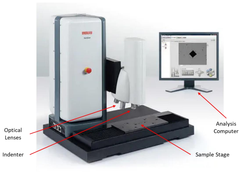
Figure 4-12: Durascan 70 Vickers hardness indenter, labelled, showing its' main components; adapted from [172]
