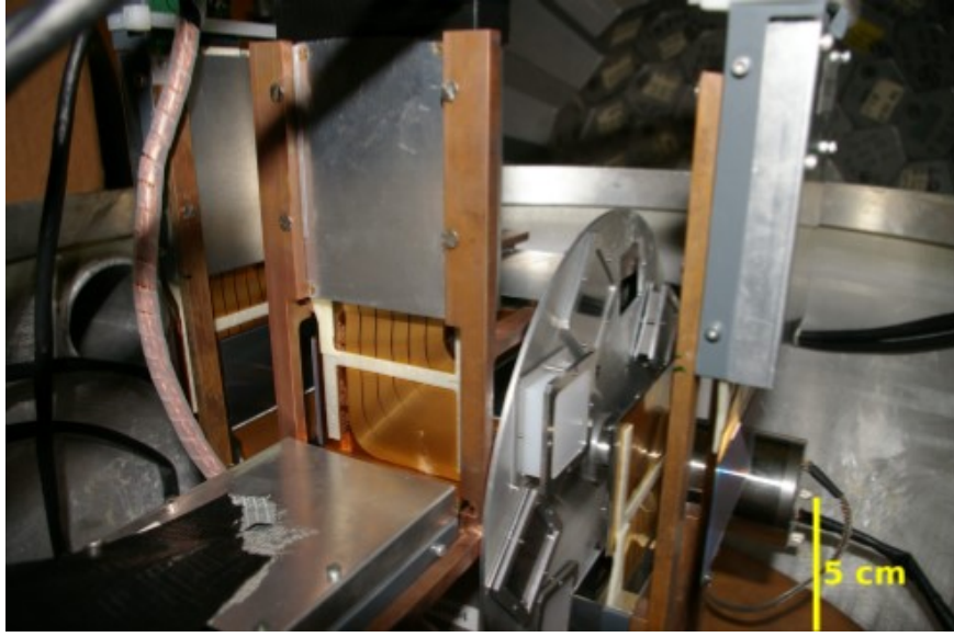
Figure 21: A picture of the vacuum reaction chamber surrounds the target wheel and the Silicon Strip Detectors (SSDs) [23].
