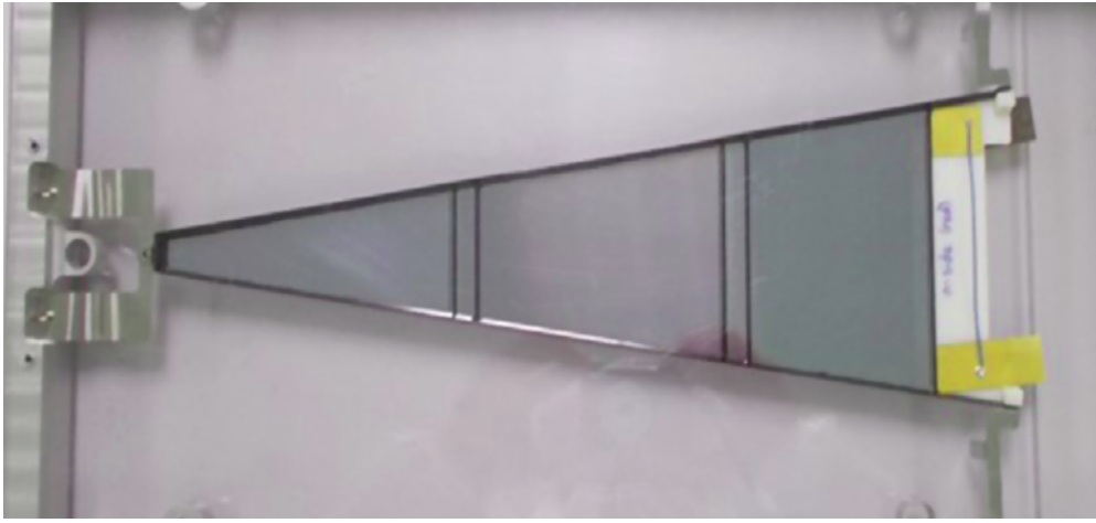
(b) The Si-assembly of the outer detector.
