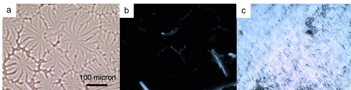
Figure 4.2. Optical microscope images of B1 sandwiched between two glass slides: a) observed without polarizer; b) with cross polarizers; c) the two glass slides were sheared with respect to each other.
