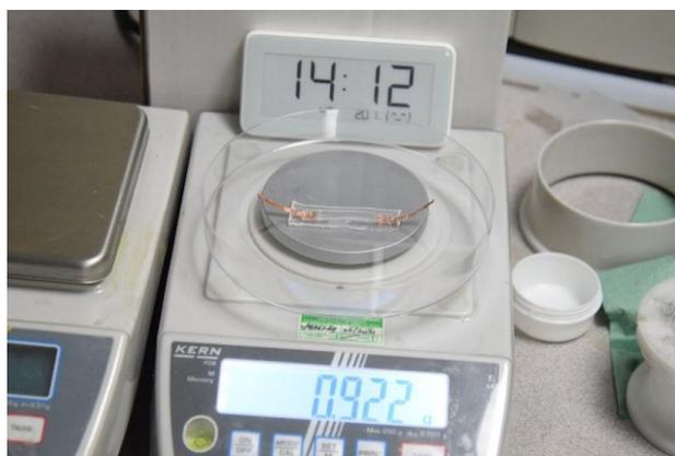
Figure 5-3 Water retention test setup for hydrogel samples. The hydrogel sample encapsulated by PDMS was exposed to the air for 24h at room temperature.
