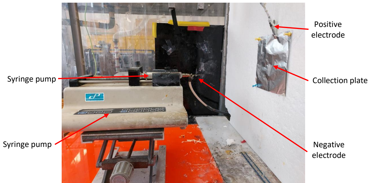
Figure 3.1 Image of electrospinning setup used for the production of nanofibre samples used in composites.
