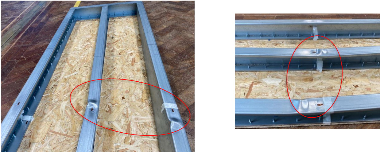
Figure 5.35 Failure modes of DR2 specimen
