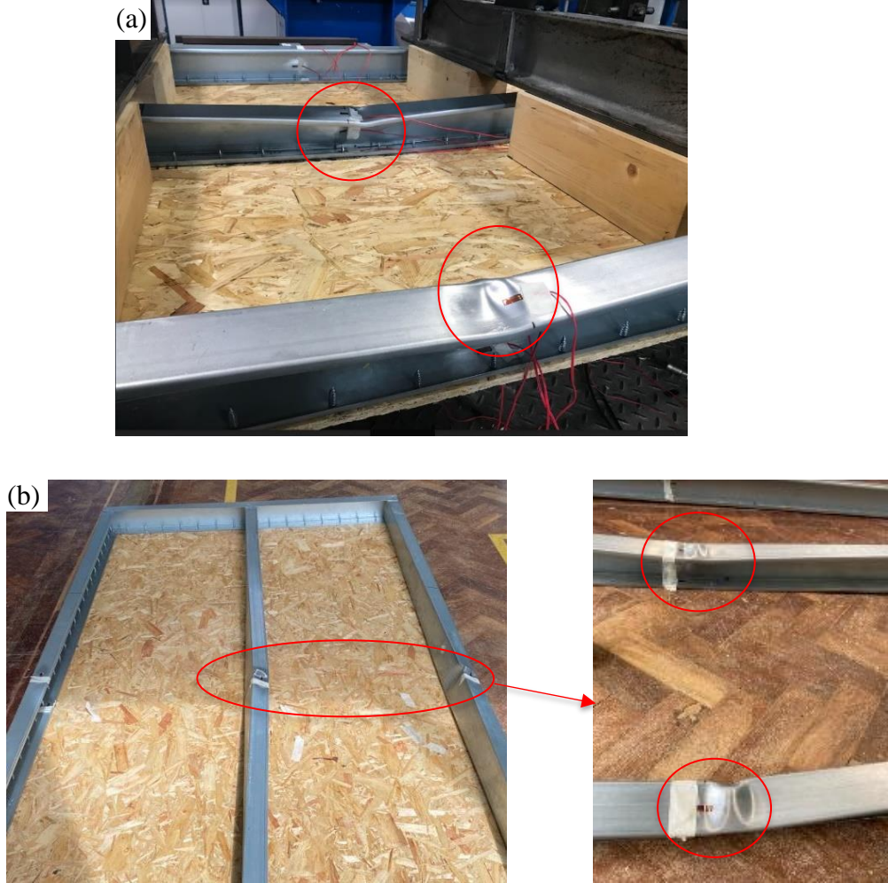
Figure 5.25 Failure modes of: (a) K3 and (b) K5 specimens
