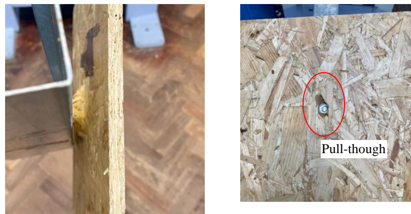
Figure 6.8 Typical failure mode captured from the pull-out tests
