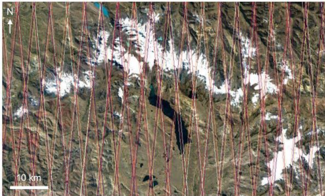
Figure 4.9 – Ground track positions of ICESat-2 over the Cordillera Vilcanota over a 2-year time period. The eight positions are demonstrated in different shading.
