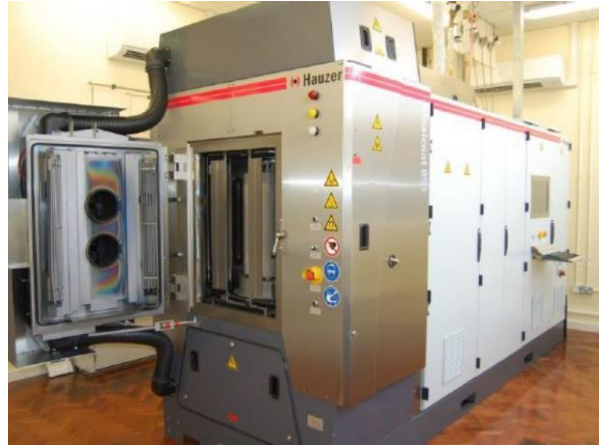
Figure 4.1 The Hauzer Flexicoat 850 PVD machine.
