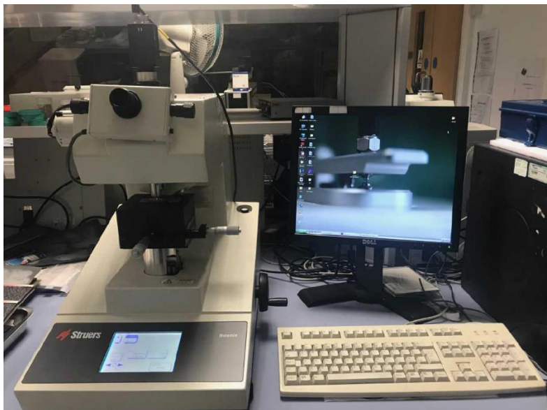
Figure 14 computer-aided Duramin Indenter Machine
