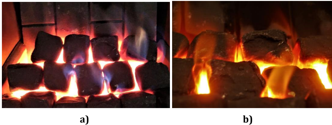
Figure 7-3: Open fronted fire FPB2 10 mbar: a) NG; b) H 2
