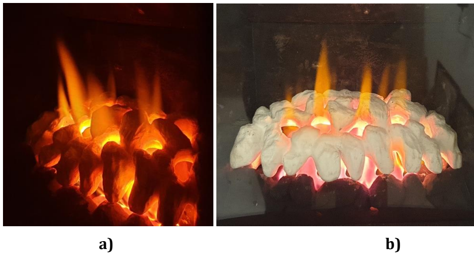
Figure 7-23: Glass fronted fire LB17 H 2 full power (3.4kW): a) lights off, b) lights on
