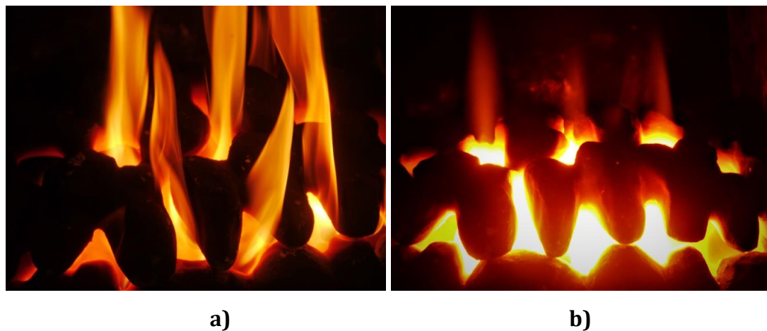
Figure 7-13: LB2 15mbar . a) Natural gas; b) Hydrogen
