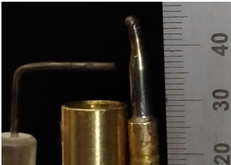
Figure 3-28. Prototype pilot used for the fires in the Hy4Heat project
