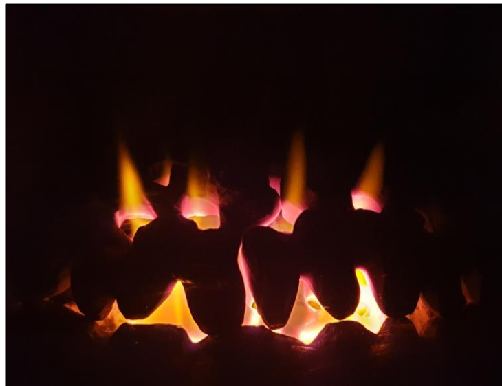
Figure 7-24: Glass fronted fire LB17 H 2 half power (3.4kW)
