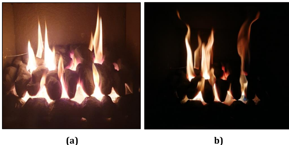
Figure 7-22: LB17-FRONT-ALLC-D-NG; a) 10 mbar, b) 20 mbar
