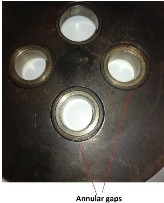
Figure 3-10. Flame stabiliser GM2 featuring an annular injection
