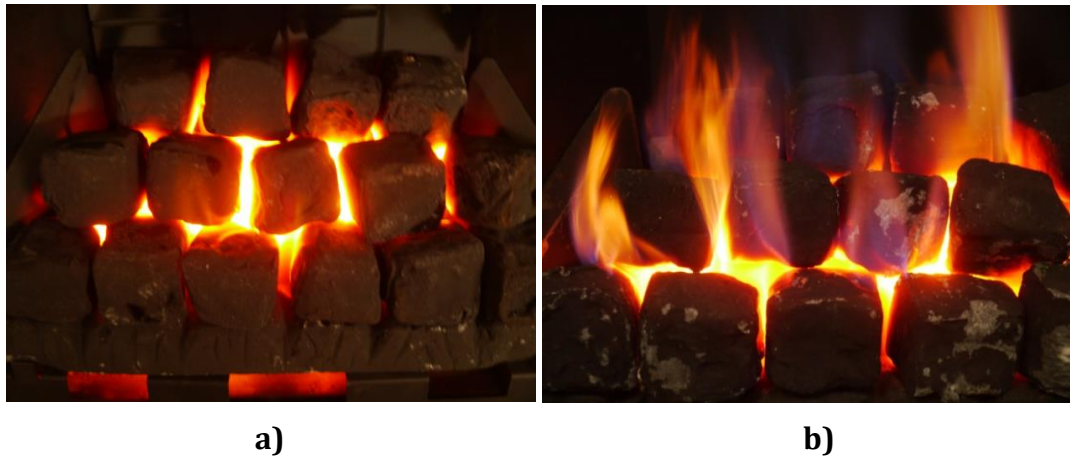
Figure 7-4: Open fronted fire FPB3 13.6 mbar: a) NG; b) H 2
