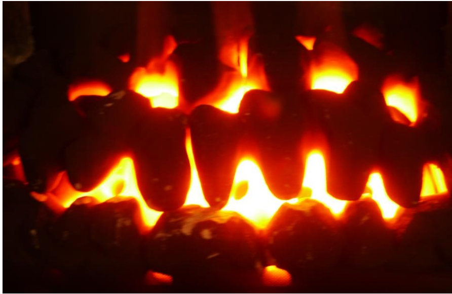
Figure 7-15: Glass fronted fire LB5 all coals H 2 3mbar
