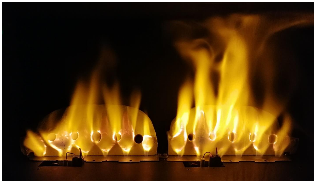
Figure 7-33: Flame for Innovative fire using LB4 (LHS) and LB5 (RH) 15 mbar, H 2
