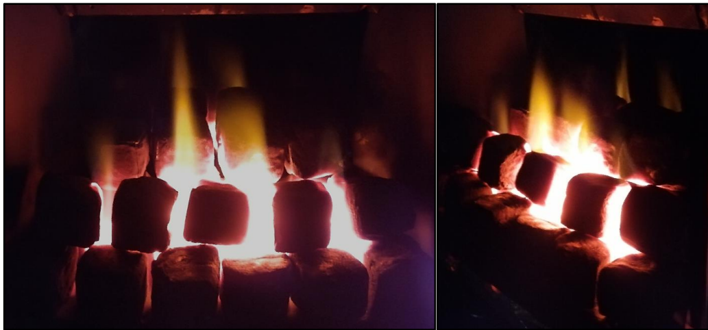
Figure 7-6: Open fronted fire FPB3 for dual fuel H 2 20 mbar.
