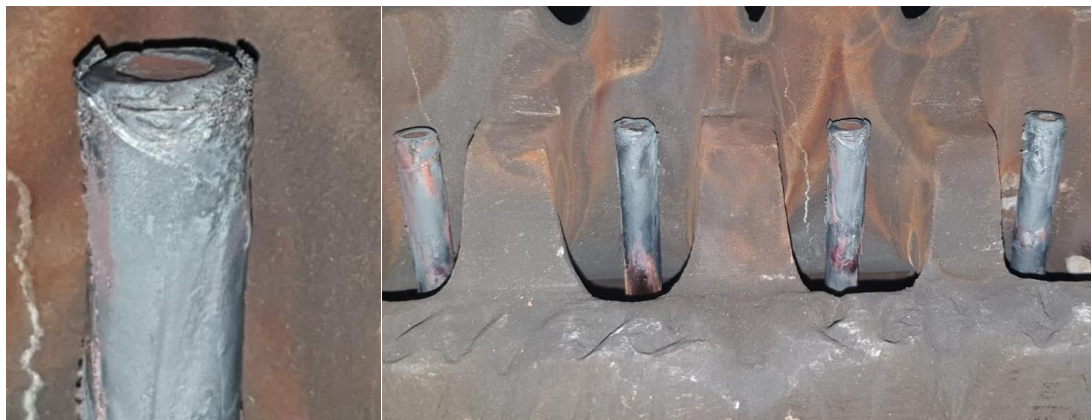
Figure 7-11: Secondary injection showing cracks and notoriously worn.
