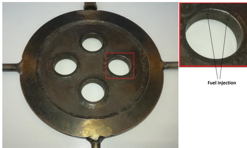
Figure 3-11. Flame stabiliser GM1 featuring eight radial inward fuel nozzles per air hole
