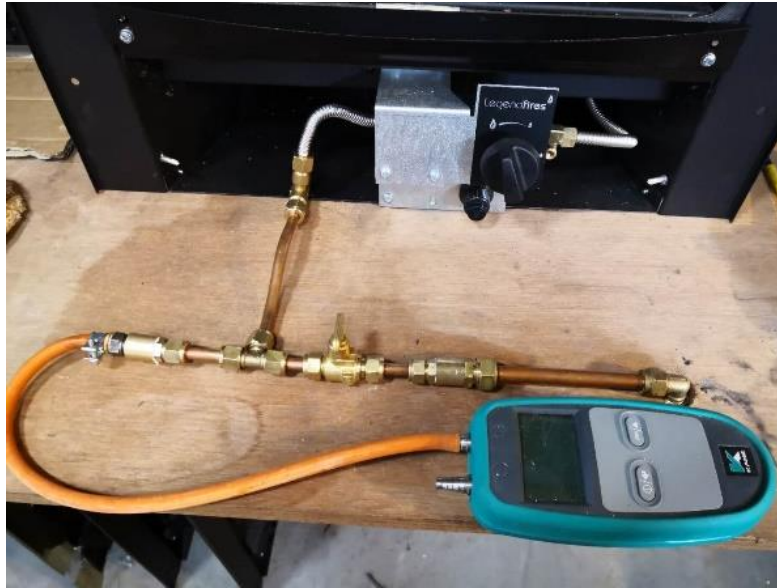
Figure 3-34: Manometer for plenum pressure in the glass-fronted fire.
