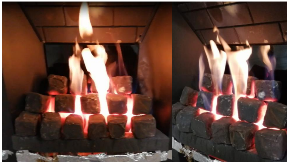
Figure 7-9: Open fronted fire FPB3 for dual fuel NG 20 mbar.
