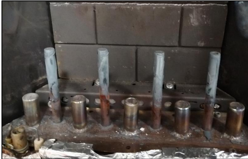
Figure 3-30: Burner design for open-fronted fire two-stage injection
