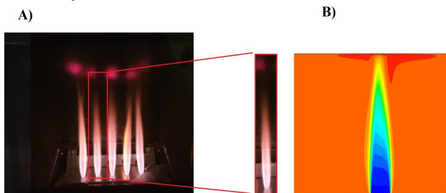
Figure 7-32. Flame shape comparison for NG. A) Experiment; B) Simulation
