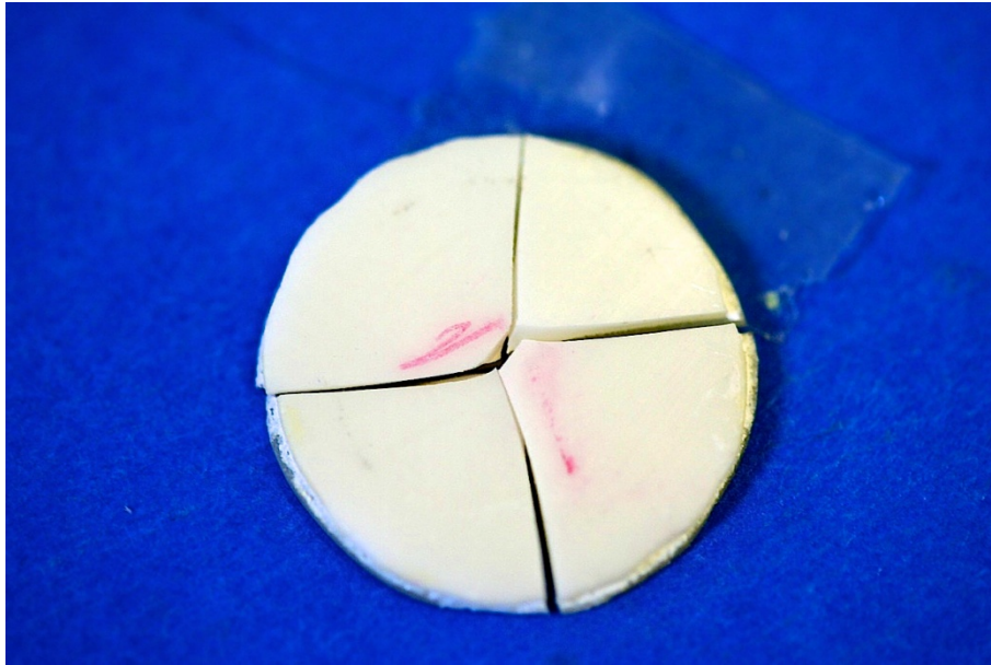
Figure 27: Zirconia/composite (YZ/LC) broken specimen. The bond was established by shot blasting and using universal primer, and as seen that both layers are still bonded after applying the occlusal load.
