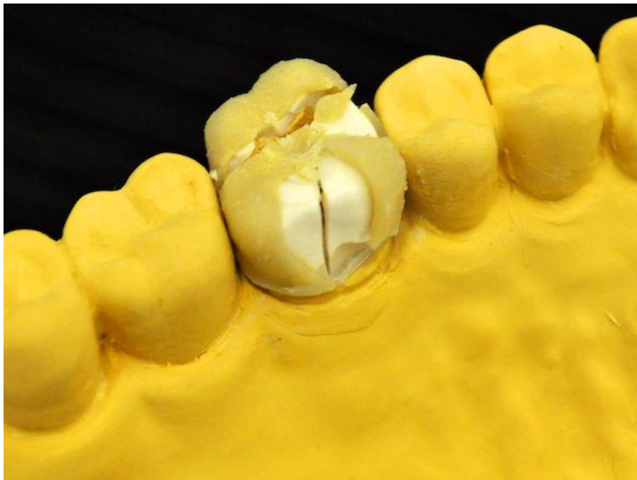
Figure 42: Fractured crown with major delamination between composite veneer and zirconia coping.
