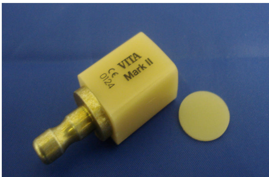
Figure 16: VITA Mark II cerc block and sample disc.
