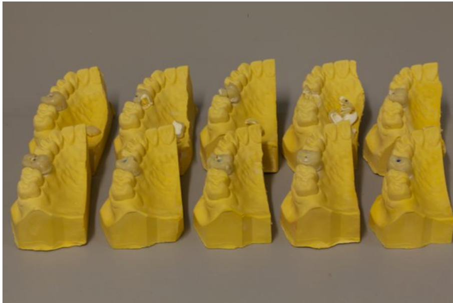
Figure 39: Tested crowns of group 2 with 0.7mm thick zirconia coping
