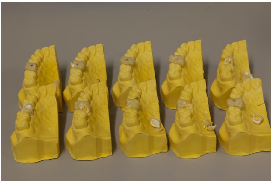
Figure 38: Tested crowns of group 1 with 1.0mm thick zirconia coping.
