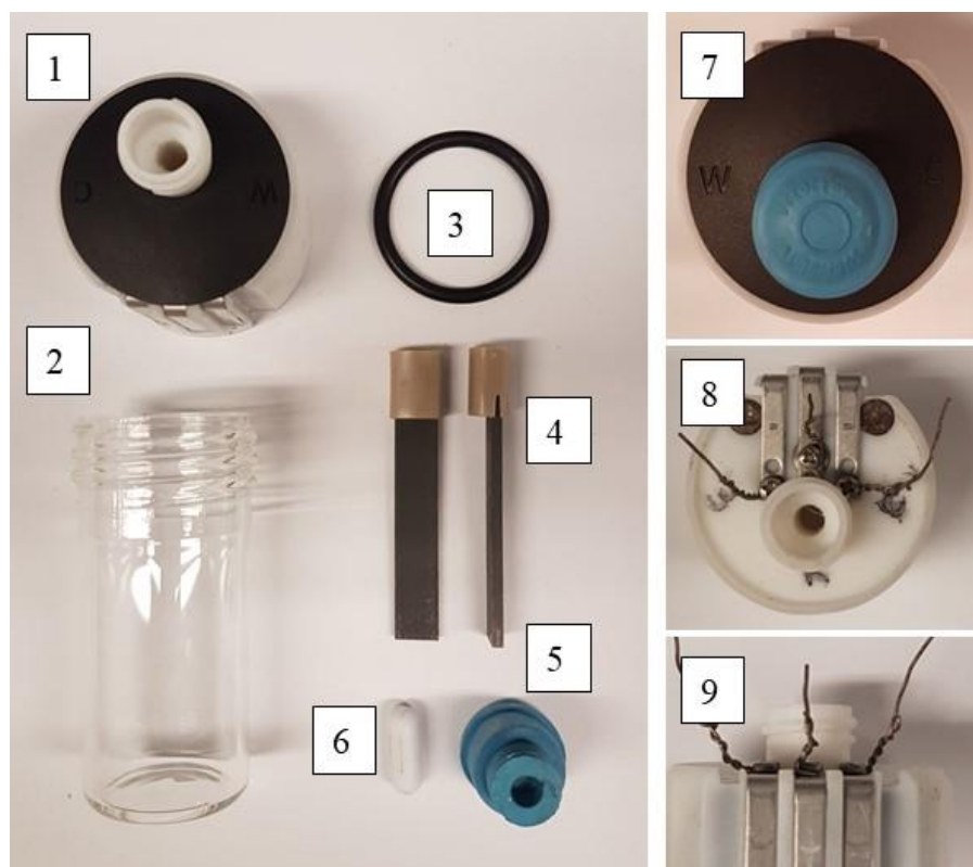
Figure 5.4: 1. ElectraSyn vial lid, 2. 20 mL ElectraSyn Vial, 3. 27 mm internal diameter O ring, 4. ElectraSyn SK-50 graphite electrodes, 5. 17 suba seal, 6. ElectraSyn stirrer bar, 7. Suba seal fitted in ElectraSyn vial lid, 8. Modified ElectraSyn vial lid (top view), 9. Modified ElectraSyn vial lid (side view).
