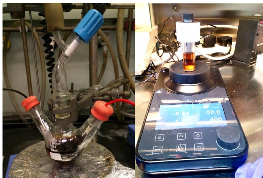
Figure 2.1: Electrochemistry under inert conditions in a three necked flask connected to a Schlenk line (left) and the IKA ElectraSyn 2 (right).
