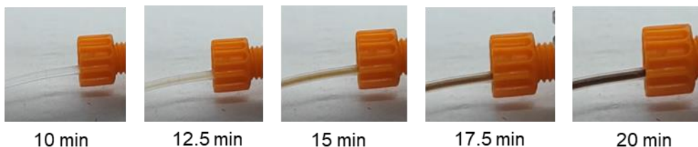
Graph 4.5: Colour analysis of the continuous electrochemical synthesis of Ni11 : 6 mM, 1 mA, 1/60 Hz, 0.04 mL min -1 . Orange line from calibration corresponds to 20% yield. 1 H NMR analysis showed a yield of 19%.
