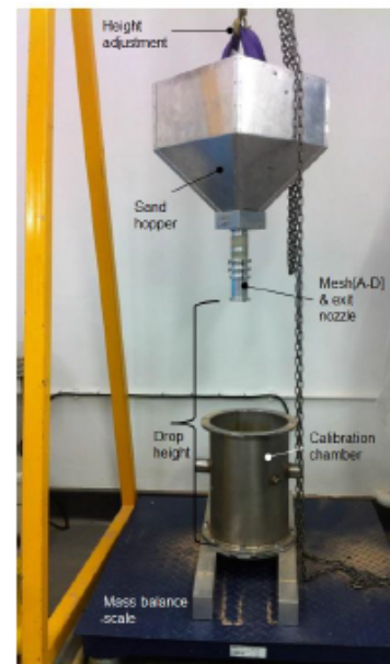
Figure 3. Sand pluviation configuration.
