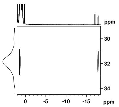
**Figure 15.** { $^{1}$ H- $^{29}$ Si} 2D NMR spectrum showing correlation between the hydride resonance for the complex Tp`RhH(Et<sub>2</sub>SiH)(PMe<sub>3</sub>) and the  $^{29}$ Si signal. The ethyl protons are also linked to the  $^{29}$ Si resonance. The second hydride belongs to starting material left.
