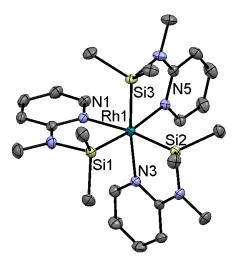
**Figure 15.** Crystal structure for the rhodium-tris-silazane complex; hydrogen atoms are omitted for clarity. Ellipsoids for the anisotropic displacement parameters are shown at the 50% level.
