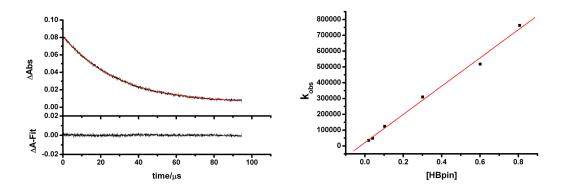
**Figure 13.** Left: transient decay after photolysis of  $Ru(dppe)_2H(Bpin)$  recorded at 470 nm at 298 K. Right: plot of the pseudo first order rate constants,  $k_{obs}$  vs the concentration of HBpin.
