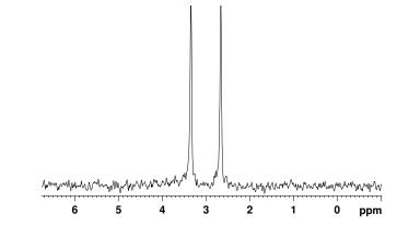
**Figure 2.** <sup>31</sup>P{<sup>1</sup>H} NMR spectrum in  $C_6D_6$  for the Tp`Rh(PMe<sub>3</sub>)H<sub>2</sub> starting material.
