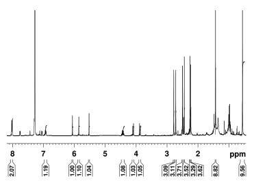
**Figure 18.** <sup>1</sup>H NMR spectrum of complex Tp`Rh(CNneopentyl)( $\eta^2$ -PhN=C=Nneopentyl) in C<sub>6</sub>D<sub>6</sub>. The spectrum shows the presence of some impurities.
