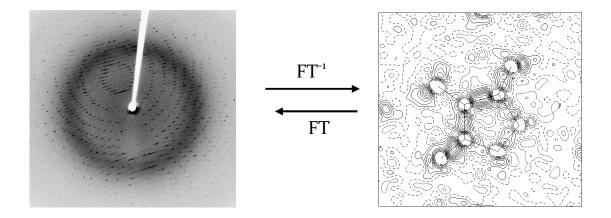
**Scheme 1.** Schematic representation of the use of the Fourier Transform in crystal structure determination. The two pictures are not related to each other.<sup>5</sup>
