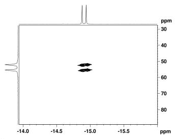
**Figure 14.** {<sup>1</sup>H-<sup>29</sup>Si} 2D NMR spectrum showing correlation between the hydride resonance and the <sup>29</sup>Si signal. The <sup>29</sup>Si signal is two resonances, confirming the presence of two inequivalent <sup>29</sup>Si environments.
