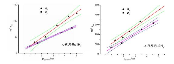
**Figure 7.** Plots of pseudo-first-order rate constants for the decay of the transients obtained upon laser flash photolysis (308 nm) of complexes  $\Lambda$ -*R*,*R*-Ru1H<sub>2</sub> and  $\Lambda$ -*R*,*R*-Ru2H<sub>2</sub> in cyclohexane vs the pressure of quenching gas (H<sub>2</sub> and D<sub>2</sub>). The lines through the points show the best fits and the colored lines show the 95% confidence limits.
