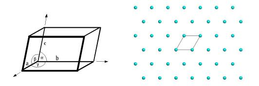
**Figure 1**. (a) Representation of a unit cell where *a,b,c* are the unit cell lengths and  $\alpha$ ,  $\beta$ ,  $\gamma$  the angles.<sup>1</sup> (b) Schematic representation of a crystal lattice where every point is a lattice point.<sup>2</sup>
