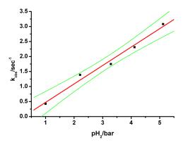
**Figure 12.** Plots of pseudo-first-order rate constants for the decay of the transient obtained upon laser flash photolysis (308 nm) of complexes  $\Lambda$ -*R*,*R*-Ru3H<sub>2</sub> in cyclohexane vs the pressure of hydrogen. The line through the points show the best fits and the colored lines show the 95% confidence limits.
