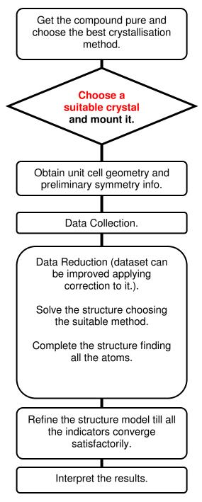
Figure 5. Flowchart for the steps of a crystal structure determination.
