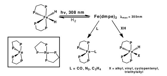
**Scheme 2.** Scheme for reaction of  $Fe(dmpe)_2H_2$  in the presence of different substrates. Inset: different geometries adopted by the Ru and Fe transients.
