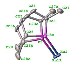
**Figure 3.** Phospholane moiety of complex **3** showing the disorder. Hydrogen atoms are omitted for clarity. Ellipsoids for the anisotropic displacement parameters are shown at the 50% level.
