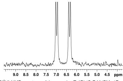
Figure 4.  ${}^{31}P{}^{1}H$  NMR spectrum of the complex Tp`Rh(C<sub>5</sub>F<sub>4</sub>N)(PMe<sub>3</sub>)F.
