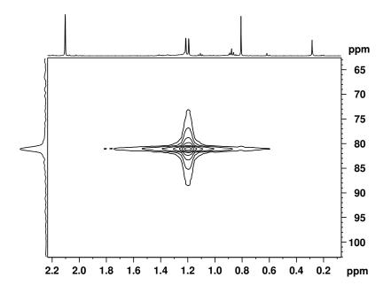
**Figure 22.** { $^{1}$ H- $^{13}$ C} 2D NMR spectrum in C<sub>6</sub>D<sub>6</sub> showing correlation between the BO*C* quaternary carbon and the methyl groups on the borane ring.
