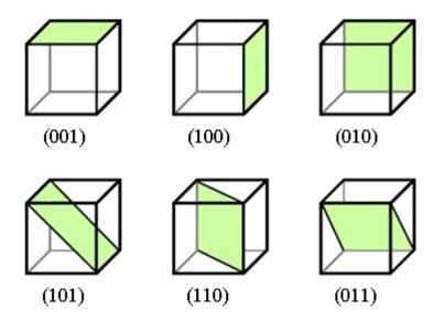
Figure 4. Miller indices in cubic crystals.
