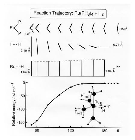
Figure 5. Calculated reaction profile and representation of changes for the  $\eta^1$  and  $\eta^2$  approaches of H\_2 to [Ru(PH\_3)\_4].^{11}
