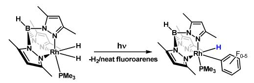
**Scheme 8.** Photochemical reaction of complex Tp`Rh(PMe<sub>3</sub>)H<sub>2</sub> in neat fluoroarenes to form the Tp`Rh(PMe<sub>3</sub>)(Ar<sup>F</sup>)(H) products.
