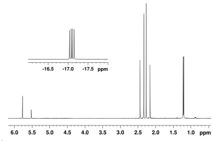
**Figure 3.** <sup>1</sup>H NMR spectrum in  $C_6D_6$  for the Tp`Rh(PMe<sub>3</sub>)H<sub>2</sub> starting material. The inset shows the hydride resonance.
