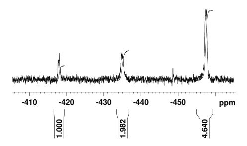
**Figure 19.** Low temperature <sup>19</sup>F NMR spectrum after photochemical reaction of complex Tp`Rh(CNneopentyl)( $\eta^2$ -PhN=C=N-neopentyl) in the presence of C<sub>5</sub>F<sub>5</sub>N.
