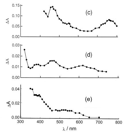
**Figure 1.**Transient UV/Vis spectra measured after solution laser flash photolysis (a)(d) 400 ns after flash and (e) 300 ns after flash. (a) Spectrum of  $Ru(dmpe)_2$  in cyclohexane under argon, (b) spectrum of  $Ru(depe)_2$  in heptane under 11 torr of  $H_2$ , (c) spectrum of  $Ru(dppe)_2$  in cyclohexane under 760 torr of  $H_2$ , (d) spectrum of  $Ru(dfepe)_2$  under 760 torr of  $H_2$ and (e) spectrum of  $Ru(dmpm)_2$  under 100 torr of  $H_2$ .<sup>3</sup>
