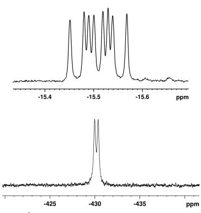
**Figure 11.** Top: <sup>1</sup>H NMR spectrum, hydride resonance for the complex Tp`Rh( $C_5F_4N$ )(PMe<sub>3</sub>)H in  $C_6D_6$ . Bottom: <sup>19</sup>F NMR spectrum, fluoride resonance for the complex Tp`Rh( $C_5F_3NH$ )(PMe<sub>3</sub>)F in  $C_6D_6$ .
