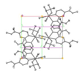
**Figure 7.** View of the crystal packing in  $P2_1/c$  for complex **5** along *b* with representation of the symmetry elements. Green: Two-fold screw axes; Pink: Glide planes perpendicular to *b*; Light orange: Inversion centers.
