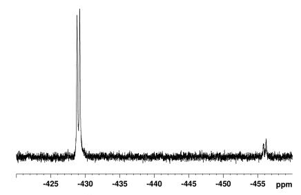
**Figure 5.** Low temperature <sup>19</sup>F NMR spectrum showing the presence of the two ortho conformers.
