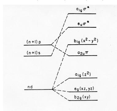
**Figure 2.** The molecular orbital energy diagram proposed for a square planar  $MP_4$  complex with a  ${}^{1}A_{1g}$  ground state assuming  $D_{4h}$  symmetry.<sup>12</sup>
