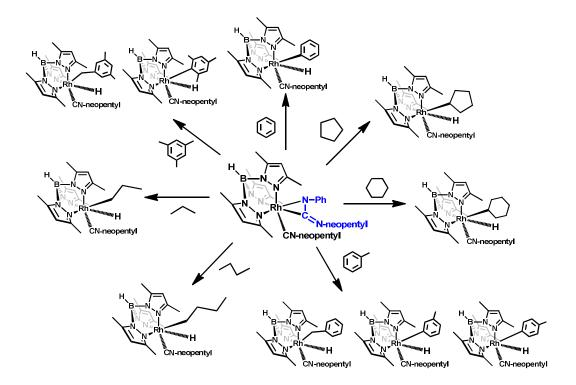
**Scheme 2.** C-H activation achieved in photochemical reactions of complex Tp`Rh(CNneopentyl)( $\eta^2$ -PhN=C=N-neopentyl) with different aromatic and aliphatic hydrocarbons.
