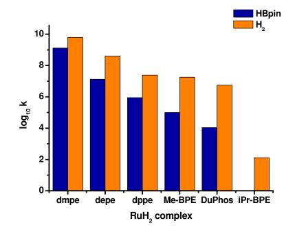
**Figure 17.** Plot of  $log_{10} k_2$  versus the different  $Ru(PP)_2H_2$  complexes in the presence of HBpin (blue) and  $H_2$  (orange) where k is the second order rate constant.
