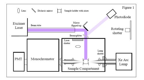
Scheme 10. Schematic representation of the LFP apparatus.
