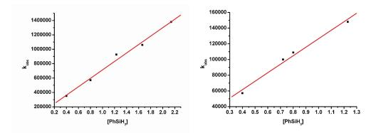
**Figure 9.** Plot of the pseudo first order rate constants,  $k_{obs}$  vs the concentration of PhSiH<sub>3</sub>:  $\Lambda$ -*R*,*R*-Ru1H<sub>2</sub> – left,  $\Lambda$ -*R*,*R*-Ru2H<sub>2</sub> – right.
