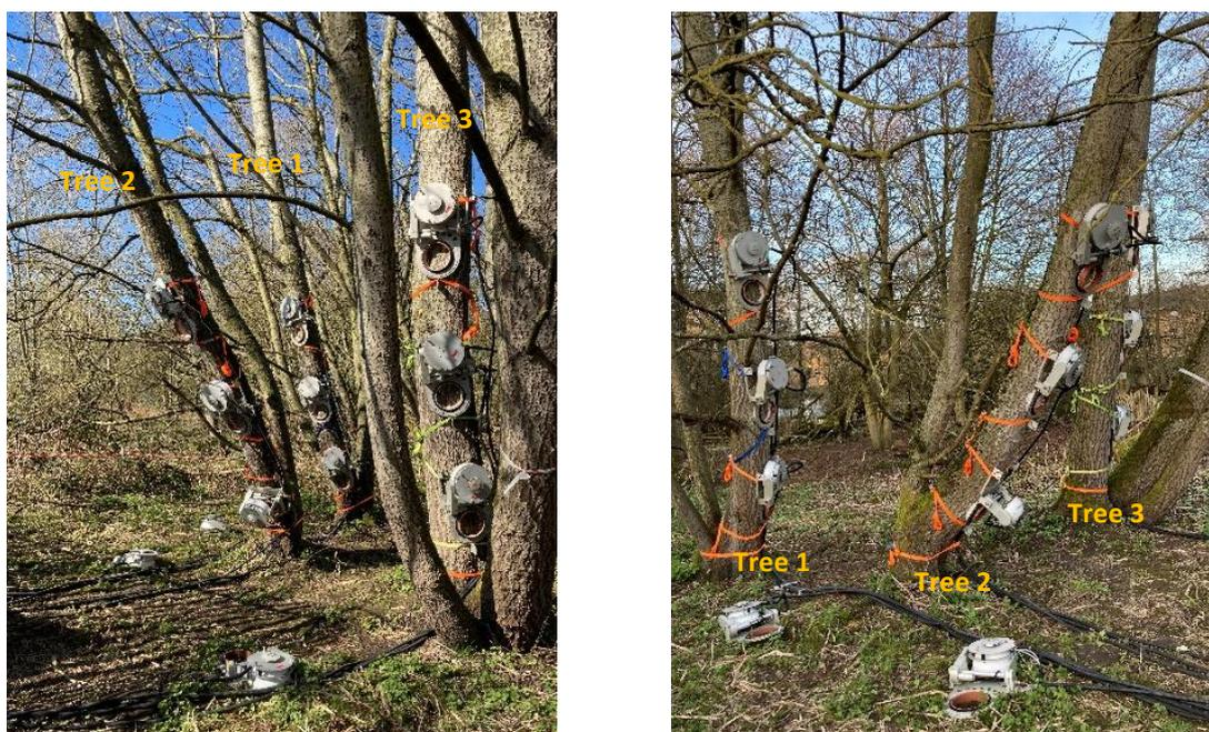
**Figure 4. 1** Automatic long-term chambers (LI-8100-101, Li-Cor, Lincoln, Nebraska, USA) on soils and three white poplar stems at 45, 130 and 200 cm above the soil surface. Tree 1, tree 2 and tree 3 were marked shown as in the pictures.
