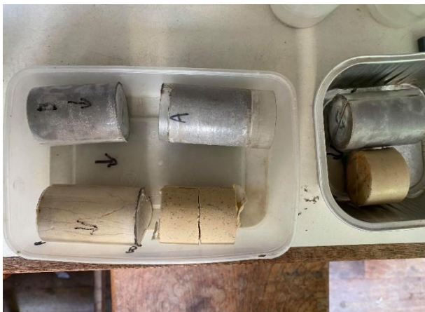
Figure 4.1: Photo of Limestone and Dolostone core samples after the closed-loop experiment. Limestone samples B, A and D and Dolostone samples B6, B2 and B1.
