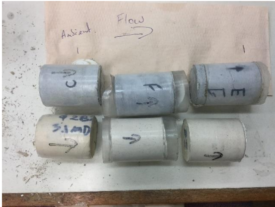
Figure 4.3: Photo of Limestone and Dolostone core samples after the open-loop experiment. Limestone samples C, F and E and Dolostone samples B5, B4 and B3.
