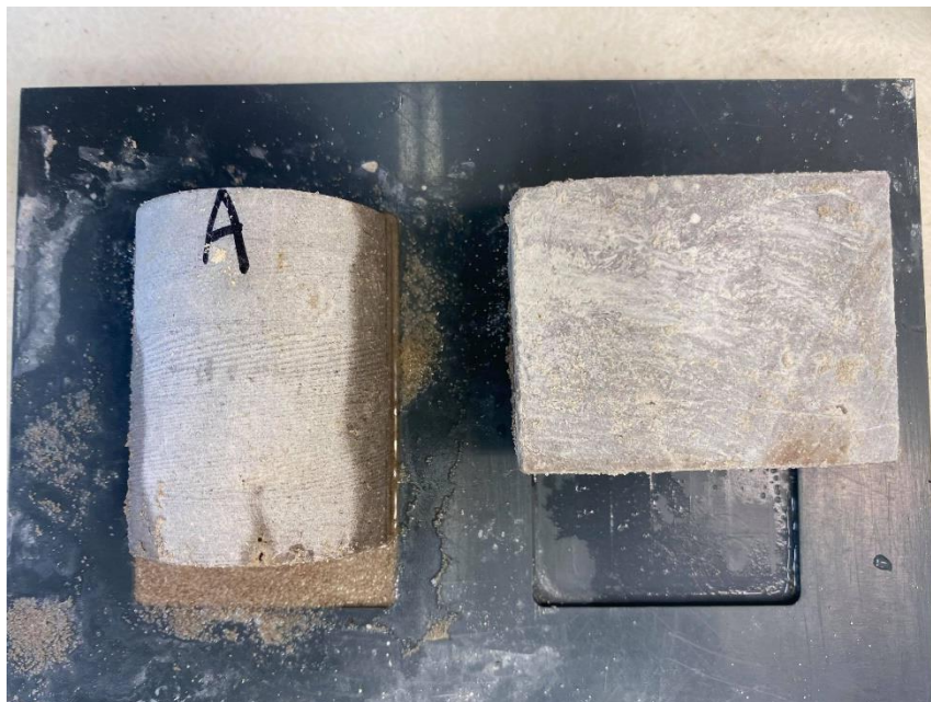
Figure 3.6: Picture of the preparation of the saturated limestone sample A before being frozen. Crushed limestone grains between 200 and 250 microns were placed into a rectangular dish. One half of the limestone core sample was placed on top so that the grains would freeze to the sample. The other half was frozen. Once the halves were frozen, they were placed together in a plastic tube which was heated and consequently moulded to the sample to hold it together.
