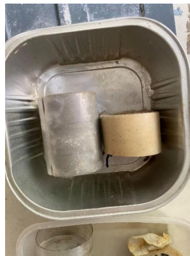
Figure 4.2: Limestone sample D and Dolostone sample B1 (closed-loop). Dolostone sample B1 was cut in half due to thinking there was an issue with the sample blocking fluid flow. This was discovered as a leak and nothing to do with the sample. This is discussed later in section 4.5.
