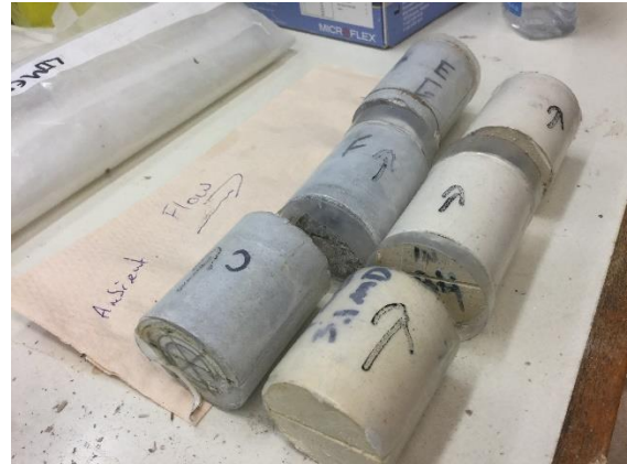
Figure 4.4: Photo of Limestone and Dolostone core samples after the open-loop experiment. Limestone samples C, F and E and Dolostone samples B5, B4 and B3.
