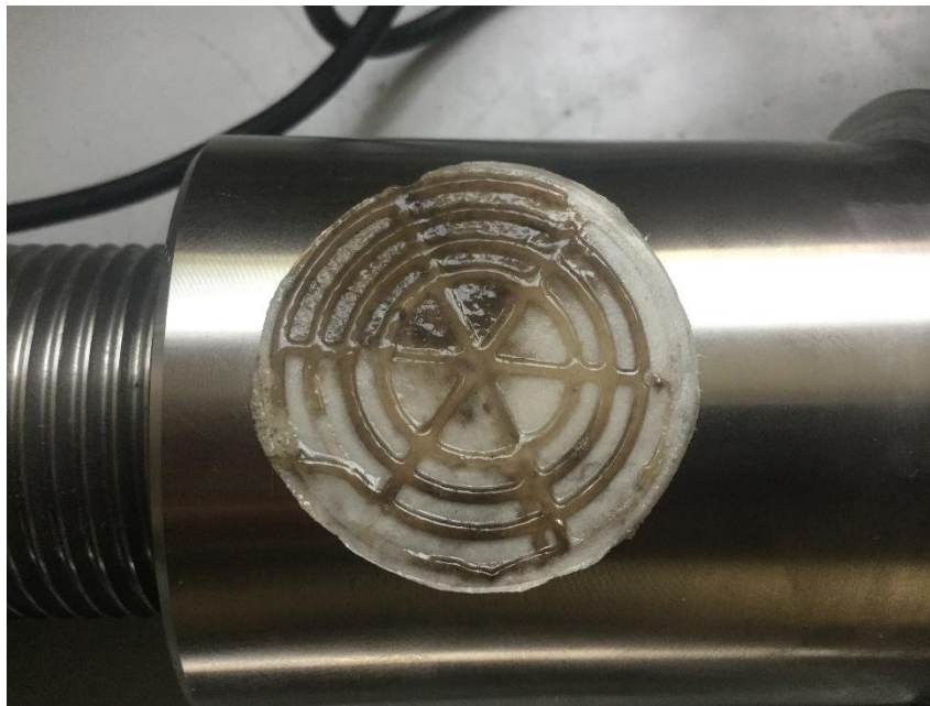
Figure 4.57: Residue left on the filter paper from the upstream (1A) of the first core holder in limestone (line one).
