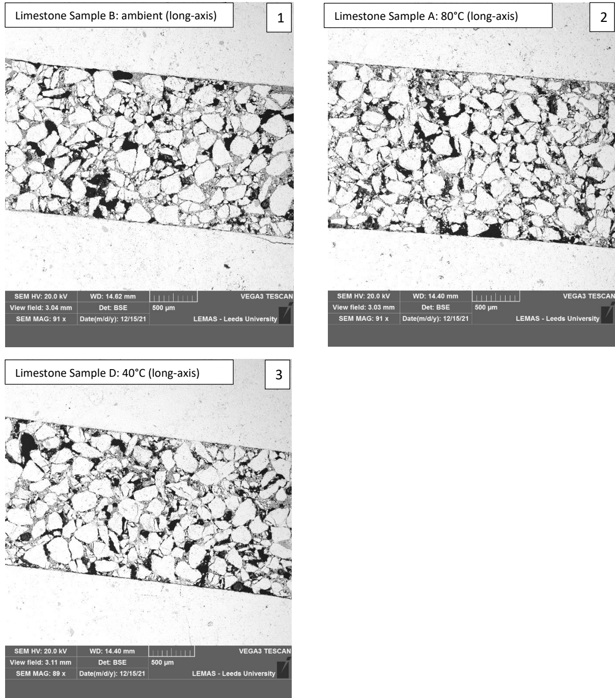
Figure 4.6.1, 4.6.2 and 4.6.3: Backscatter-Electron (BSE) images taken of the fracture from Limestone core samples B, A and D, located in the closed-loop experiment. All photographs are taken from the long-axis section. (1) Sample B was located in the ambient core holder, (2) sample A was located in the 80°C core holder and (3) sample D was located in the 40°C core holder. The white grains represent the limestone. The black areas represent porosity.
