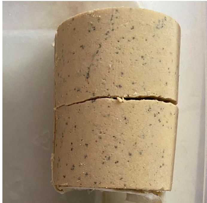
Figure 4.14: Photograph of Dolostone Sample B2 after the closed-loop experiment. An evident natural fracture has occurred during the experiment and was discovered after removal of the sample.
