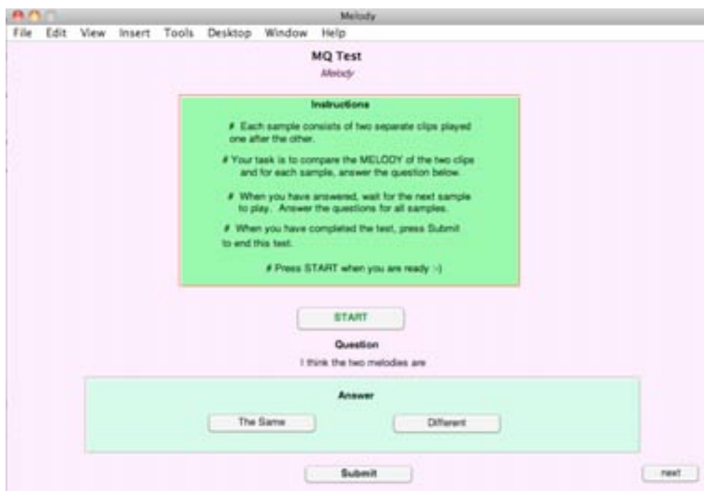
Figure 4.7 An example of the Melody subtest in LTware . Listeners press “Start” and hear two consecutive melodies. The sequential trials play automatically following the listeners answer selection. When the test is completed, listeners press “Submit” then click “next” for the subsequent subtest.
