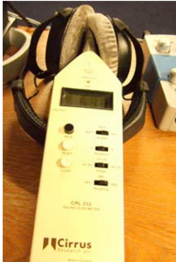
Figure 3.9. An example of using the sound level meter to measure the sound pressure level in the headphones.
