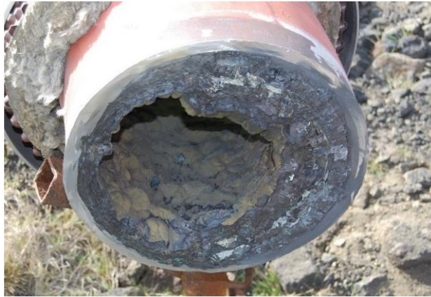
Figure 2.8: Metal sulphide scaling in 14" pipes close to wellhead. The metal sulphides form a tough scale on the downstream pipe surfaces [61].
