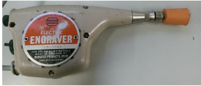
Figure 3.4: Modified engraver to tight pack the sand column
