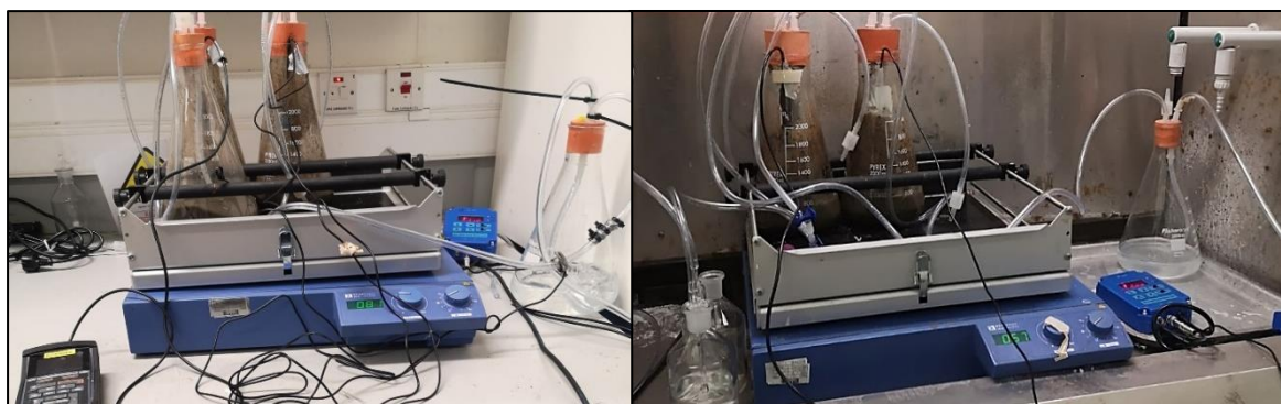
Figure 3.0: Schematic drawing of the experimental rig used to control redox potential. Three treatments of this design were simulated in tandem.
