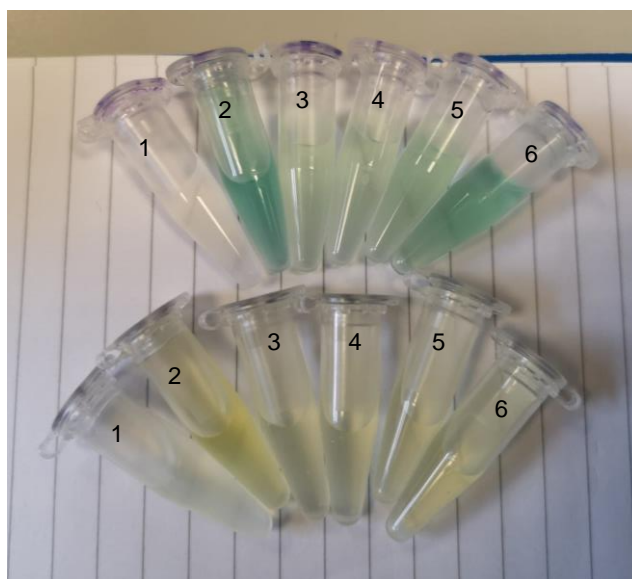
Figure 8.16 Coloured activity assays with the peroxidative activity assay with ABTS 118a on the top row and the peroxygenative activity with NBD 119a on the bottom row. The numbers correspond to the samples as follows: 1. Negative control 2. rAaeUPO, 3. artUPO yeast with direct pH adjustment 4. artUPO yeast after dialysis 5. artUPO yeast in crude fermentation culture 6. Purified artUPO yeast from shake flask expression
