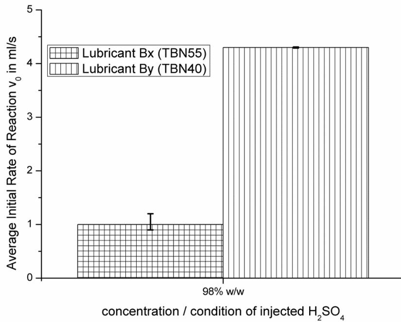
Figure 3.24: Initial rate of reaction for lubricants from manufacturer B with lower alkaline reserve for operation on low sulphur fuel
