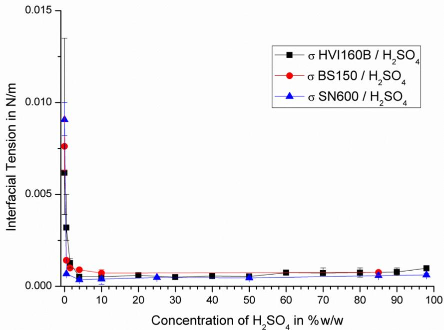
**Figure 4.10: Results of interfacial tension measurements between API Group I base oils and aqueous sulphuric acid at 22 °C after heating to 90 °C**
