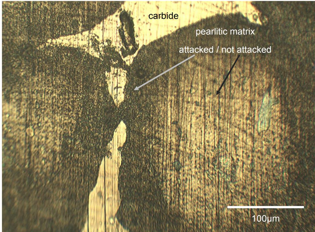
**Figure 5.8: Corrosive attack on grey cast iron after contact angle measurements with 25 %w/w H<sub>2</sub>SO<sub>4</sub> at 20 °C**
