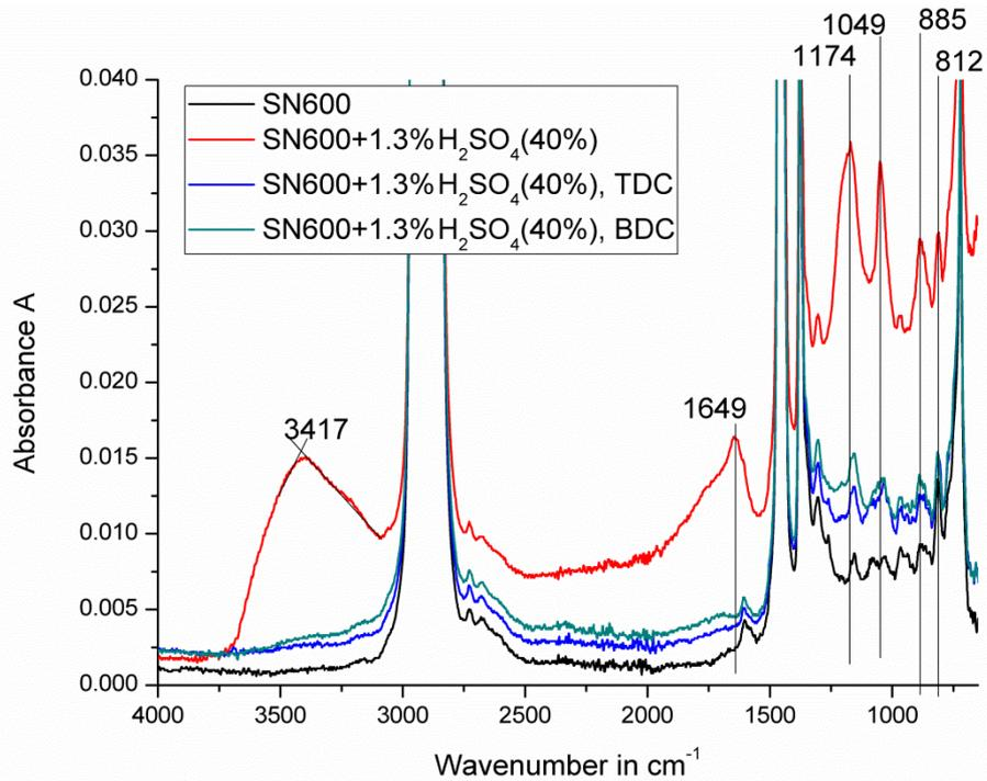
**Figure 7.20: FTIR-ATR spectra of SN600+1.3%v/v40%w/wH<sub>2</sub>SO<sub>4</sub>, fresh and sampled during the friction test at 80 °C. Test no. 6.**
