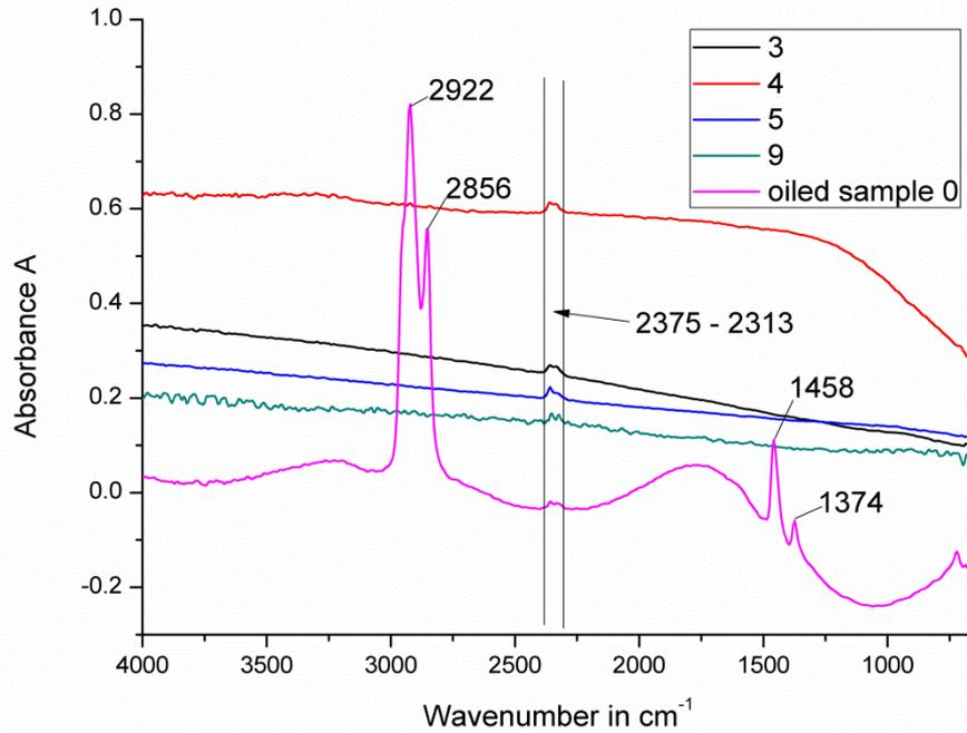
**Figure 7.26: FTIR-spectra of the areas indicated in Figure 7.25**
