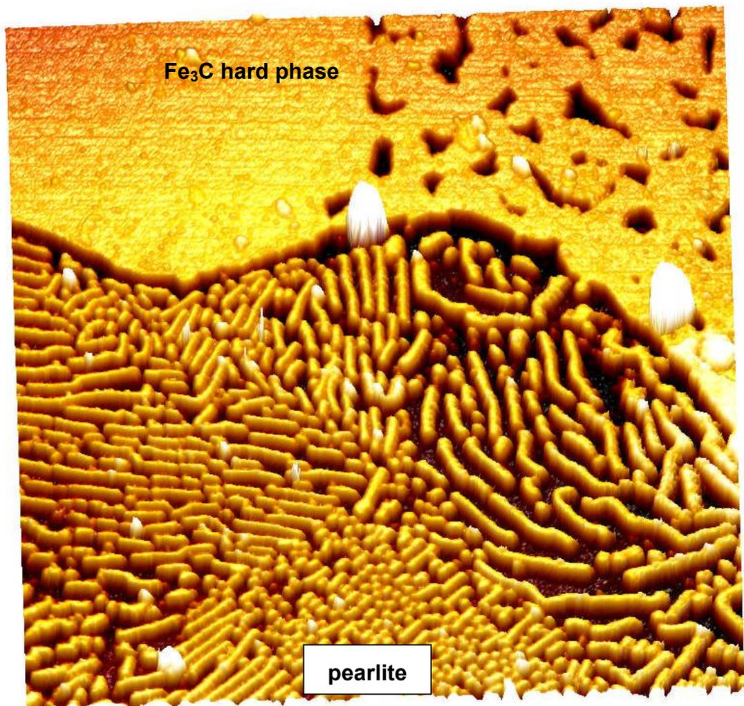
**Figure 8.12: 100x100 $\mu\text{m}$  AFM scan of grey cast iron polished and etched with NITAL. Iron and iron phosphide removed by  $\sim 100$  nm**
