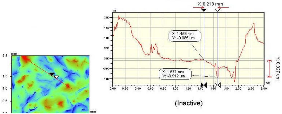
Figure 8.2: Distance between pearlitic matrix and graphite lamella at 20 °C
