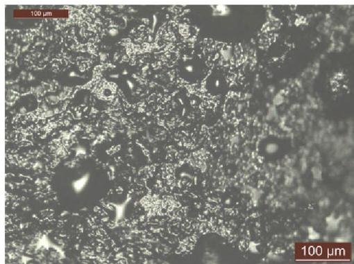
**Fig. 20** Deposit formed during viscosity measurements at 150 °C with the water washed bitumen created with 98 %w/w H<sub>2</sub>SO<sub>4</sub>. Magnification: ×100
