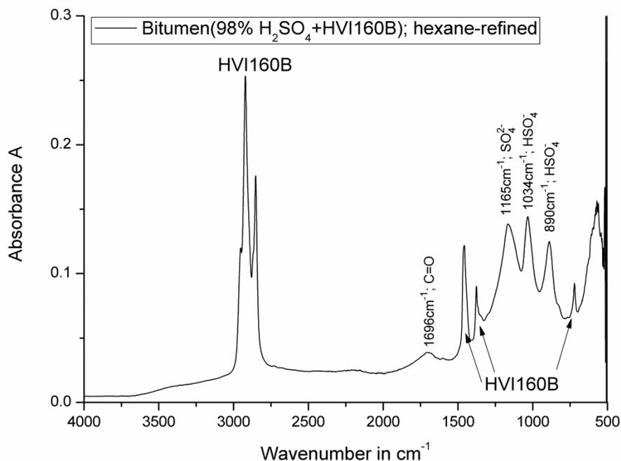
**Figure 4.14: FTIR-ATR spectrum of hexane-refined bitumen, formed between 98 %w/w H<sub>2</sub>SO<sub>4</sub> and API Group I base oil HVI160B at 90 °C and four weeks storing at room temperature**
