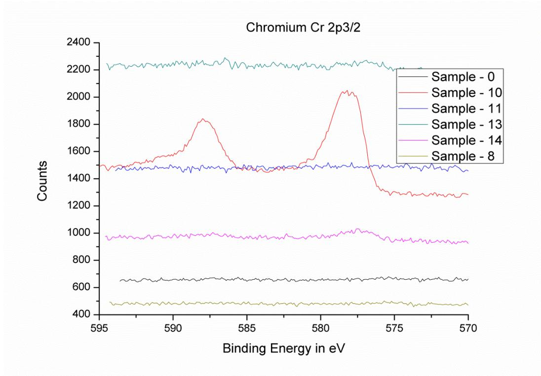
Figure 7.43: Cr<sub>2p<sub>3/2</sub></sub> XPS spectra for all cylinder liner wear scars
