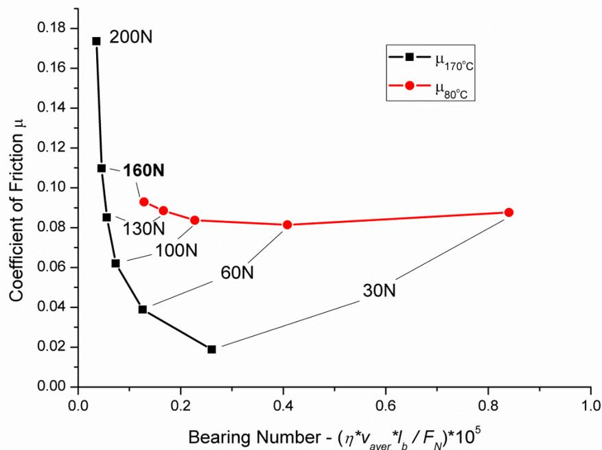
**Figure 7.3: Partial Stribeck diagram for piston ring cylinder liner contact lubricated with SN600 at 80 and 170 °C.**
