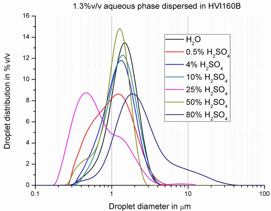
**Figure 3.19: Droplet size distribution of 1.3 %v/v aqueous H<sub>2</sub>SO<sub>4</sub> dispersed in API Group I base oil HVI160B**
