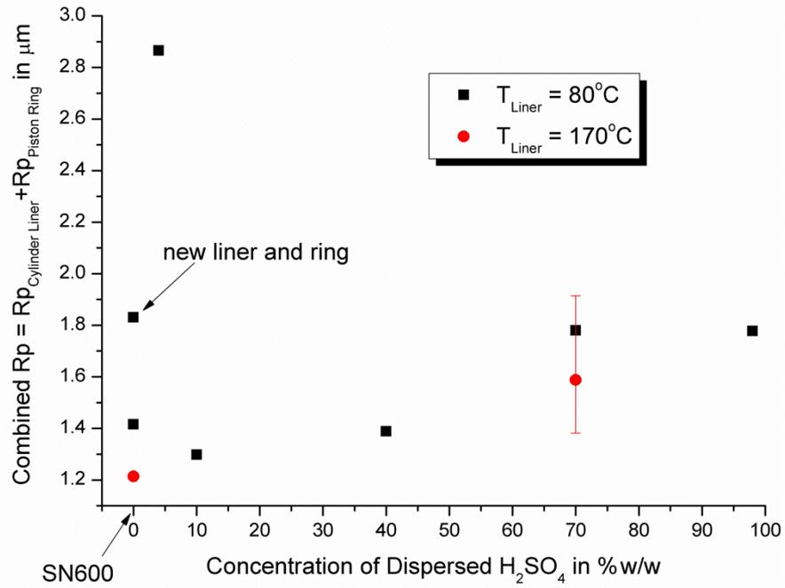
Figure 7.46: Combined roughness peak height form the mean line,  $R_p$ , for piston ring and cylinder liner
