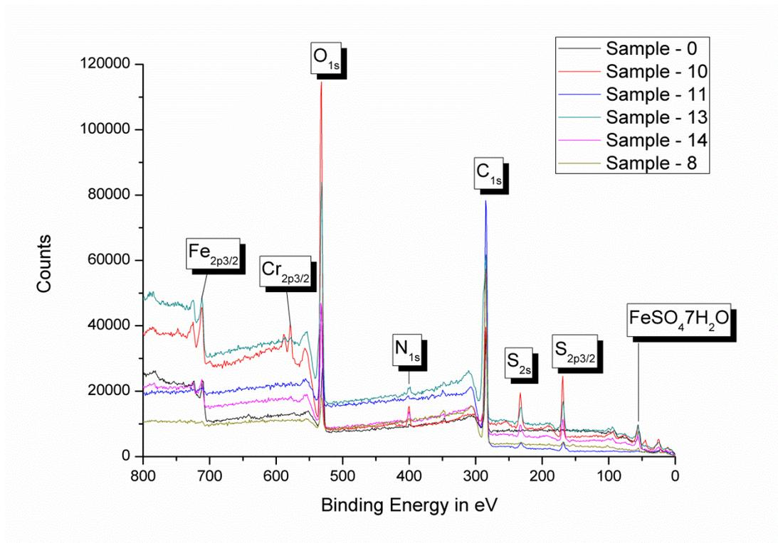
**Figure 7.38: Overall XPS spectra for all cylinder liner wear scars**
