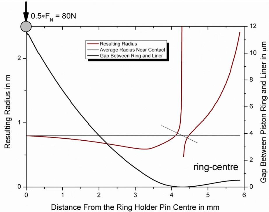
Figure 6.29: Influence of Hertzian contact pressure on piston ring deformation and conformity of the parts in unworn condition on the TE77 test bed according to the model shown in Figure 6.28
