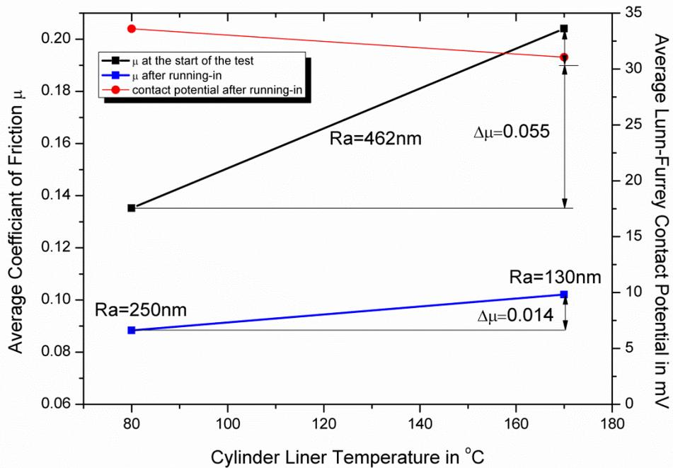
**Figure 7.1: Coefficient of friction before and after running-in with SN600 and the corresponding contact potential measurement after running-in.**
