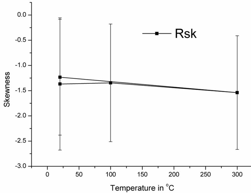
**Figure 8.5: Change in surface skewness over temperature. Error bars indicate the standard deviation from the mean**
