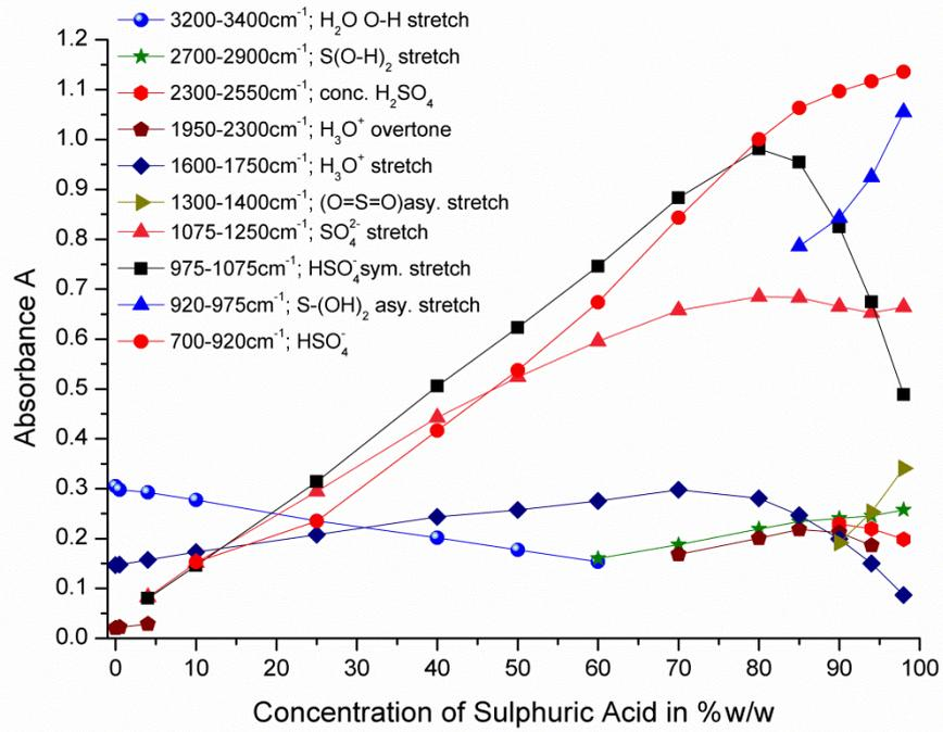
Figure 3.15: FTIR-ATR absorbance in correlation to the concentration of  $\text{H}_2\text{SO}_4$
