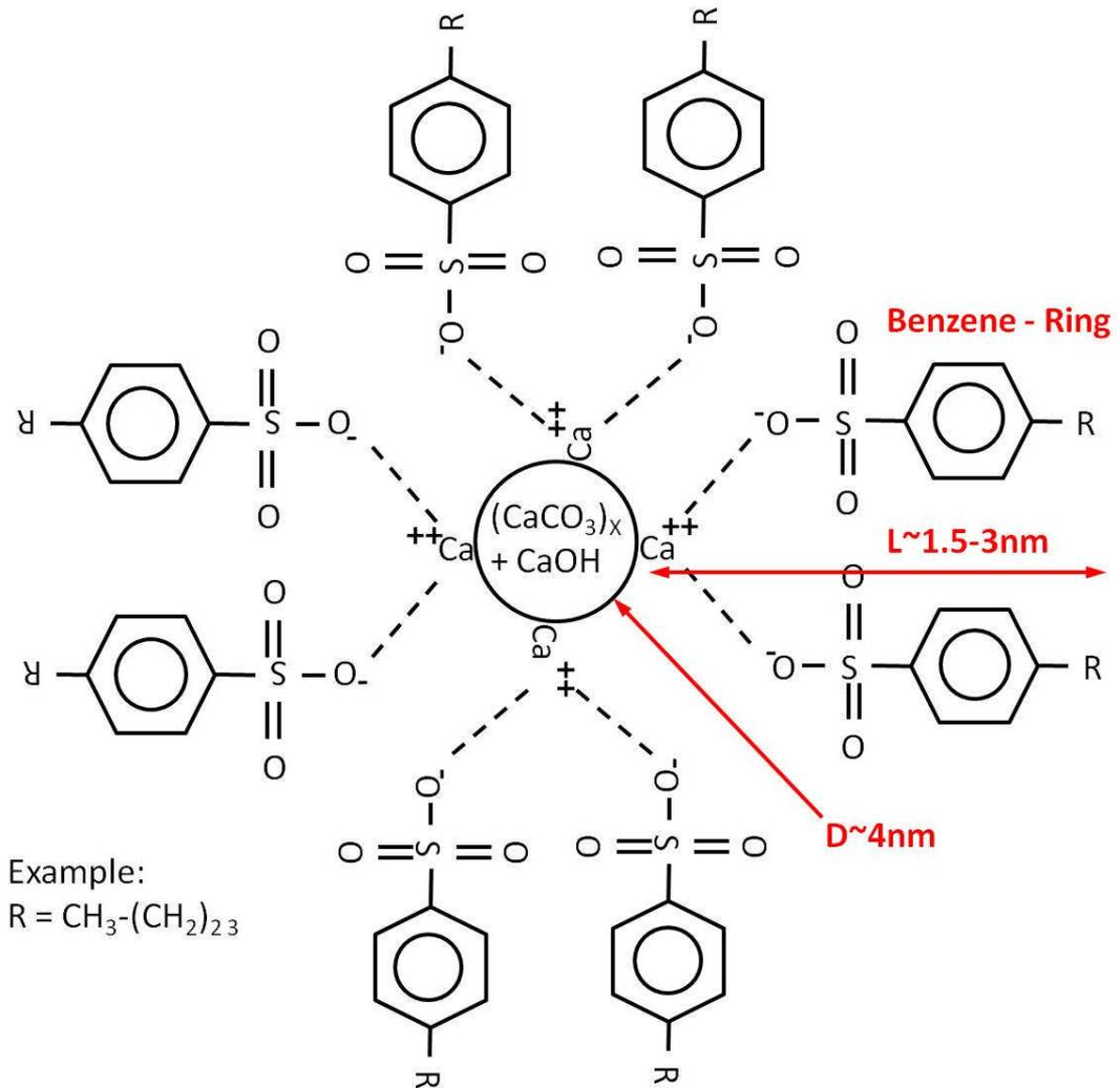
**Figure 2.1: Schematic of a overbased calcium sulphonate reverse micelle containing  $\text{CaCO}_3$  particles and  $\text{CaOH}$  in aqueous solution (Kubo, et al., 2006), (Giasson, et al., 1993), (Wu, et al., 2000) and (Topolovec-Miklozic, et al., 2008)**
