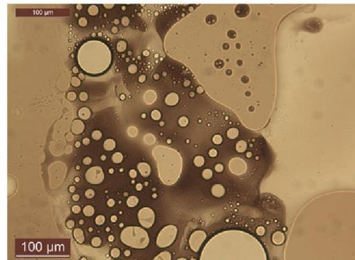
**Fig. 17** Microscopic view on bituminous matter formed between 98 %w/w H<sub>2</sub>SO<sub>4</sub> and HVI160B before separating from oil phase. Magnification: ×100
