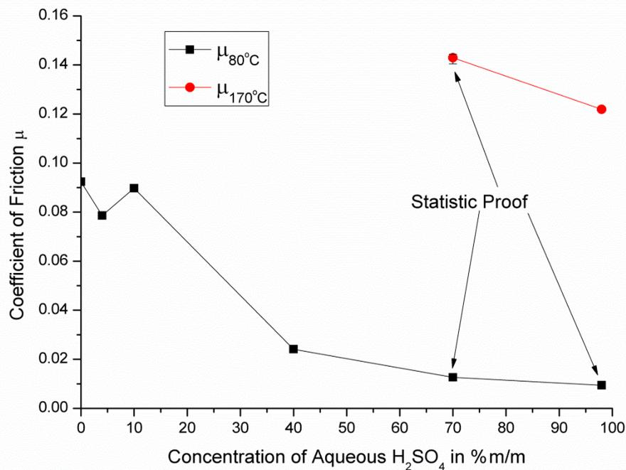
**Figure 7.4: Coefficient of friction for various concentrations of aqueous H<sub>2</sub>SO<sub>4</sub> dispersed in SN600 at 80 and 170 °C**
