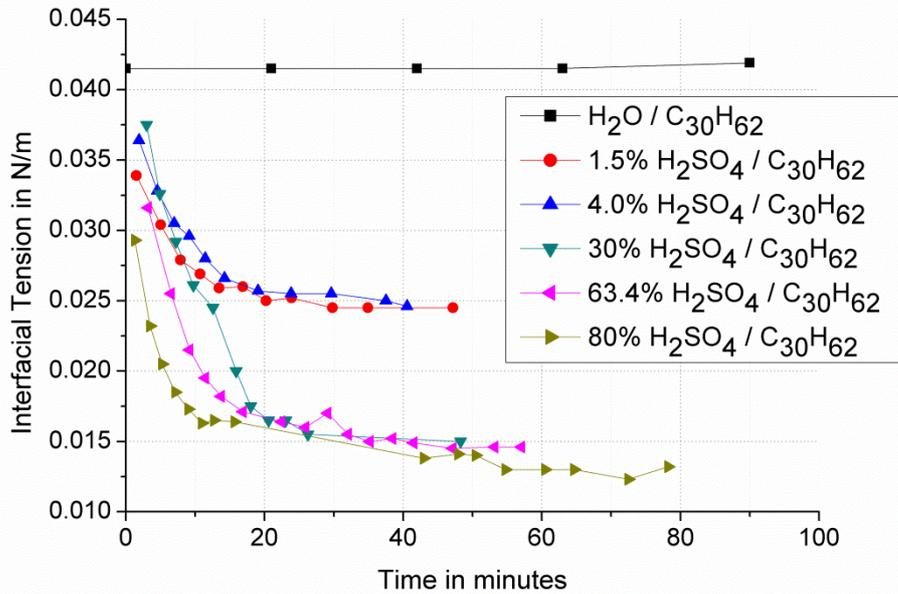
**Figure 4.7: Time dependent development of interfacial tension between water (H<sub>2</sub>O), aqueous concentrations (%w/w) of H<sub>2</sub>SO<sub>4</sub> and C<sub>30</sub>H<sub>62</sub> at 20 °C**
