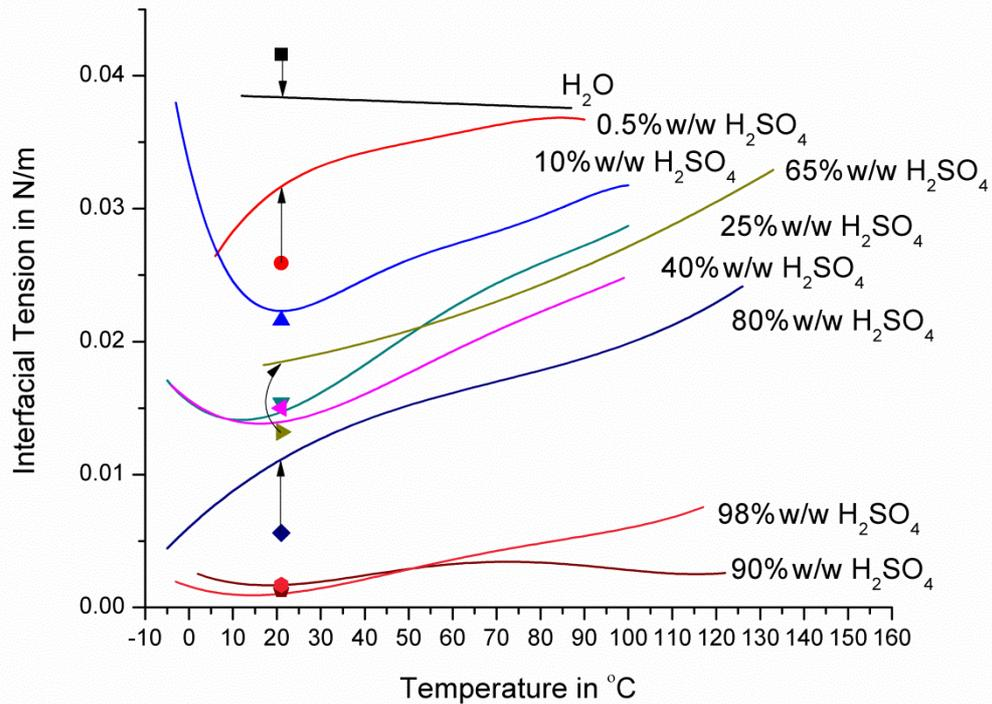
**Figure 4.12: Concentration and temperature dependency of the interfacial tension between sulphuric acid,  $H_2SO_4$ , and squalane,  $C_{30}H_{62}$ . The values from Figure 4.9 are added for comparison.**
