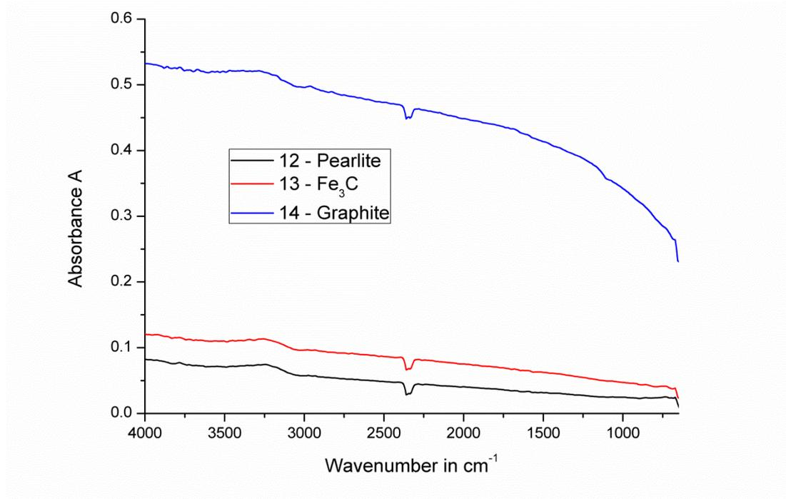
**Figure 8.9: FTIR measurement scan on highly polished grey cast iron marine Diesel cylinder liner material. Spectra were taken at the positions indicated in Figure 8.8.**
