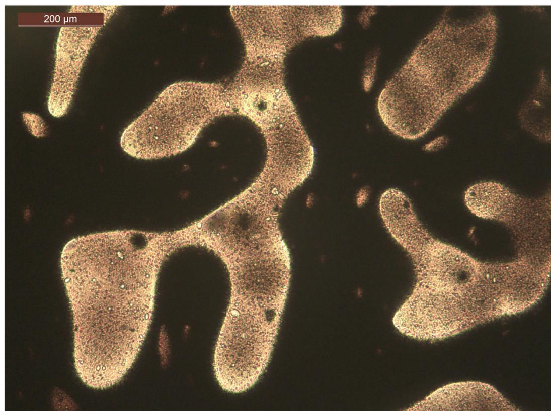
**Figure 3.7: Microscopic view on bituminous matter formed between 98 %w/w  $\text{H}_2\text{SO}_4$  and HVI160B after separating from oil phase in water. Squeezed between microscope slides. 50x**
