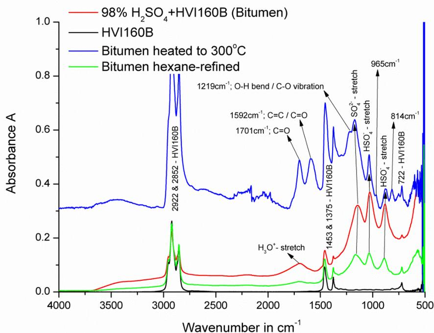
**Figure 3.1: Bitumen formed between HVI160B and 98%w/w  $\text{H}_2\text{SO}_4$  at various treatment stages.**
