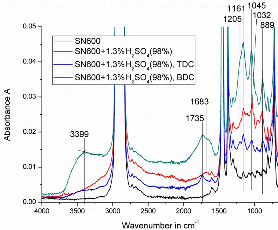
**Figure 7.22: FTIR-ATR spectra of SN600+1.3%v/v98%w/wH<sub>2</sub>SO<sub>4</sub>, fresh and sampled during the friction test at 80 °C. Test no. 9.**
