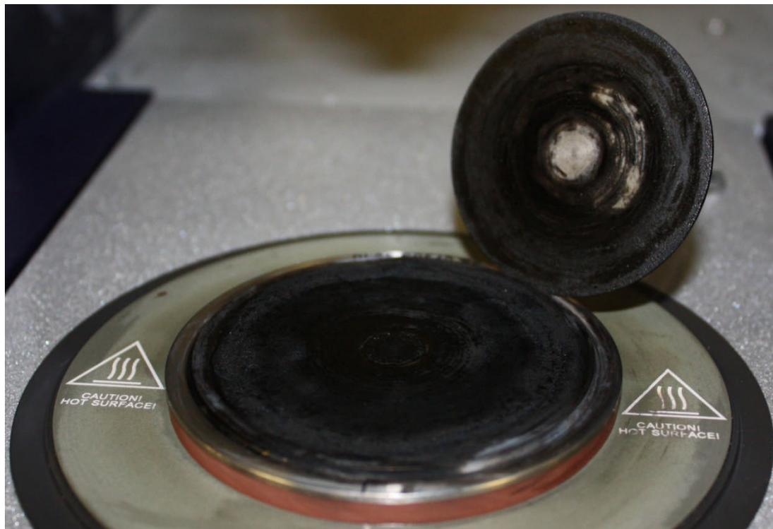
**Figure 3.35: Solidification of bitumen formed between HVI160B and 98 %w/w H<sub>2</sub>SO<sub>4</sub> during viscosity measurements at 150 °C**
