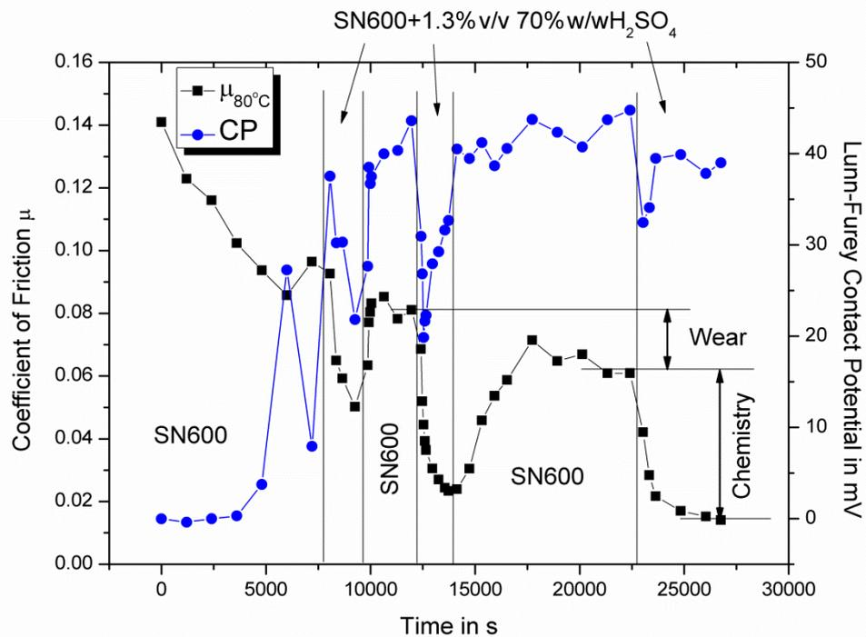
**Figure 7.5: Shuttle test between pure SN600 and SN600 + 70 %  $H_2SO_4$  at 80 °C, revealing the influence of wear and chemistry on friction**
