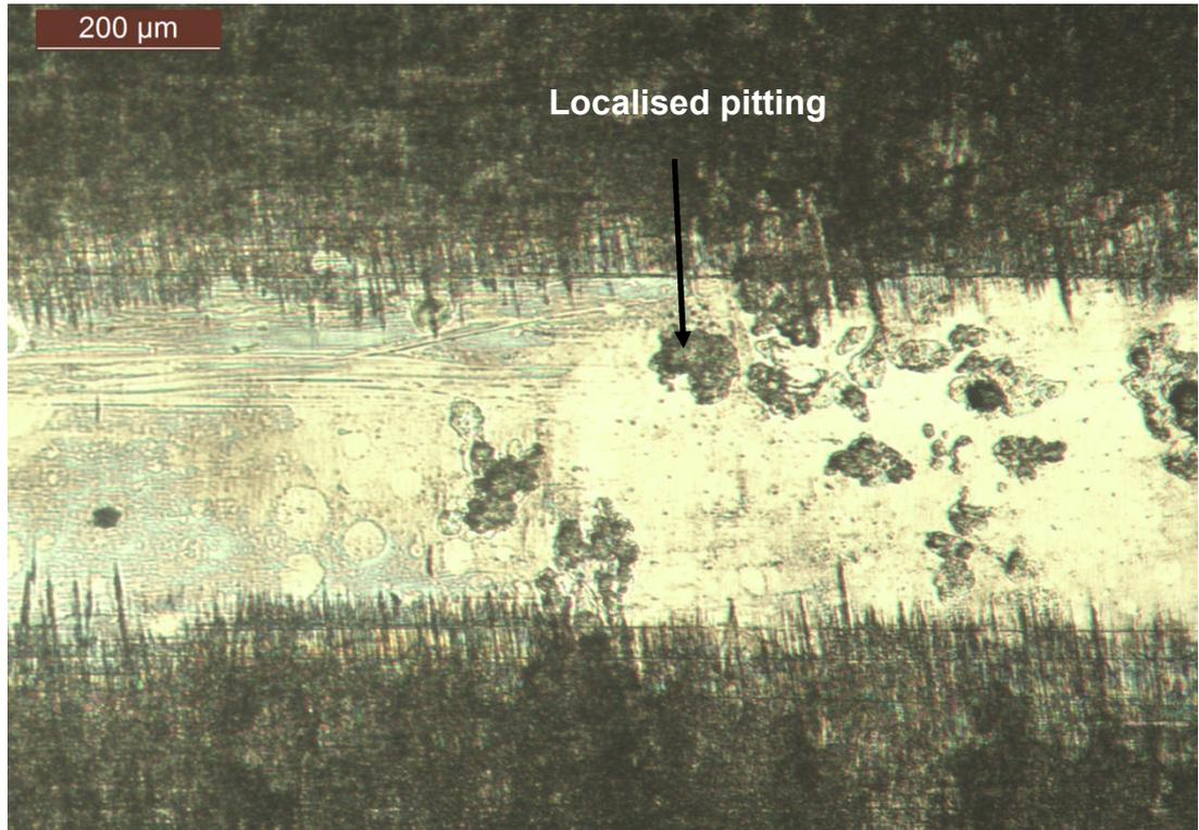
**Figure 7.12: Piston ring wear scar, test 10, lubricated with SN600 + 70 %w/w H<sub>2</sub>SO<sub>4</sub> at 80 °C**
