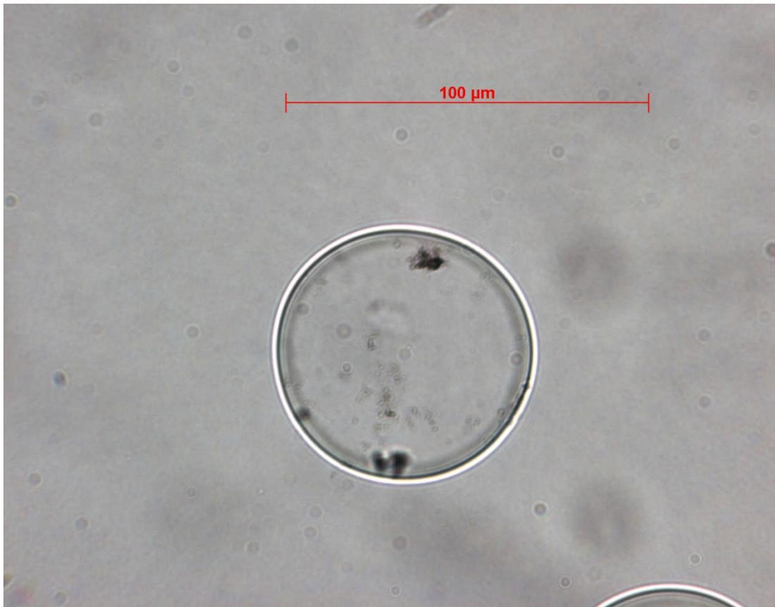
**Figure 3.4: Transmission microscopic image of the acid phase (80 %w/w  $H_2SO_4$ ) below  $C_{30}H_{62}$  exposed to 165 °C**
