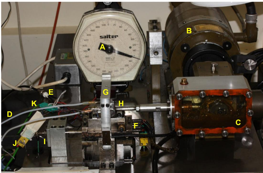
**Figure 6.7: Overview of the TE77 friction testing machine**
