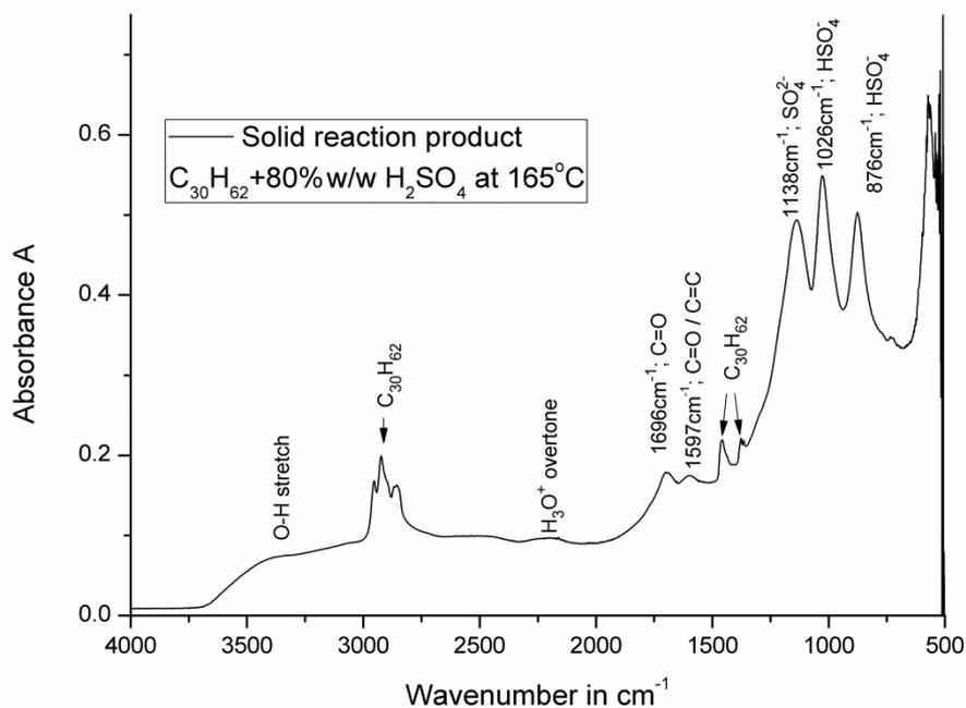
**Figure 4.13: FTIR-ATR spectrum of a solid formed between C<sub>30</sub>H<sub>62</sub> and 80 %w/w H<sub>2</sub>SO<sub>4</sub> at 165 °C**
