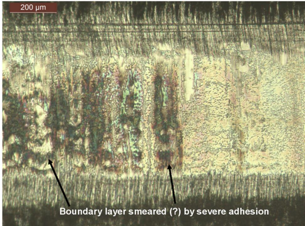
Figure 14: Piston ring wear scar, lubricated with lubricant B & SN600 + 70 %w/w H<sub>2</sub>SO<sub>4</sub> at 170 °C. The test finished after an 53 minute period of adding lubricant B.
