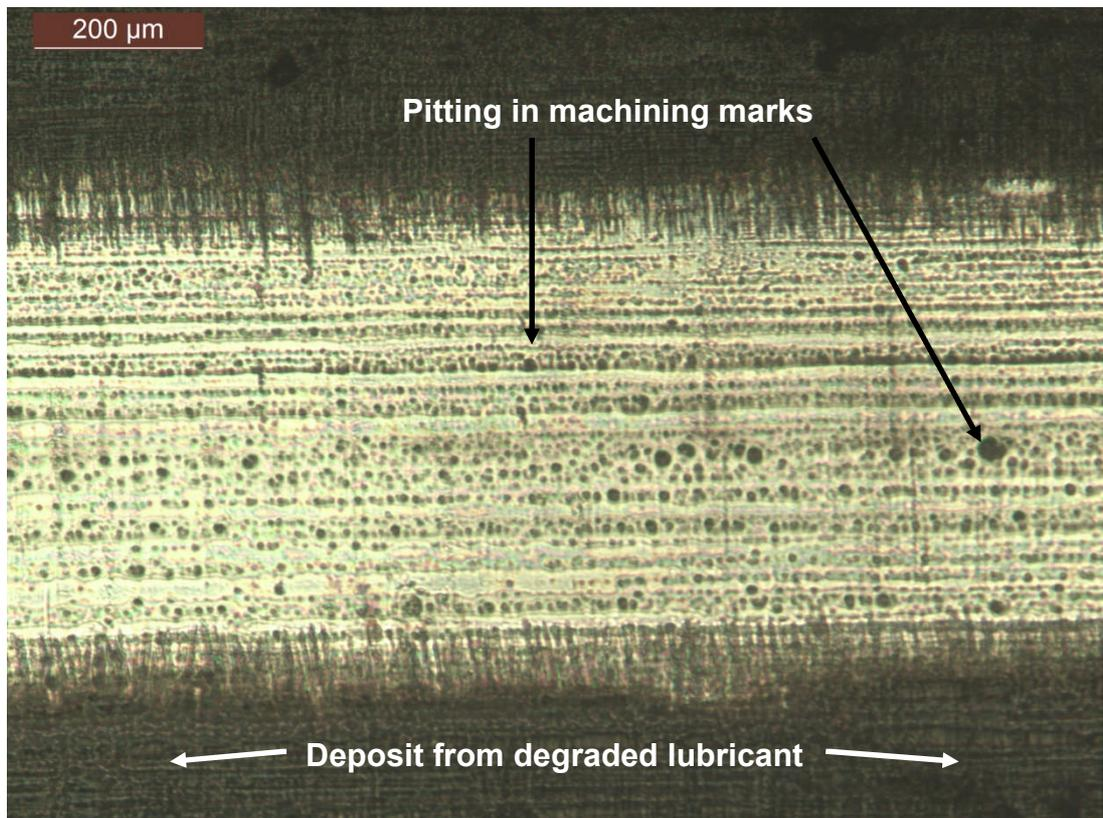
**Figure 7.13: Piston ring wear scar, test 12, lubricated with SN600 + 70 %w/w H<sub>2</sub>SO<sub>4</sub> at 170 °C**
