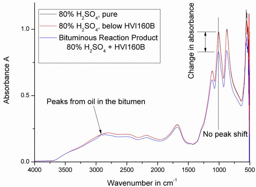
Figure 3.16: FTIR-ATR absorbance spectra of pure 80 %w/w  $\text{H}_2\text{SO}_4$ , remaining acid used in the reaction and the reaction product
