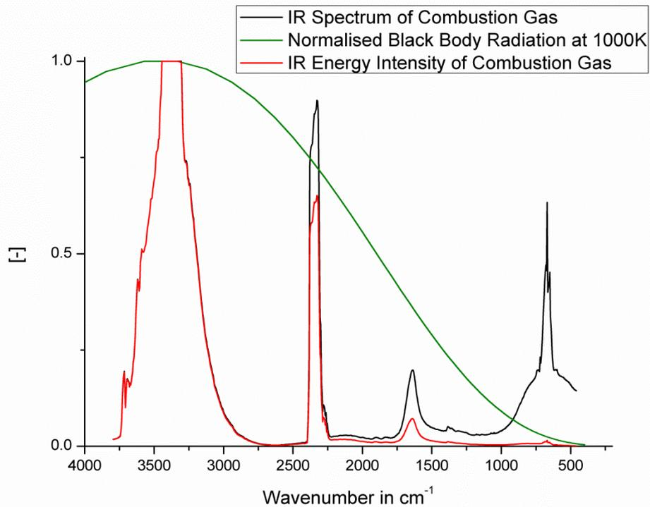
**Figure 8.6: Infra red radiation of a black body at 1000 K and estimated chromatographic combustion gas radiation. Combustion gas composition according Table 8.1**
