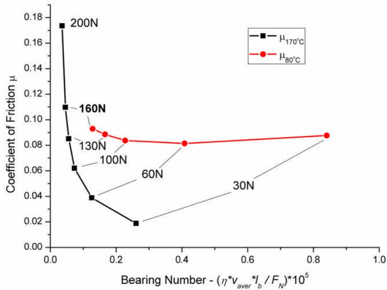
Figure 4: Partial Stribeck diagram for piston ring cylinder liner contact lubricated with SN600 at 80 and 170 °C.
