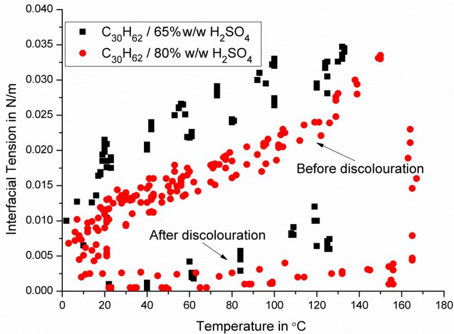
**Figure 4.11: Temperature dependent interfacial tension of 65 % and 80 %w/w H<sub>2</sub>SO<sub>4</sub> towards C<sub>30</sub>H<sub>62</sub>**
