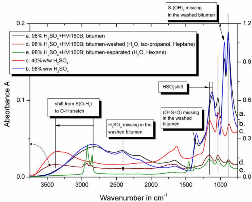
**Figure 4:** FTIR-ATR absorbance spectra of bituminous reaction product (a.), solvent washed bituminous reaction product (d.), solvent separated bituminous reaction product (e.) and pure 40 %w/w and 98 %w/w  $H_2SO_4$  (c. and b.).
