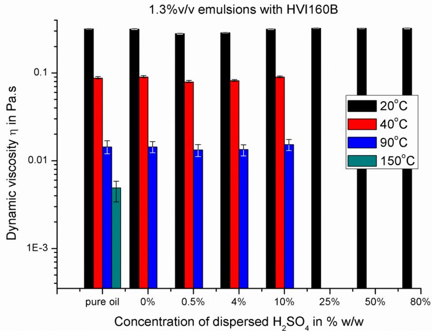
**Figure 3.31: Viscosity of pure and emulsified API Group I base oil HVI160B with 1.3 %v/v aqueous H<sub>2</sub>SO<sub>4</sub> as dispersed phase. Applied shear rate was 200 – 700 s<sup>-1</sup>**
