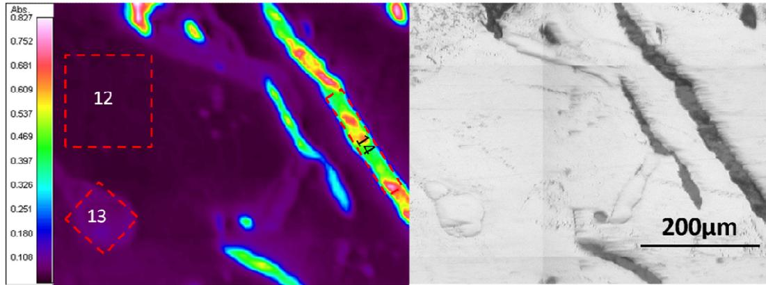
**Figure 8.8: FTIR-scan and visual image on highly polished grey cast iron marine Diesel cylinder liner material. Position 12 is the pearlite matrix, 13 a  $\text{Fe}_3\text{C}$  hard phase and 14 a graphite lamella.**
