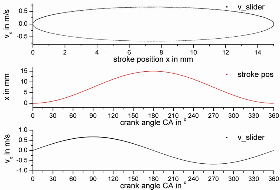
Figure 6.17: Kinetics of the Scotch-Yoke mechanism
