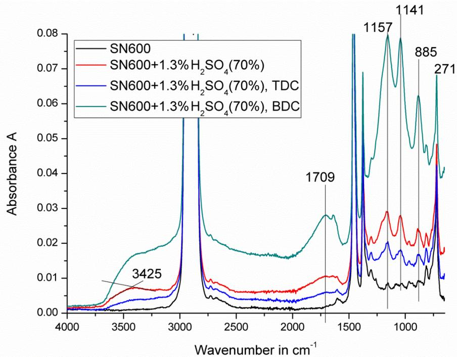
**Figure 7.21: FTIR-ATR spectra of SN600+1.3%v/v70%w/wH<sub>2</sub>SO<sub>4</sub>, fresh and sampled during the friction test at 80 °C. Test no. 7.**
