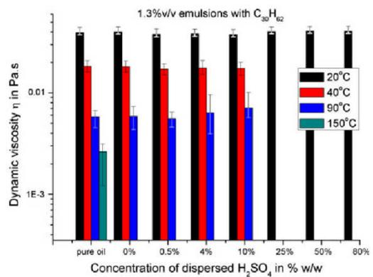
Fig. 9 Viscosity of pure and emulsified C<sub>30</sub>H<sub>62</sub> with 1.3 %v/v aqueous H<sub>2</sub>SO<sub>4</sub> as dispersed phase. Applied shear rate was 200–700 s<sup>-1</sup>
