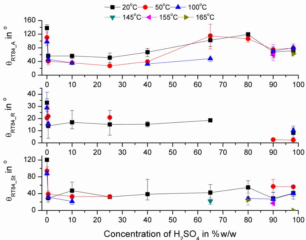
**Figure 5.4: Contact angle measurement results for cylinder liner grey cast Iron, RT84, over H<sub>2</sub>SO<sub>4</sub> concentration and at various temperatures**
