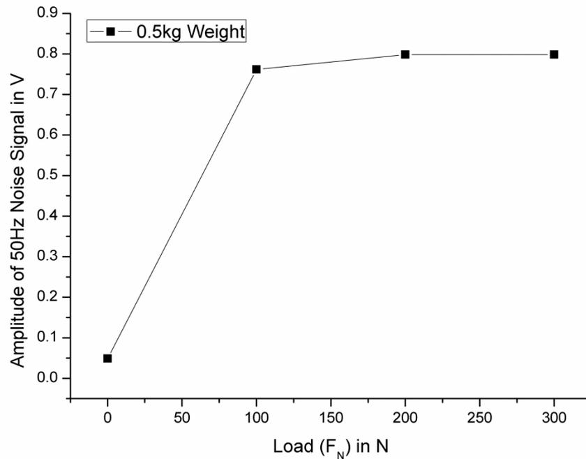
**Figure 6.15: Amplitude of 50 Hz noise in correlation to increasing normal force**
