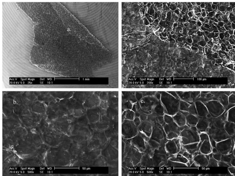
Fig. 5. SEM pictures of solid reaction product created between 80% w/w  $H_2SO_4$  and  $C_{30}H_{62}$  at  $165\text{ }^\circ\text{C}$ : (a) overview; (b) top side; (c) bottom side.
