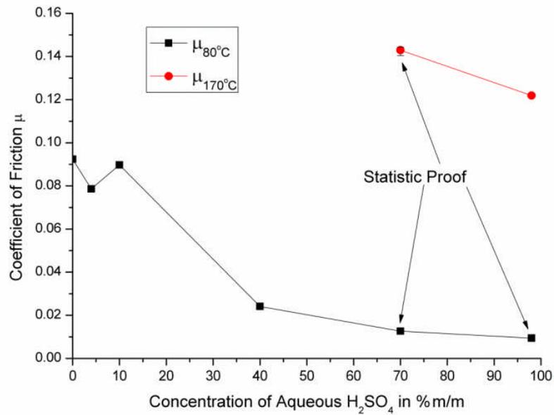
Figure 5: COF for various concentrations of aqueous H<sub>2</sub>SO<sub>4</sub> at 80 and 170 °C
