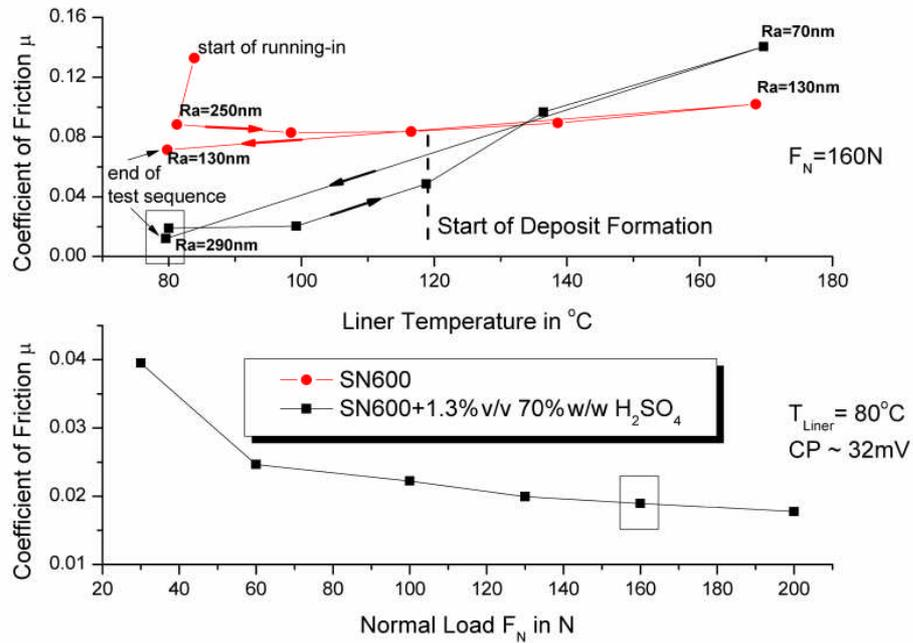
Figure 8: Influence of temperature and load on the COF
