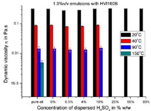
Fig. 8 Viscosity of pure and emulsified API Group I base oil HVI160B with 1.3 %v/v aqueous H<sub>2</sub>SO<sub>4</sub> as dispersed phase. Applied shear rate was 200–700 s<sup>-1</sup>
