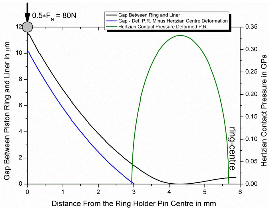
Figure 6.30: Influence of piston ring deformation on the Hertzian contact pressure and conformity of the parts in unworn condition on the TE77 test bed according to the model shown in Figure 6.28.
