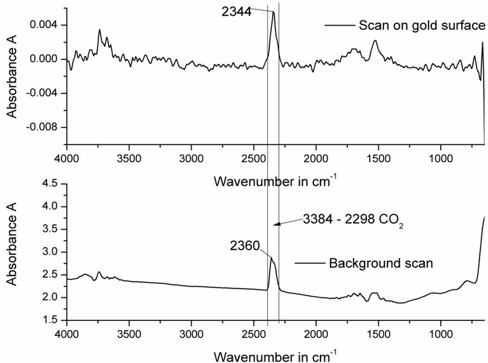
**Figure 7.27: FTIR background and measurement scan on a plain gold surface**
