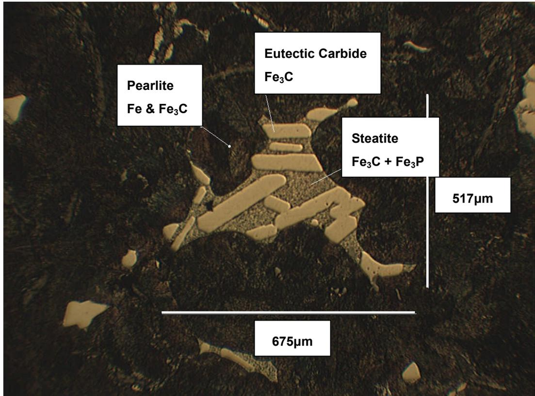
Figure 6.1: Hard phase of a marine cylinder liner grey cast iron
