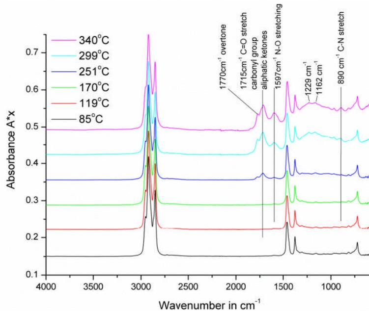
Figure 17: FTIR-ATR spectra of SN600 exposed to various cylinder liner temperatures during the friction tests at 85 - 340 °C
