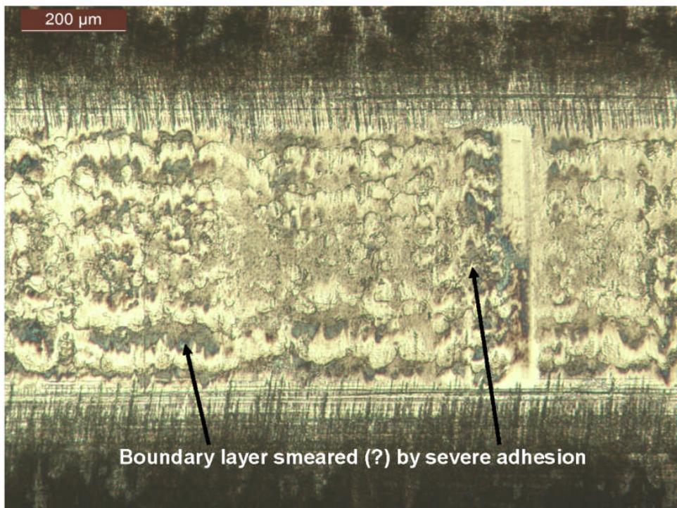
Figure 11: Piston ring wear scar, lubricated with SN600 at 170 °C for 6.5 hours
