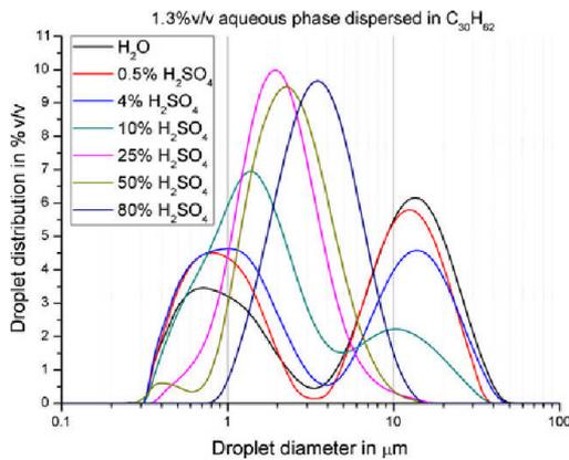
**Fig. 4** Droplet size distribution of 1.3 %v/v aqueous H<sub>2</sub>SO<sub>4</sub> dispersed in C<sub>30</sub>H<sub>62</sub>
