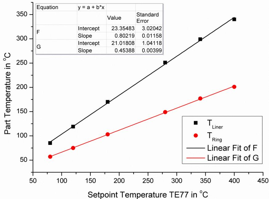
**Figure 6.11: Correlation of temperature control set point to piston ring and cylinder liner temperature in the running TE77 friction testing machine**
