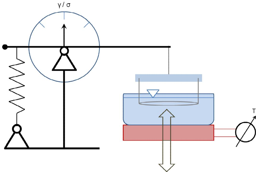
Figure 4.4: Schema of the Du-Nöuy ring surface tension balance with temperature controlled hot plate
