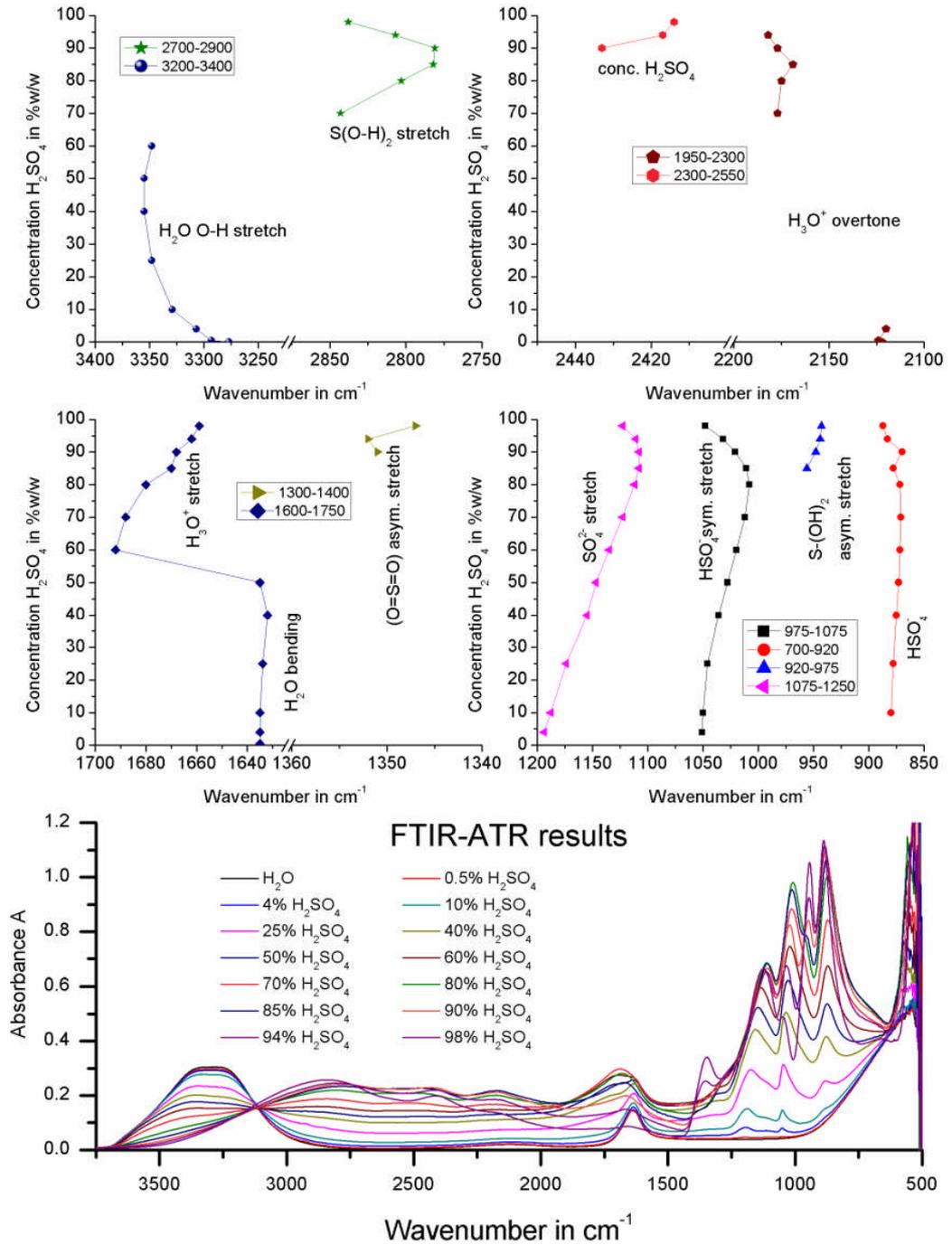
Figure 1: FTIR-ATR peak position of aqueous H<sub>2</sub>SO<sub>4</sub> of various concentrations.
