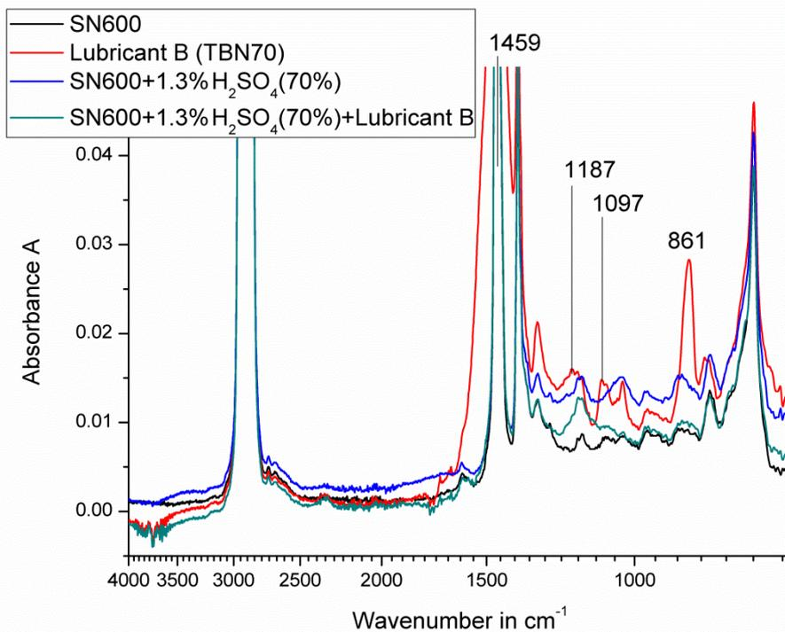
**Figure 7.23: FTIR-ATR spectra of SN600+1.3%v/v70%w/wH<sub>2</sub>SO<sub>4</sub> and a fully formulated “lubricant B” with a alkaline reserve of 70 mgKOH/g. Fresh and sampled during the friction test at 170 °C. Test no. 19.**
