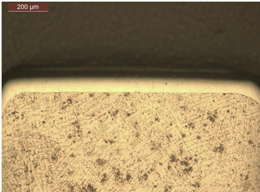
**Figure 6.6: Chrome coating and base material of a automotive piston ring as used in this study**
