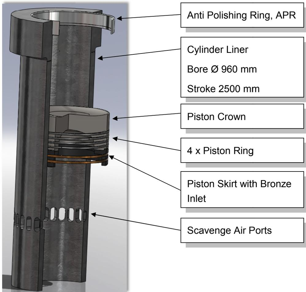
**Figure 1.6: Parts directly involved in piston running, sketched after the Wärtsilä RT96 engine type**
