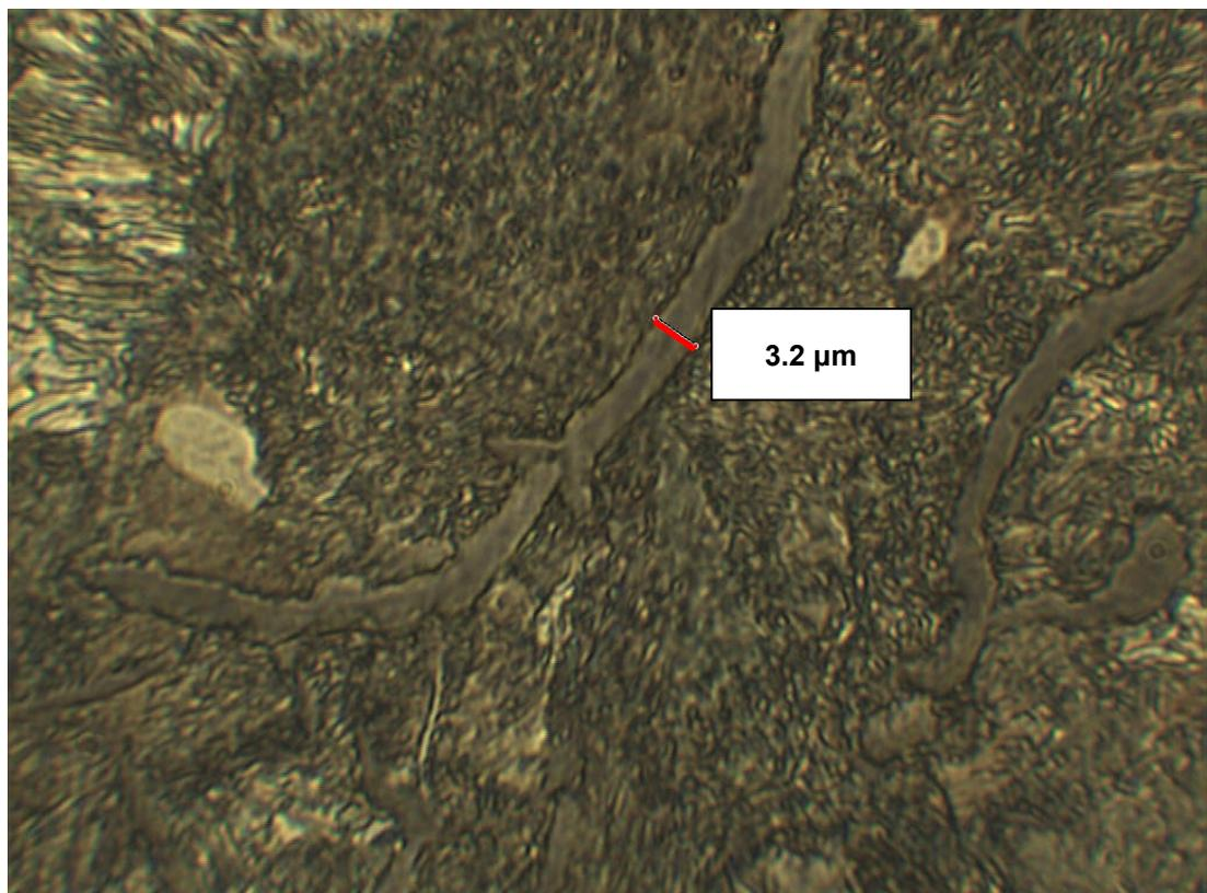
**Figure 6.4: Graphite lamella of a grey cast iron automotive cylinder liner as used in this study**
