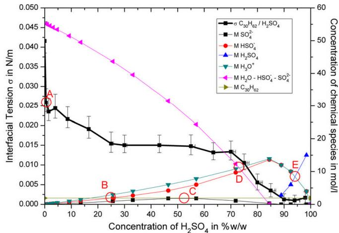
Fig. 2. Results of interfacial tension measurements between squalane and sulphuric acid ( $\sigma_{\text{C}_{30}\text{H}_{62}/\text{H}_2\text{SO}_4}$ ) at 21 °C in comparison to molecular concentration of species in the acid phase, according to [7].
