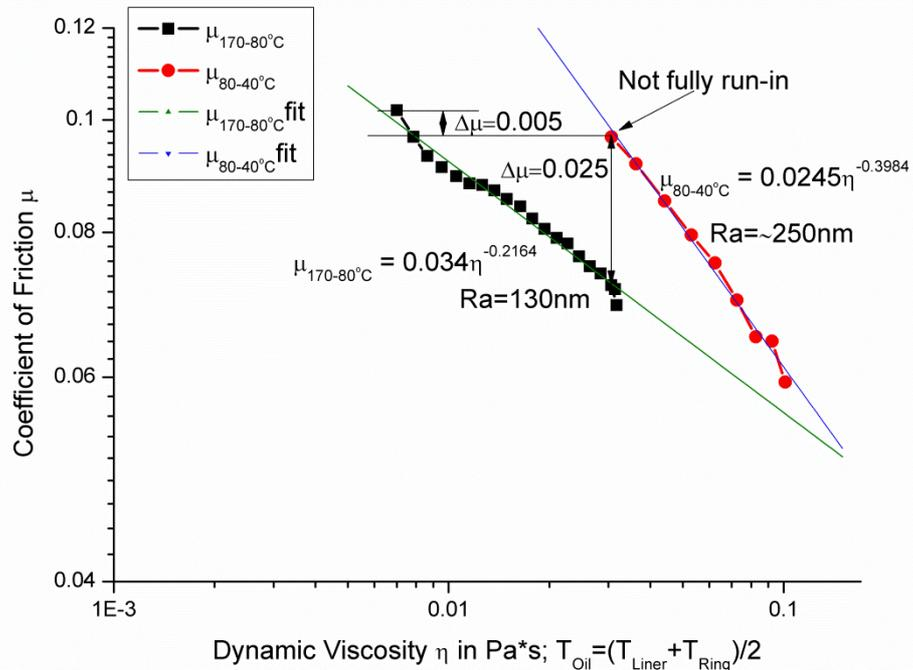
**Figure 7.2: Influence of viscosity on the coefficient of friction, measured by dropping the temperature on two run-in surfaces with different surface roughness's, lubricated with SN600.**
