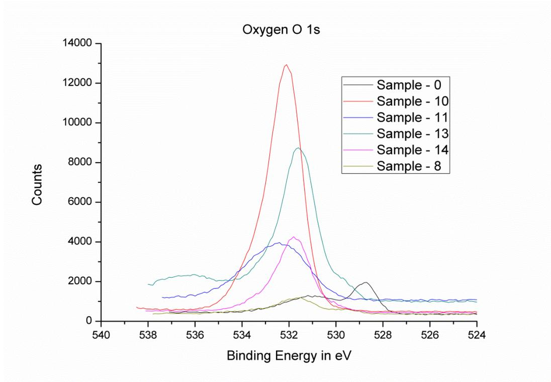
**Figure 7.42: O1s XPS spectra for all cylinder liner wear scars**
