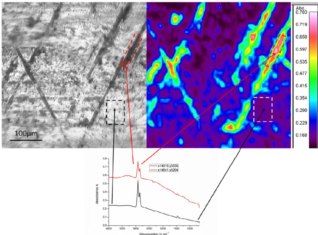
**Figure 6.36: Typical result from a FTIR-microscope area scan. Comparison of visual stitched image, absorbance map and averaged spectra**
