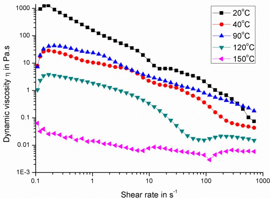
**Figure 3.34: Viscosity of bitumen formed between HVI160B and 98 %w/w  $H_2SO_4$ . See text for encountered difficulties**
