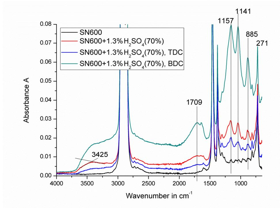
**Figure 16:** FTIR-ATR spectra of SN600+1.3 %v/v 70 %w/w H<sub>2</sub>SO<sub>4</sub>, fresh and sampled during the friction test at 80 °C
