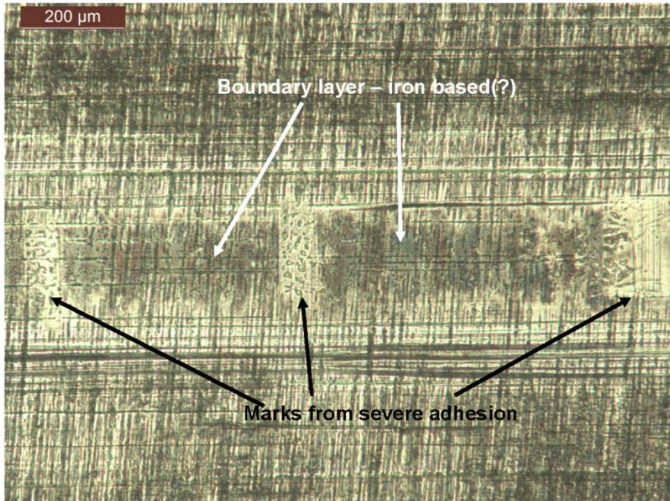
Figure 10: Piston ring wear scar, lubricated with SN600 at 80 °C for 6.5 hours
