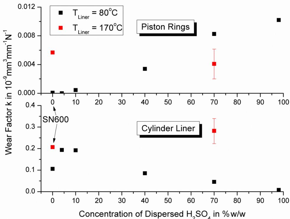
**Figure 7.45: Wear factor  $k$  of piston ring and cylinder liner over various concentrations of H<sub>2</sub>SO<sub>4</sub> at 80 and 170 °C**
