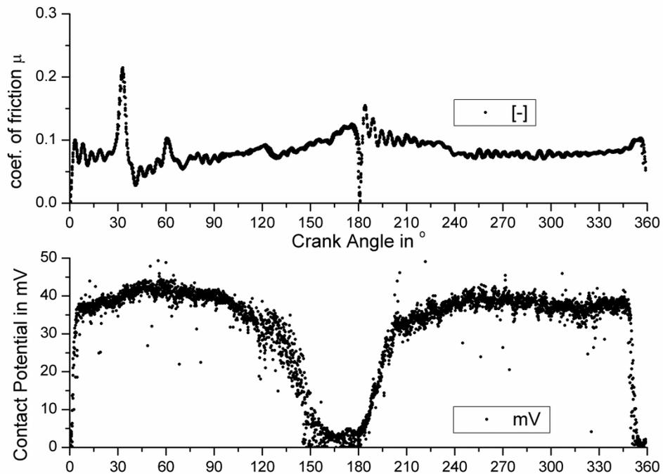
**Figure 6.20: Typical result from the evaluated force transducer signal and the Lunn-Furey contact potential difference over the crank angle**
