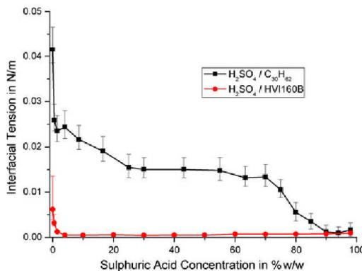
Fig. 2 Interfacial tension of H<sub>2</sub>SO<sub>4</sub> to squalane and API Group I base oil HV1160B at 22 °C after heating to 90 °C
