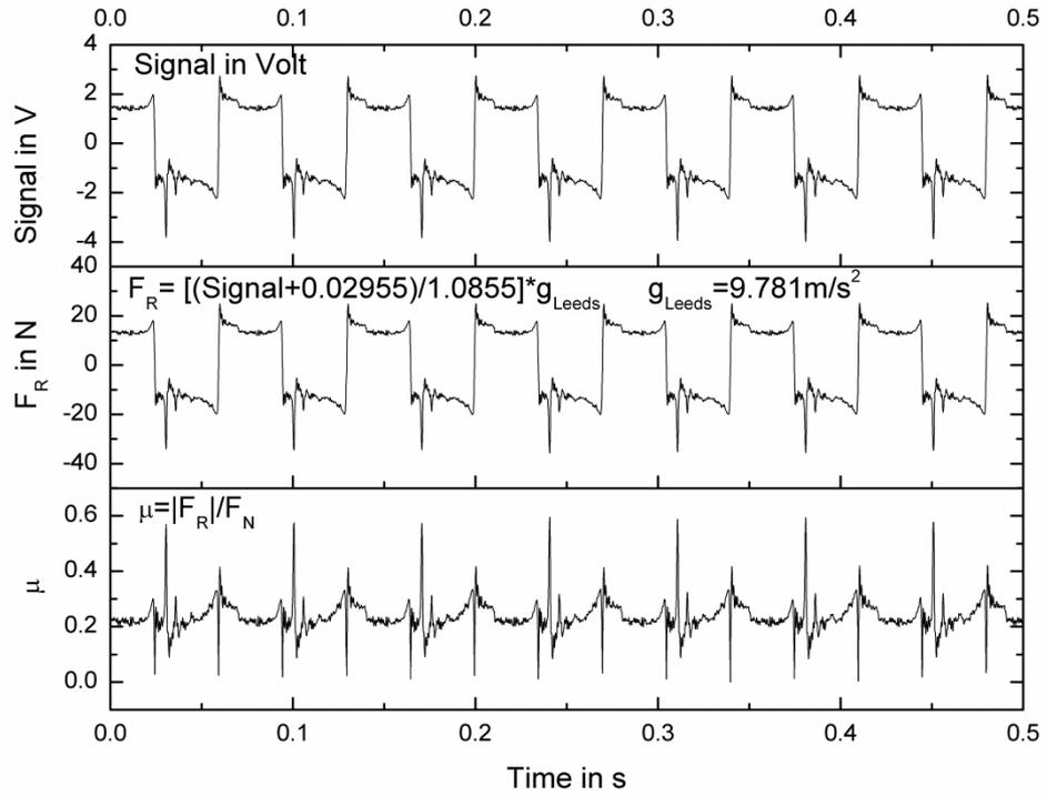
**Figure 6.18: Evaluation of force transducer volt signal into a friction coefficient**
