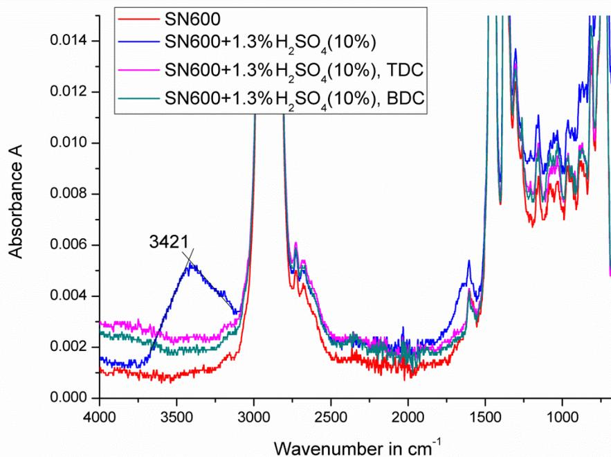
**Figure 7.19: FTIR-ATR spectra of SN600+1.3%v/v10%w/w $\text{H}_2\text{SO}_4$ , fresh and sampled during the friction test at 80 °C. Test no. 5.**
