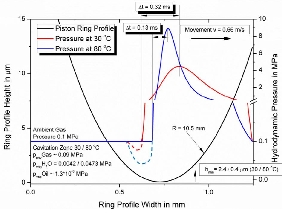
**Figure 7.18: Hydrodynamic pressure distribution below a moving piston ring profile at 30 and 80 °C with an applied load of 30 N.**
