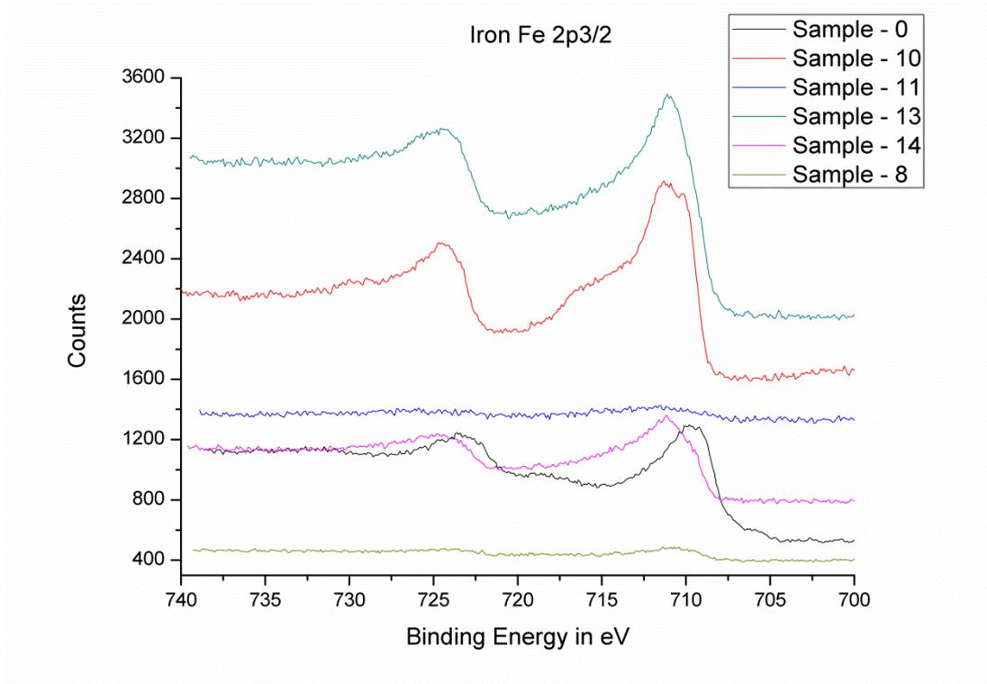
Figure 7.44: Fe<sub>2p<sub>3/2</sub></sub> XPS spectra for all cylinder liner wear scars
