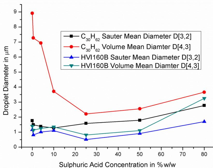
**Figure 3.20: Statistic evaluation of the droplet size distribution for dispersed  $H_2SO_4$  in  $C_{30}H_{62}$  and HVI160B; volume and surface rated.**
