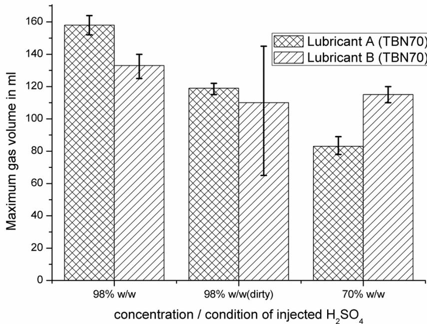
**Figure 3.28: Final CO<sub>2</sub> gas volume at the end of the test.**
