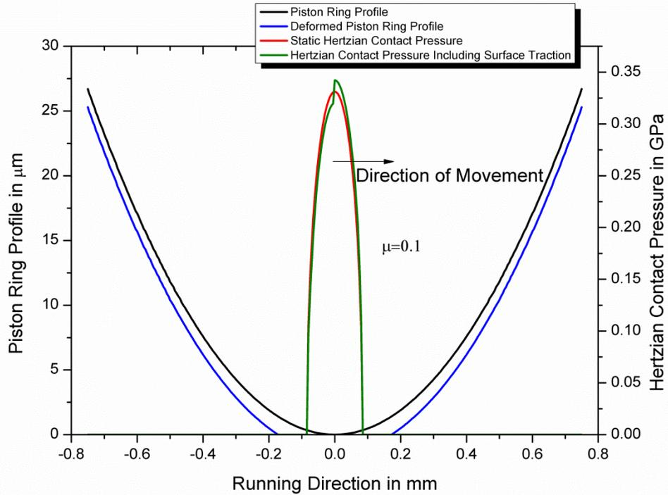
**Figure 6.31: Side view of Figure 6.30 at the centre of the contact. Hertzian contact pressure in unworn condition on the TE77 test bed in static and moving condition**
