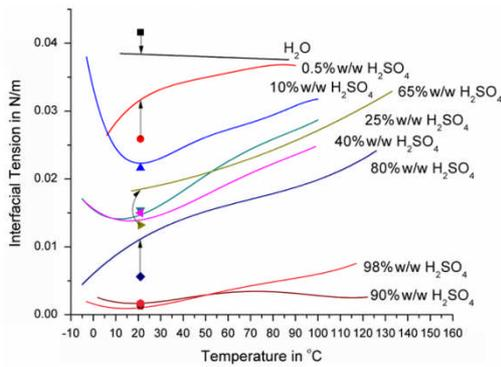
Fig. 4. Concentration and temperature dependency of the interfacial tension between sulphuric acid,  $H_2SO_4$ , and squalane,  $C_{30}H_{62}$ . The values from Fig. 2 are added for comparison.
