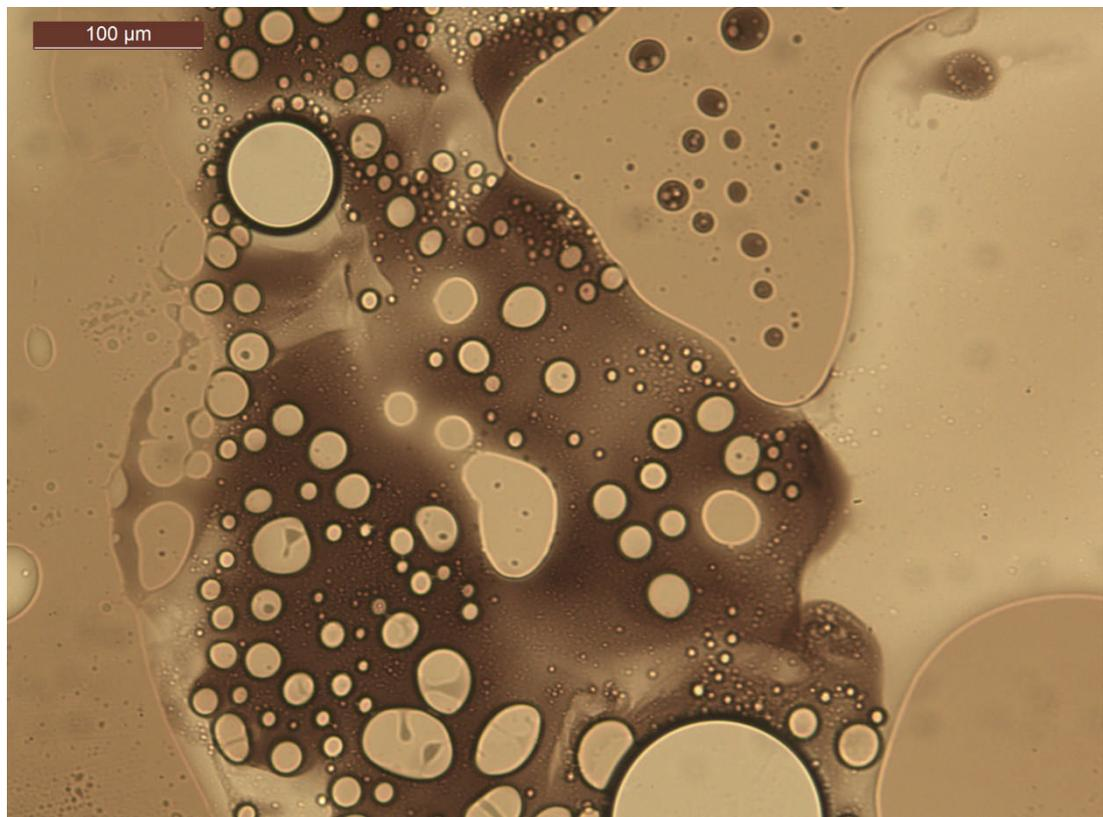
**Figure 3.6: Microscopic view on bituminous matter formed between 98 %w/w H<sub>2</sub>SO<sub>4</sub> and HVI160B before separating from oil phase. 100x**
