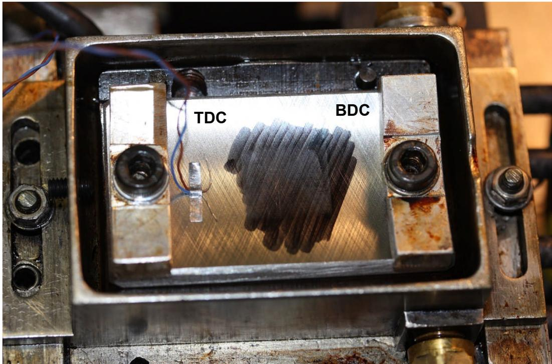
**Figure 6.10: Cylinder liner sample with spot welded K-type thermocouple after the alignment check**
