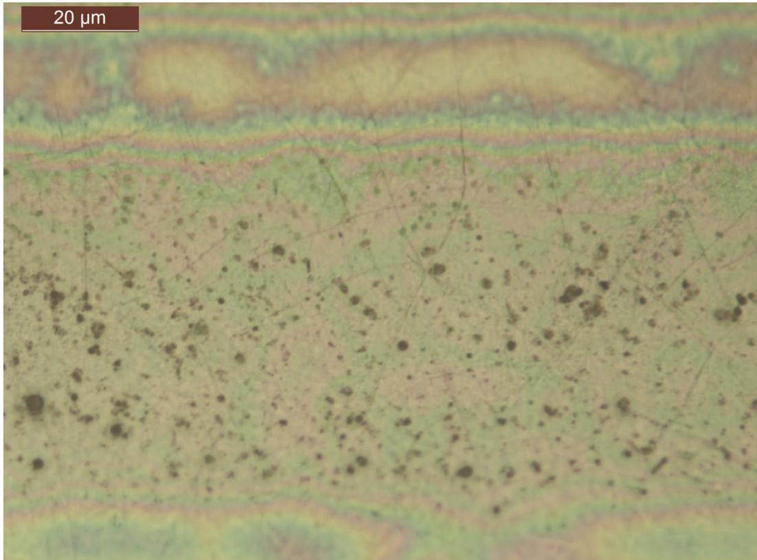
**Figure 7.14: Piston ring wear scar, test 12, lubricated with SN600 + 70 %w/w H<sub>2</sub>SO<sub>4</sub> at 170 °C**
