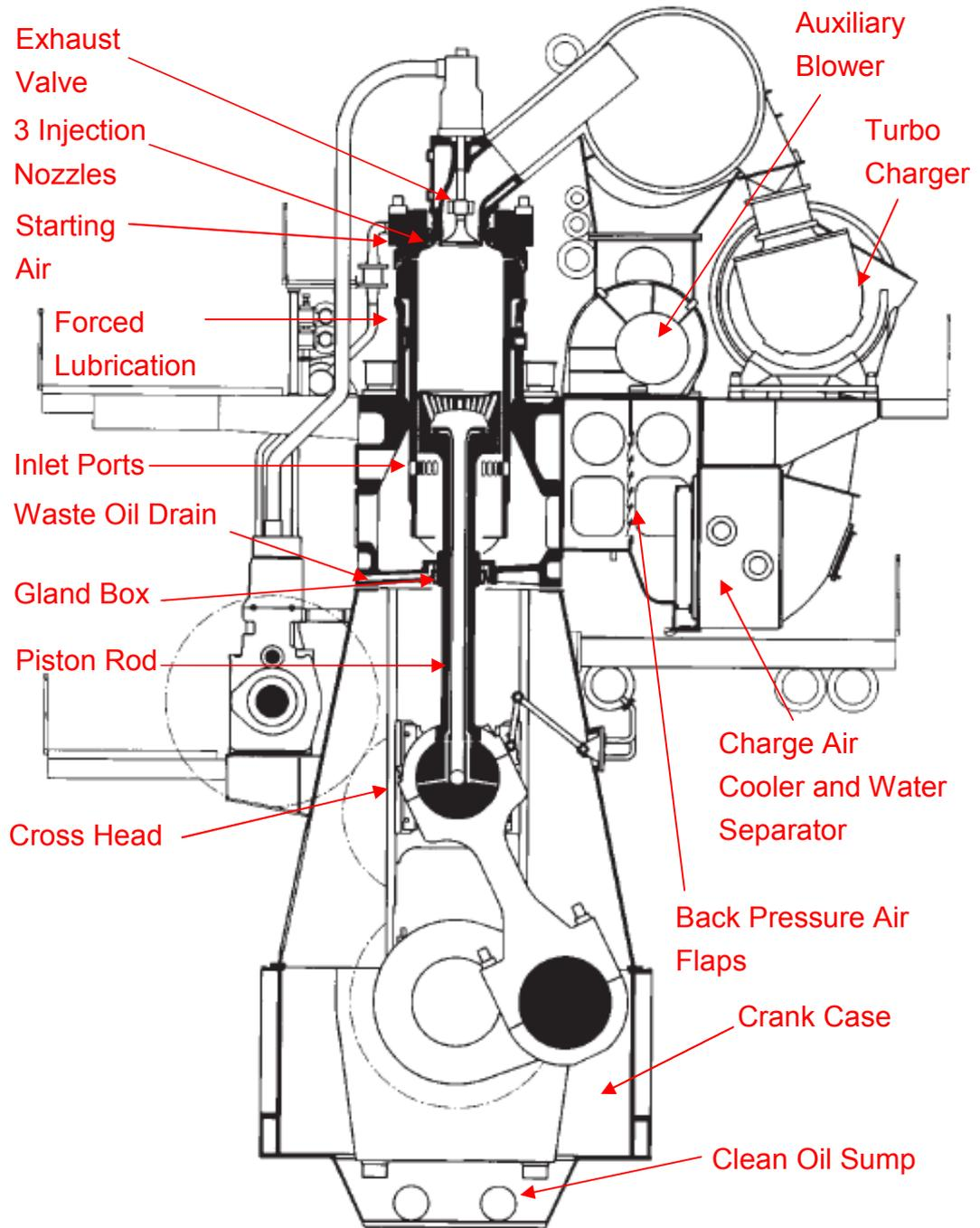
**Figure 1.2: Cross-section of a modern large bore 2-stroke low speed Diesel engine, the Wärtsilä RTA96C (Woodyard, 2004)**
