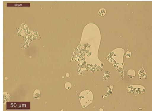
**Fig. 16** Microscopic view on bituminous matter formed between 80 %w/w H<sub>2</sub>SO<sub>4</sub> and HVI160B. Magnification: ×200
