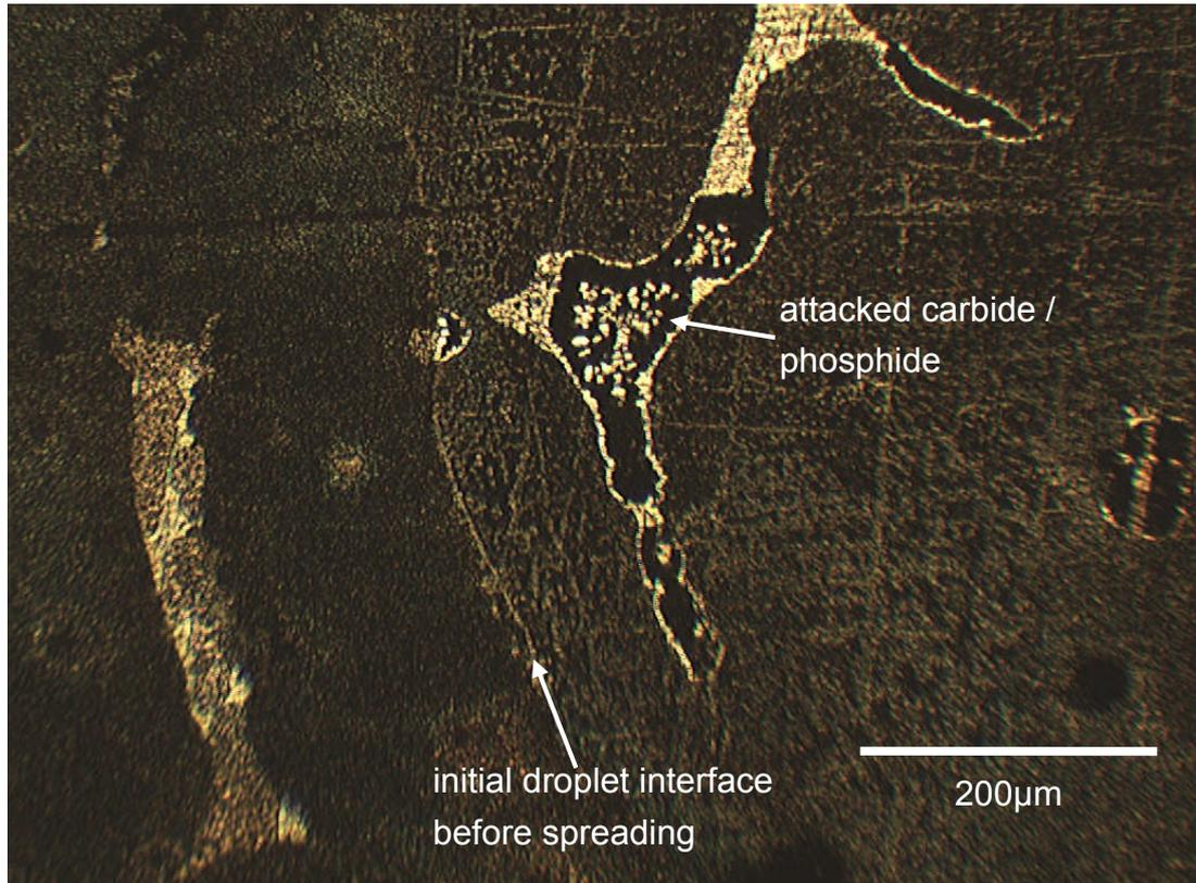
**Figure 5.10: Corrosive attack on grey cast iron after contact angle measurements with 65 %w/w H<sub>2</sub>SO<sub>4</sub> at 145 °C**
