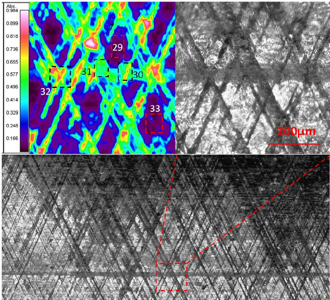
**Figure 7.36: FTIR-scan and visual image on sample 21 in midstroke**
