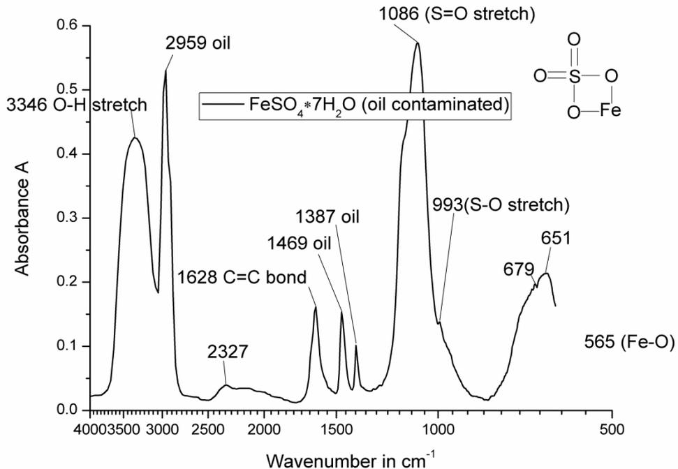
**Figure 6.37: FTIR-spectrum of ferrous sulphate,  $\text{FeSO}_4 \cdot 7\text{H}_2\text{O}$ , in oil (NIST, 2011), a compound suggested by the XPS results**
