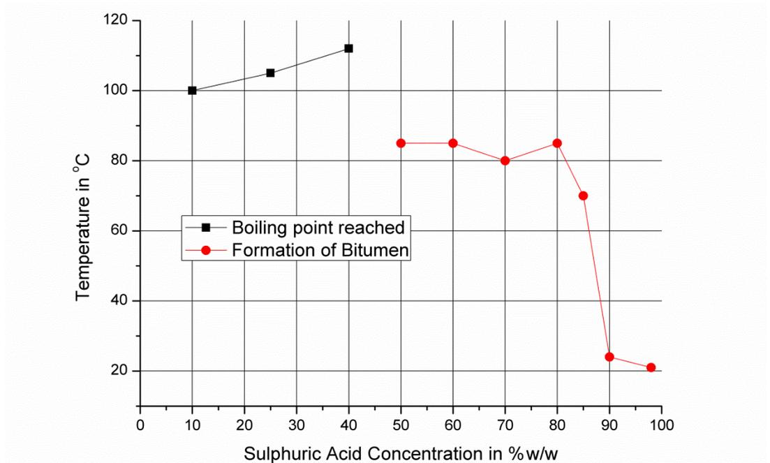
Figure 3.38: Fast heating of API Group I base oil HVI160B in contact with various concentrations of aqueous  $H_2SO_4$  until bitumen is formed.
