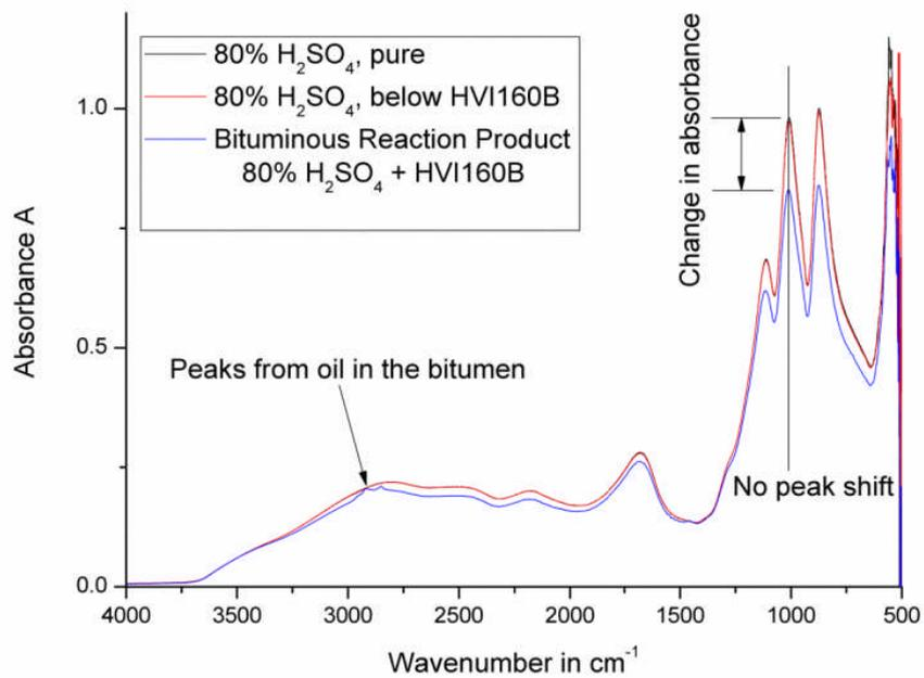
Figure 3: FTIR-ATR absorbance spectra of pure  $80\% H_2SO_4$ , remaining acid used in the reaction and the reaction product
