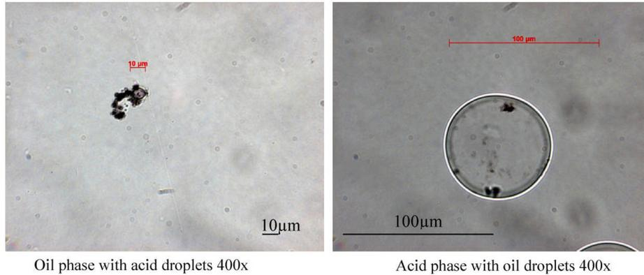
Fig. 6. Transmission microscopic image of the oil and acid phase of the mixture 80% w/w  $H_2SO_4$  and  $C_{30}H_{62}$  after exposure to 165 °C.
