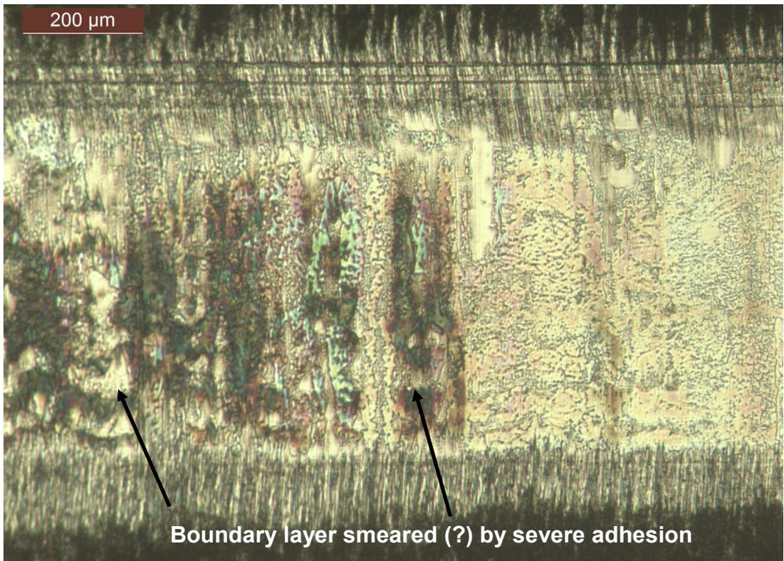
**Figure 7.15: Piston ring wear scar, test 18, lubricant B & SN600 + 70 %w/w H<sub>2</sub>SO<sub>4</sub> at 170 °C. Test finished after an 53 minute period of adding lubricant B.**
