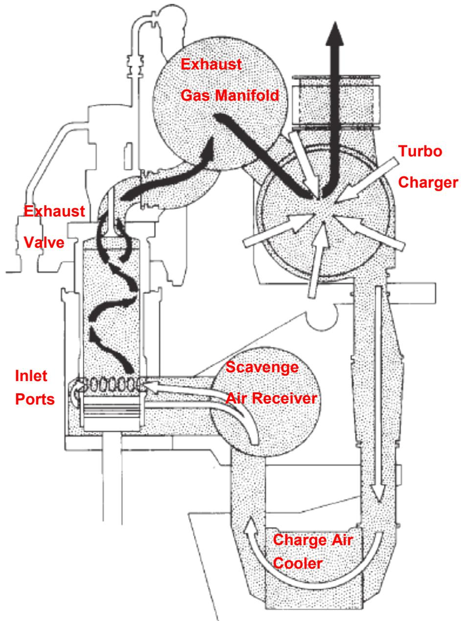
Figure 1.3: B&W uniflow scavenging system (Woodyard, 2004)
