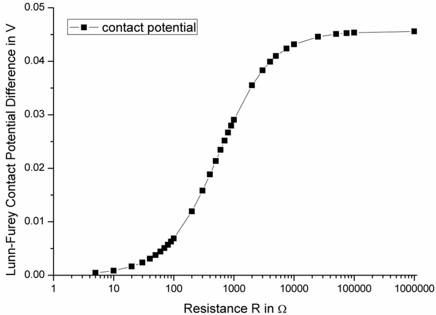
**Figure 6.12: Lunn-Furey contact potential difference versus applied electrical resistance**
