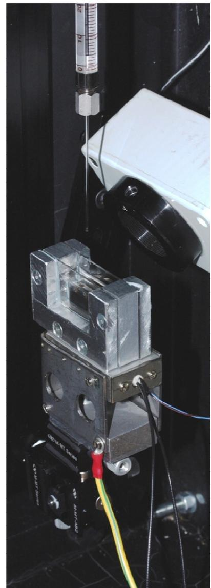
**Figure 5.1: Experimental arrangement of the contact angle measurements**
