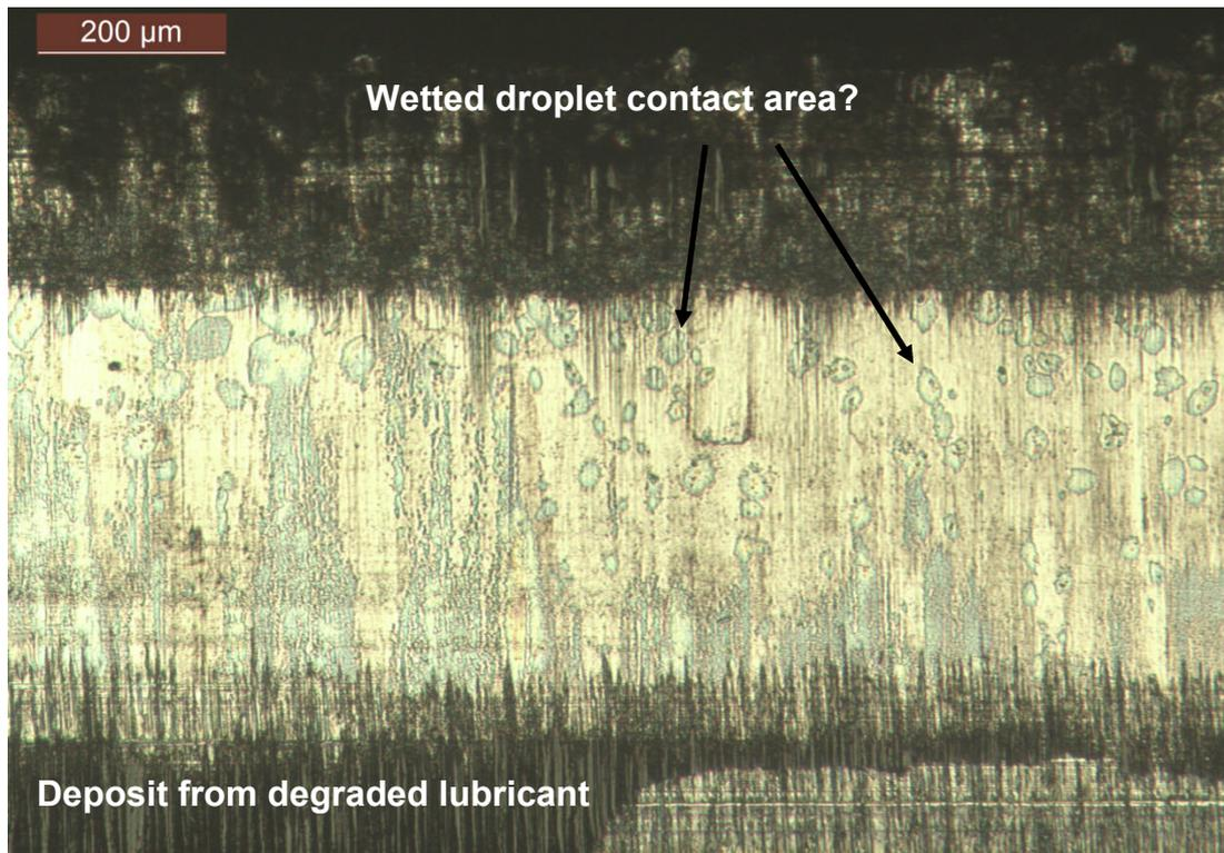
**Figure 7.16: Piston ring wear scar, test 19, lubricant B & SN600 + 70 %w/w H<sub>2</sub>SO<sub>4</sub> at 170 °C. Test finished after an 8 minute period of adding lubricant B.**
