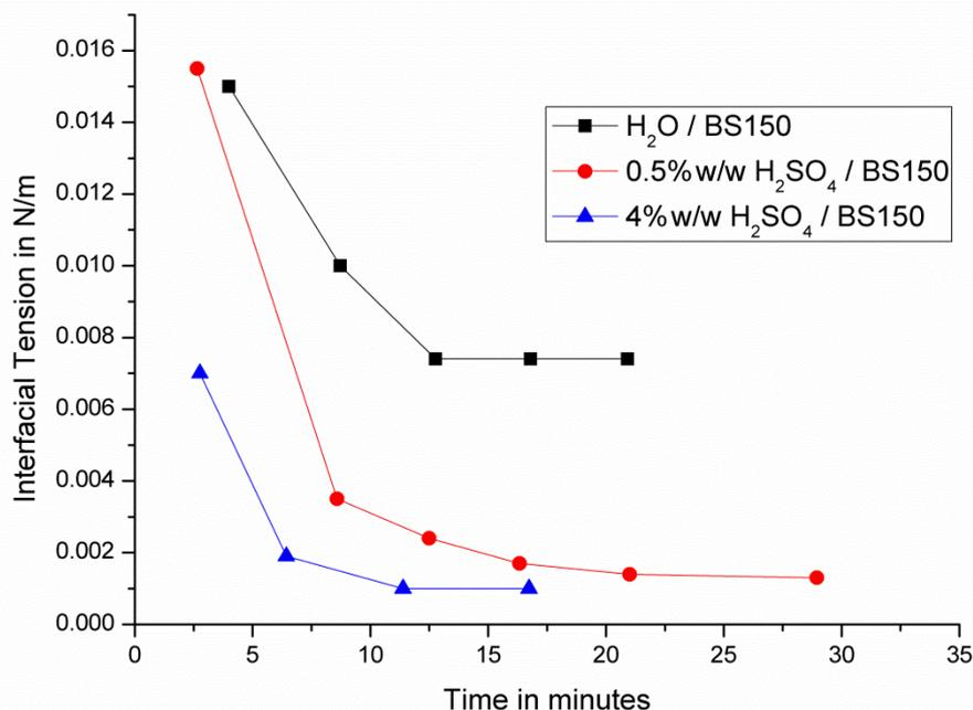
**Figure 4.8: Time dependent development of interfacial tension between water (H<sub>2</sub>O), aqueous concentrations (%w/w) of H<sub>2</sub>SO<sub>4</sub> and API Group I base oil BS150 at 22 °C**
