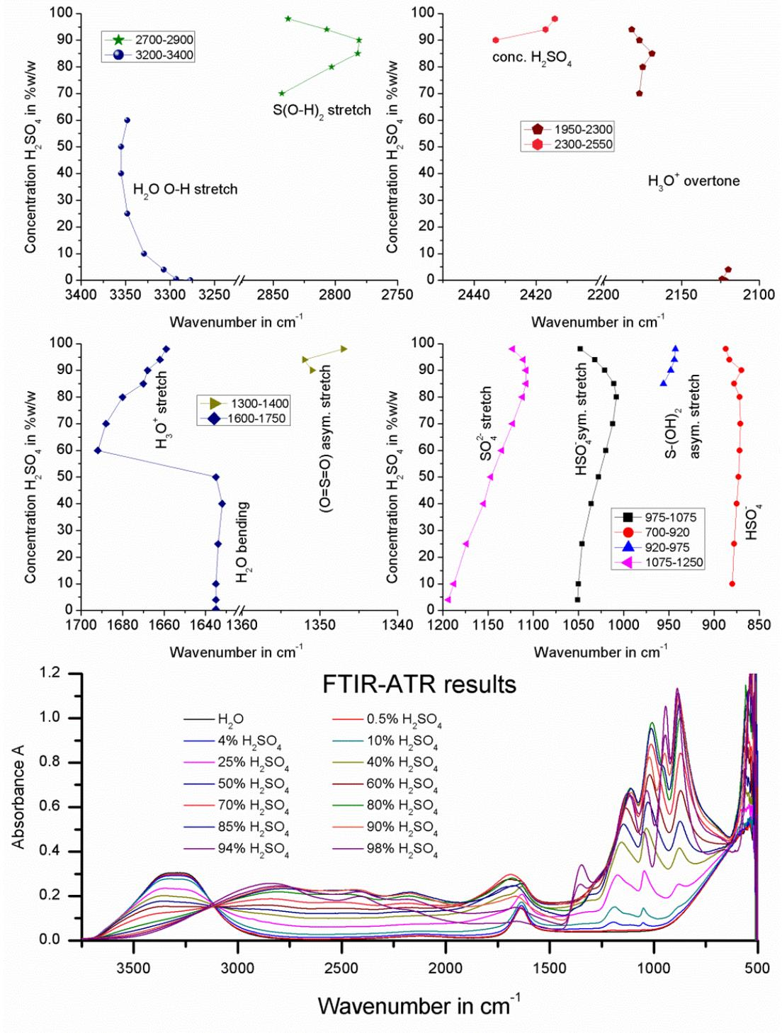
Figure 3.14: FTIR-ATR peak position of aqueous H<sub>2</sub>SO<sub>4</sub> of various concentrations.
