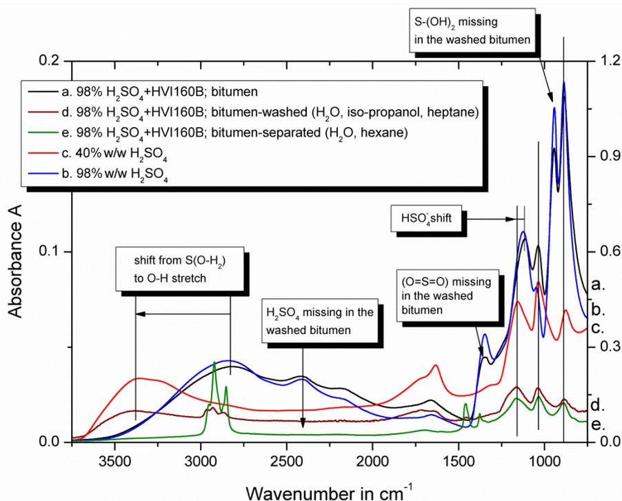
**Figure 3.17: FTIR-ATR absorbance spectra of bituminous reaction product (a.), solvent washed bituminous reaction product (d.), solvent separated bituminous reaction product (e.) and pure 40 %w/w and 98 %w/w H<sub>2</sub>SO<sub>4</sub> (c. and b.).**
