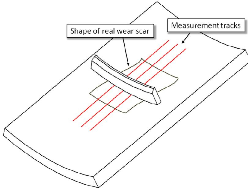
**Figure 6.32: Measurement tracks along the cylinder liner wear scar and across the piston ring profile**
