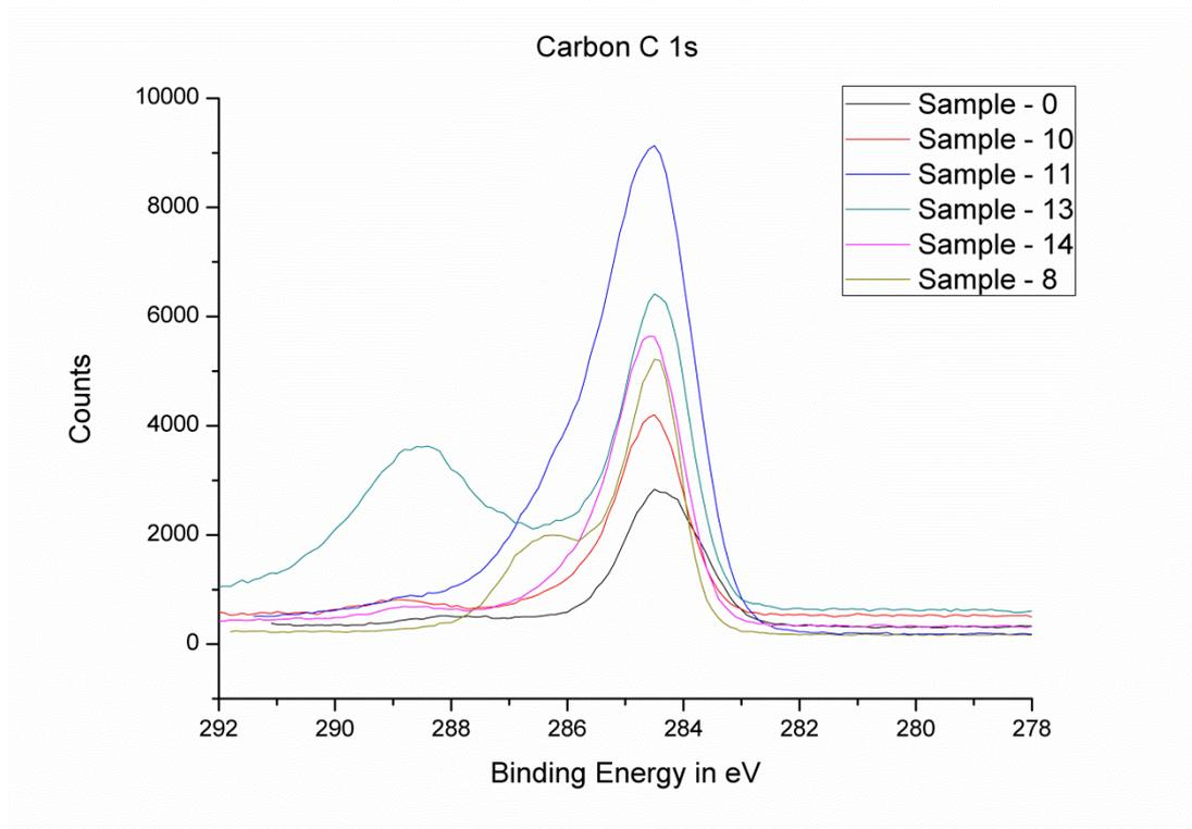
**Figure 7.40: C1s XPS spectra for all cylinder liner wear scars**
