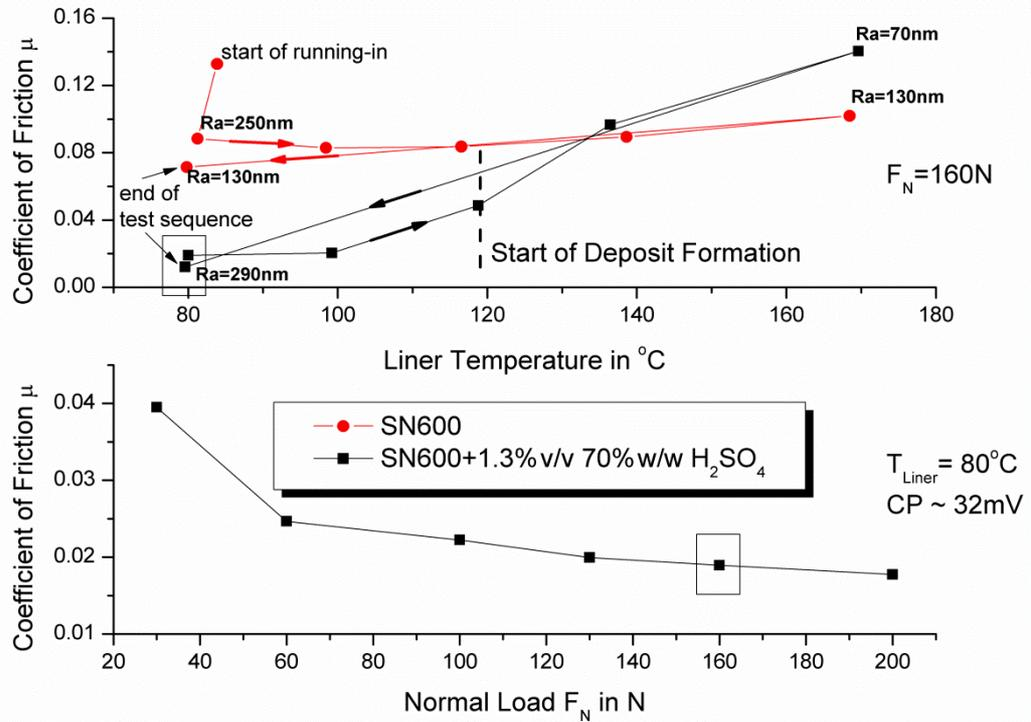
**Figure 7.7: Influence of temperature and load on the coefficient of friction for pure and acid contaminated base oil SN600.**
