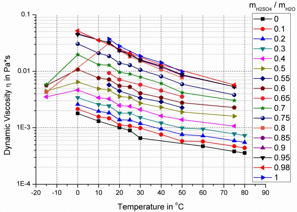
**Figure A.2: Temperature dependent dynamic viscosity,  $\eta$ , for various concentrations of aqueous sulphuric acid (DECHEMA e.V., 2005 - 2008)**
