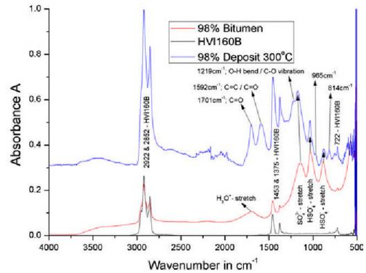
**Fig. 21** FTIR-ATR analysis of deposit formed at 300 °C with bitumen created with 98 %w/w H<sub>2</sub>SO<sub>4</sub>
