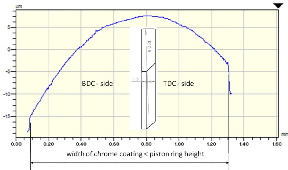
**Figure 6.35: Typical measurement profile across a worn piston ring profile**
