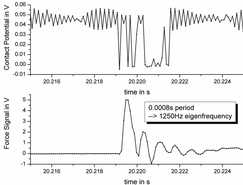
**Figure 6.21: Evaluation of the eigenfrequency of the cylinder liner holder – force transducer arrangement**
