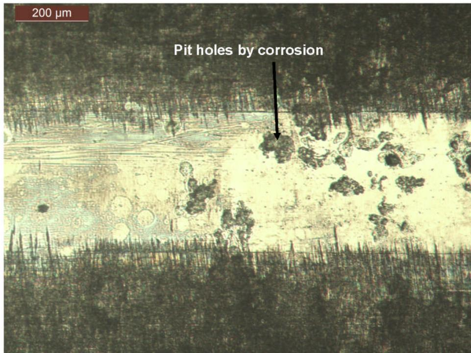
**Figure 12: Piston ring wear scar, lubricated with SN600+70%/w/w H<sub>2</sub>SO<sub>4</sub> at 80 °C for 6.5 hours**
