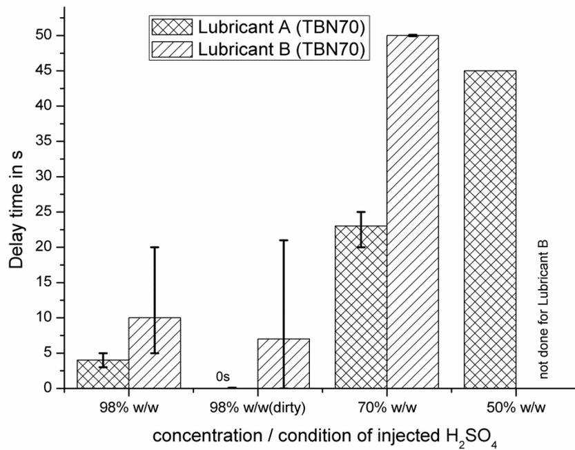
Figure 3.27: Delay time between injection of H<sub>2</sub>SO<sub>4</sub> and CO<sub>2</sub> gas release
