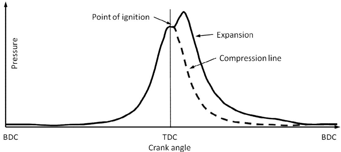
**Figure 1.5: Typical indicator diagram of the pressure in the combustion chamber drawn over crank angle (Woodyard, 2004)**
