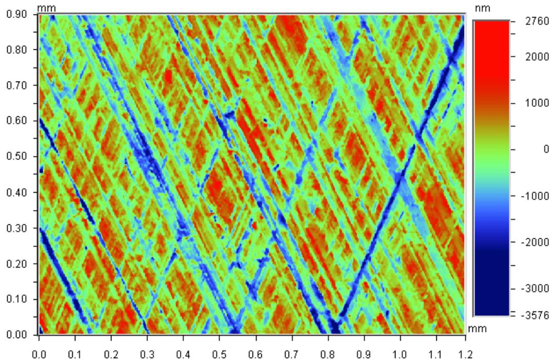
**Figure 8.7: Surface topography of a honed automotive cylinder liner.**
