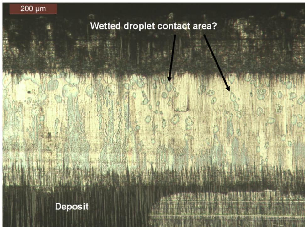
Figure 15: Piston ring wear scar, lubricated with lubricant B & SN600 + 70 %w/w H<sub>2</sub>SO<sub>4</sub> at 170 °C. The test finished after an 8 minute period of adding lubricant B.
