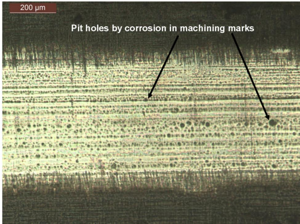
**Figure 13: Piston ring wear scar, lubricated with SN600+70%w/w H<sub>2</sub>SO<sub>4</sub> at 170 °C for 6.5 hours**
