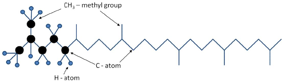
**Figure 4.1: Chemical structure of squalane (C<sub>30</sub>H<sub>62</sub>), for ease of understanding in a mixed, model and skeletal form (Enevoldsen, et al., 2007).**
