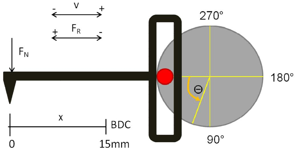
Figure 6.16: Definition of directions in the TE77 friction testing machine
