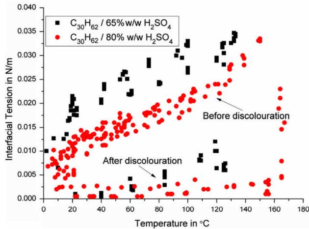
Fig. 3. Temperature dependent interfacial tension of 65% and 80%  $H_2SO_4$  towards  $C_{30}H_{62}$ .
