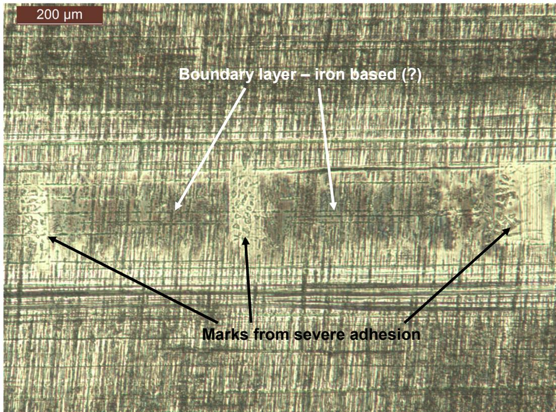
Figure 7.9: Piston ring wear scar, test 8, lubricated with SN600 at 80 °C
