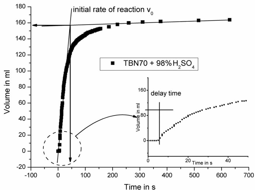
**Figure 3.22: Typical result of CO<sub>2</sub> gas release from TBN70 lubricant**
