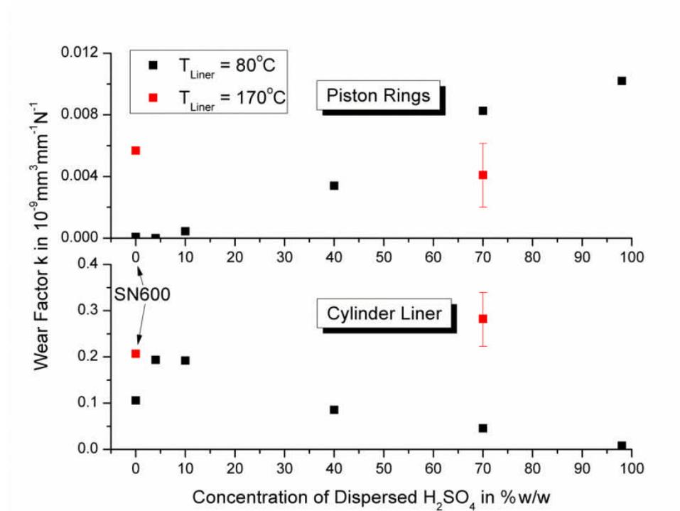
Figure 18: Wear factor k of piston ring and cylinder liner over various concentrations of H<sub>2</sub>SO<sub>4</sub> at 80 and 170 °C
