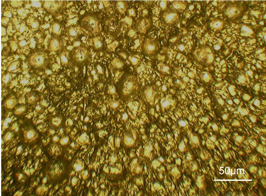
**Figure 3.8: 200x magnification of a solid reaction product created between 80%w/w  $H_2SO_4$  and  $C_{30}H_{62}$  at 165 °C**
