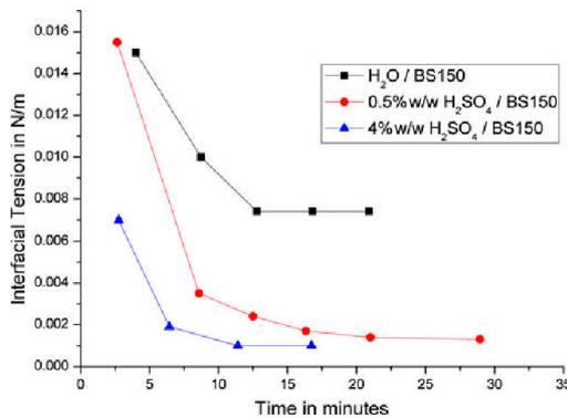
Fig. 1 Time-dependent drop of interfacial tension between API Group I base oil BS150 and water and aqueous H<sub>2</sub>SO<sub>4</sub> at 22 °C
