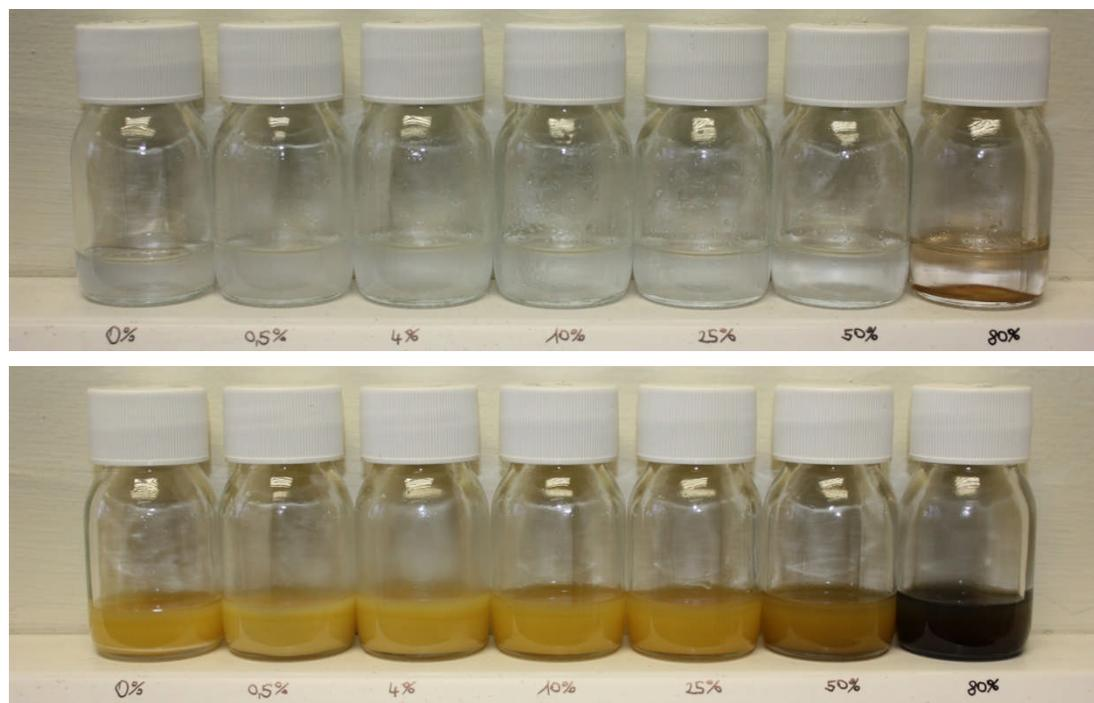
**Figure 3.21: 1.3%v/v aqueous H<sub>2</sub>SO<sub>4</sub> dispersed in C<sub>30</sub>H<sub>62</sub> (upper) and HVI160B (lower) after 72 hours of settling. From left: 0, 0.5, 4, 10, 25, 50 & 80 %w/w**
