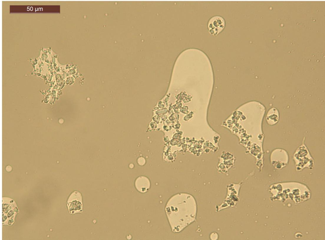
**Figure 3.5: Microscopic view on bituminous matter formed between 80 %w/w H<sub>2</sub>SO<sub>4</sub> and HVI160B, after viscosity measurements. 200x**
