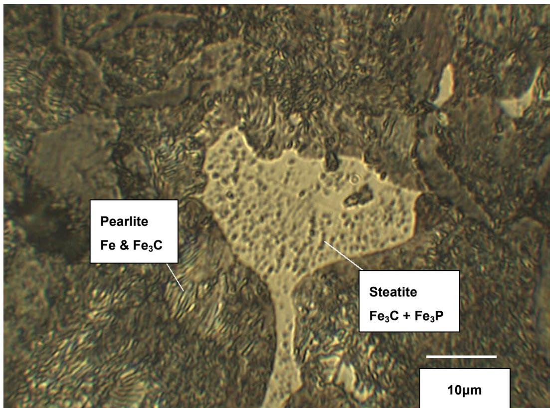
Figure 6.2: Hard phase of a grey cast iron automotive cylinder liner as used in this study
