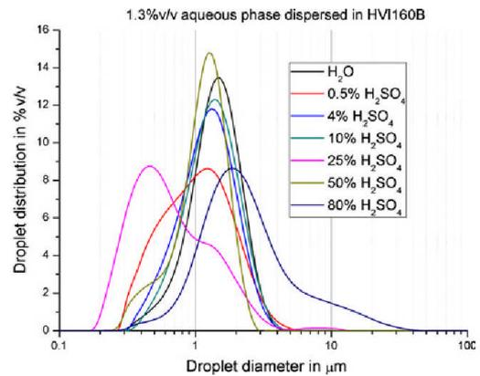
**Fig. 5** Droplet size distribution of 1.3 %v/v aqueous H<sub>2</sub>SO<sub>4</sub> dispersed in API Group I base oil HVI160B
