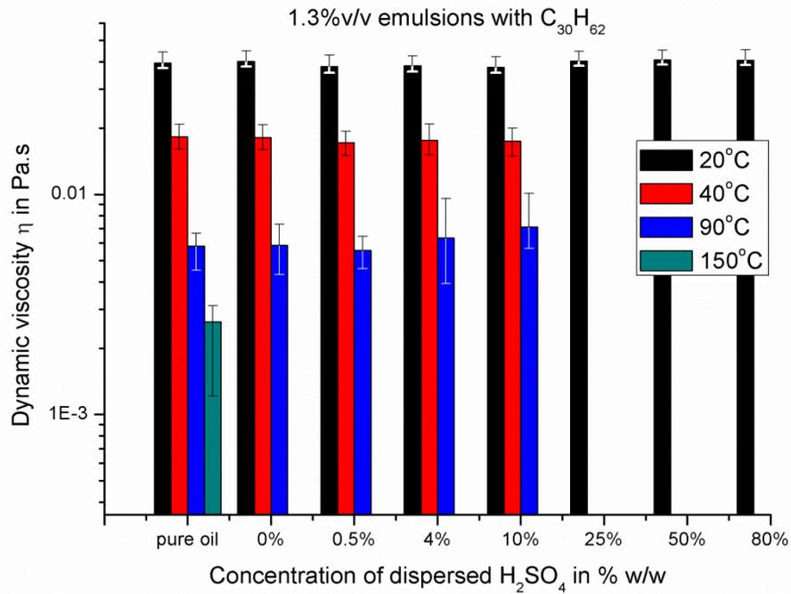
Figure 3.32: Viscosity of pure and emulsified  $C_{30}H_{62}$  with 1.3 %v/v aqueous  $H_2SO_4$  as dispersed phase. Applied shear rate was 200 – 700  $s^{-1}$
