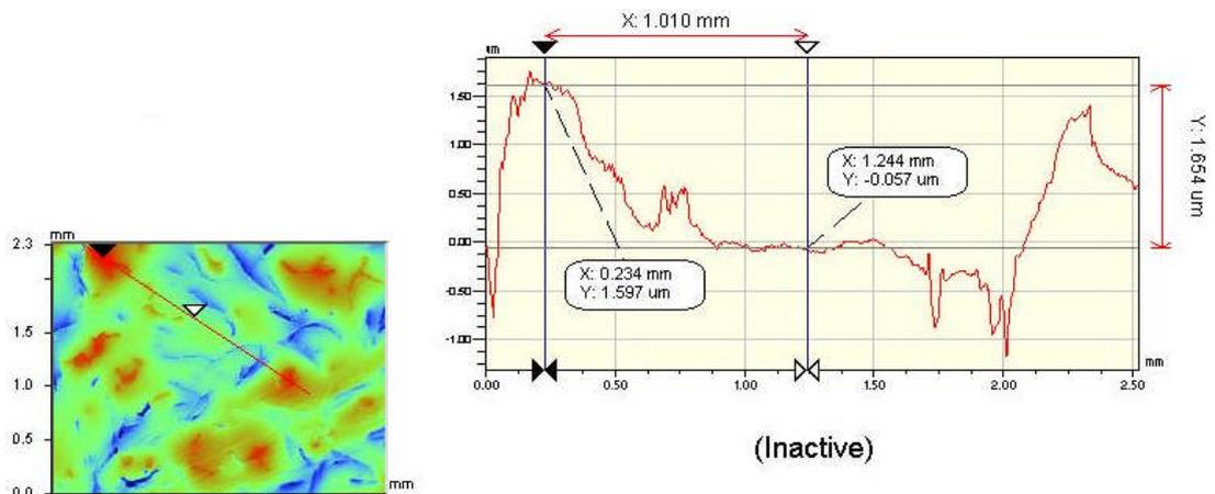
Figure 8.3: Distance between embossed hard phase and pearlitic matrix at 300 °C
