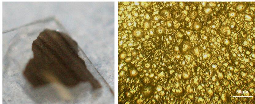
Fig. 7. Solid reaction product after separation, left an overview of the approximately 2 mm × 3 mm flake, right a 200 × microscopic image of the same flake.
