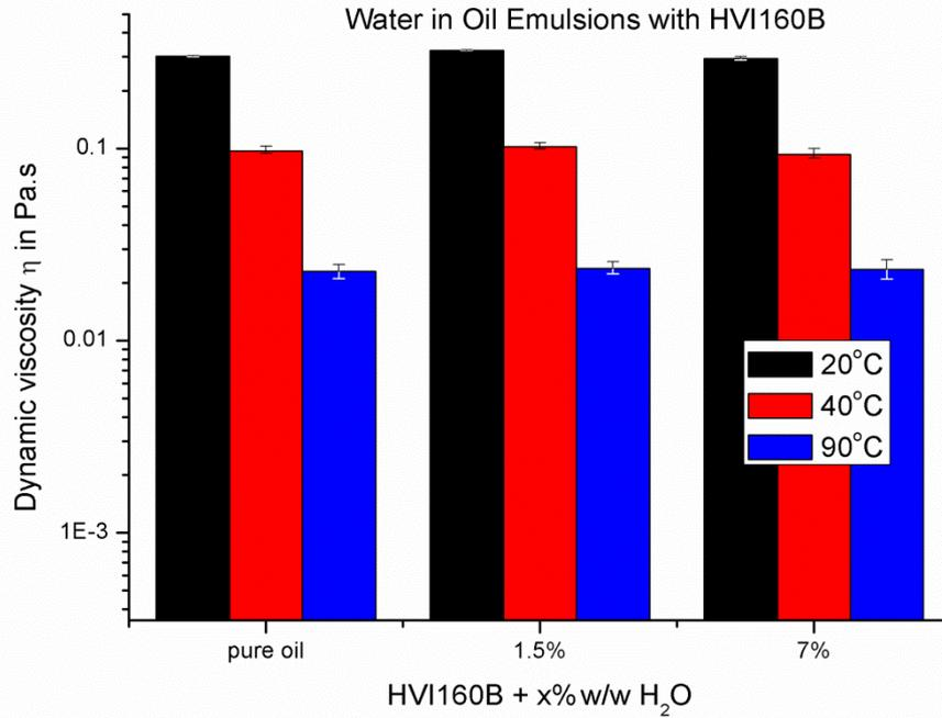
**Figure 3.30: Viscosity of pure and emulsified API Group I base oil HVI160B with water as dispersed phase. Applied shear rate was 200 – 700 s<sup>-1</sup>**
