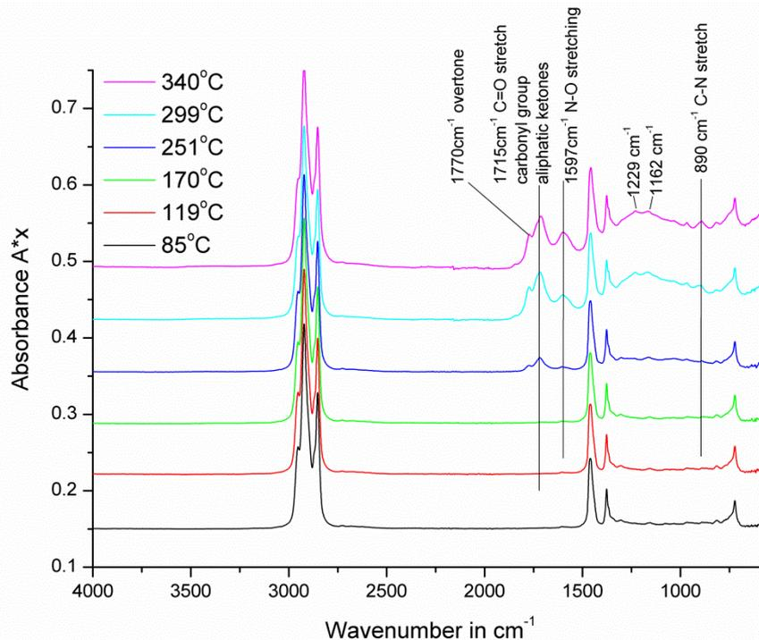
**Figure 7.24: FTIR-ATR spectra of SN600 exposed to various cylinder liner temperatures during the friction tests at 85 – 340 °C, revealing the start of lubricant oxidation at 250 °C and nitration at 300 °C combined with the excessive formation of deposit.**
