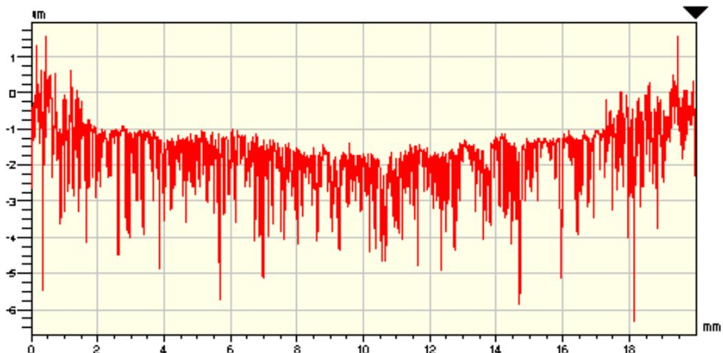
**Figure 6.34: Typical measurement profile along the wear scar on a cylinder liner**
