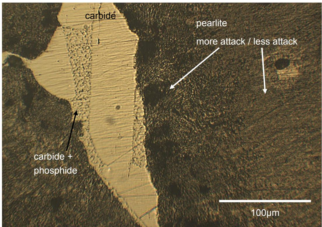
**Figure 5.9: Corrosive attack on grey cast iron after contact angle measurements with 65 %w/w H<sub>2</sub>SO<sub>4</sub> at 20 °C**
