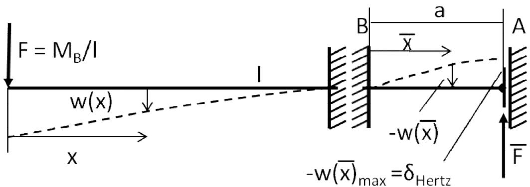
Figure 6.28: Second approach to piston ring deformation with Hertzian contact pressure.
