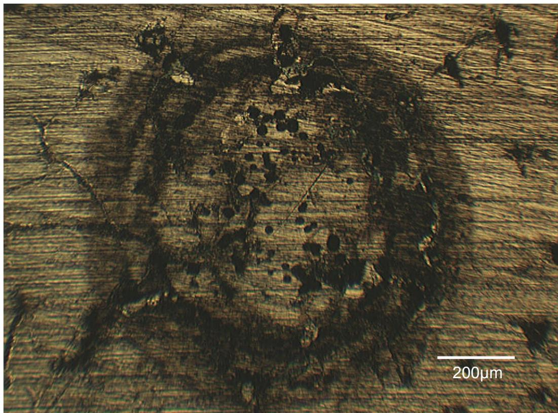
**Figure 5.7: Corrosive attack on grey cast iron after contact angle measurements with pure water at 20 °C**
