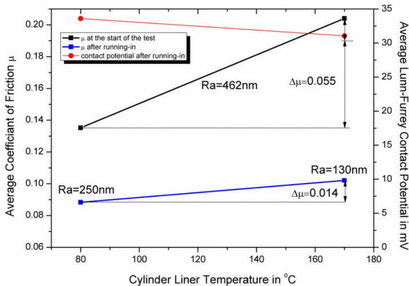
Figure 2: COF before (upper square markers) and after (lower square markers) running-in with SN600 and the corresponding CP measurement after running-in (round markers)
