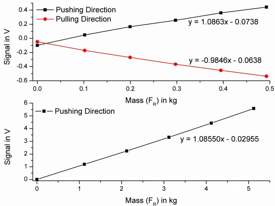
**Figure 6.13: Calibration of TE77 force transducer with known mass**
