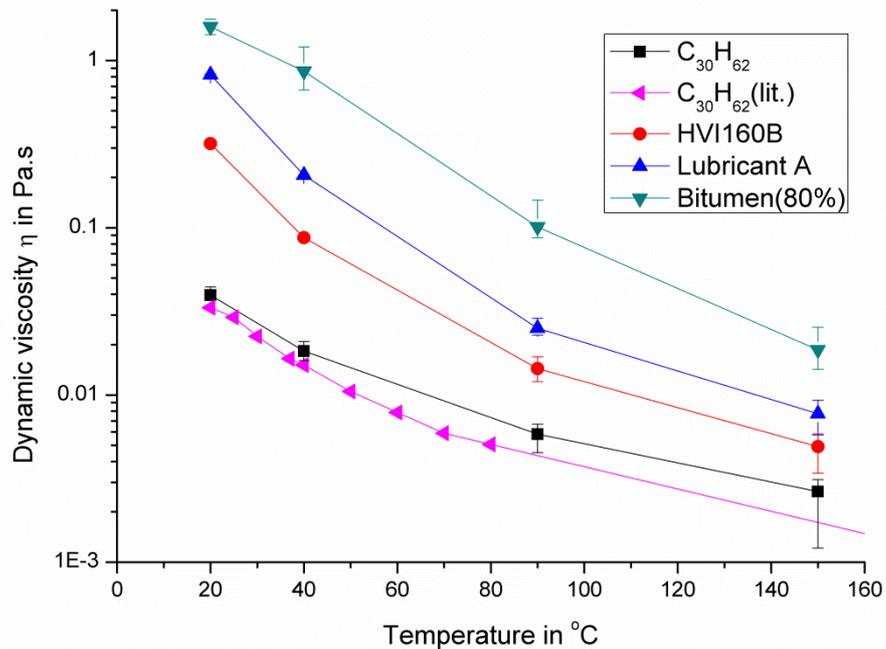
Figure 3.33: Measured viscosity of  $C_{30}H_{62}$  and values found in the literature (DECHEMA e.V., 2005 - 2008), a fully formulated lubricant A, the corresponding base oil HVI160B and the bitumen formed between HVI160B and 80 %w/w  $H_2SO_4$
