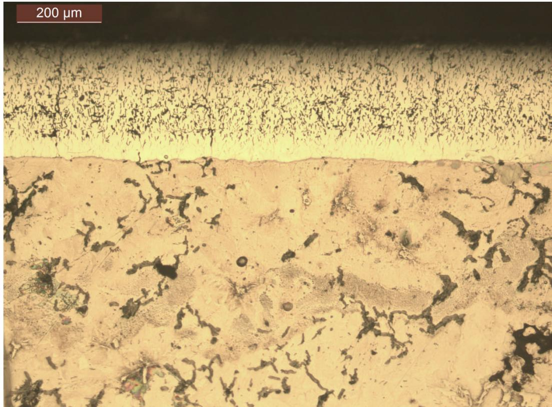
**Figure 6.5: Chrome (CKS) coating and base material of a marine piston ring**
