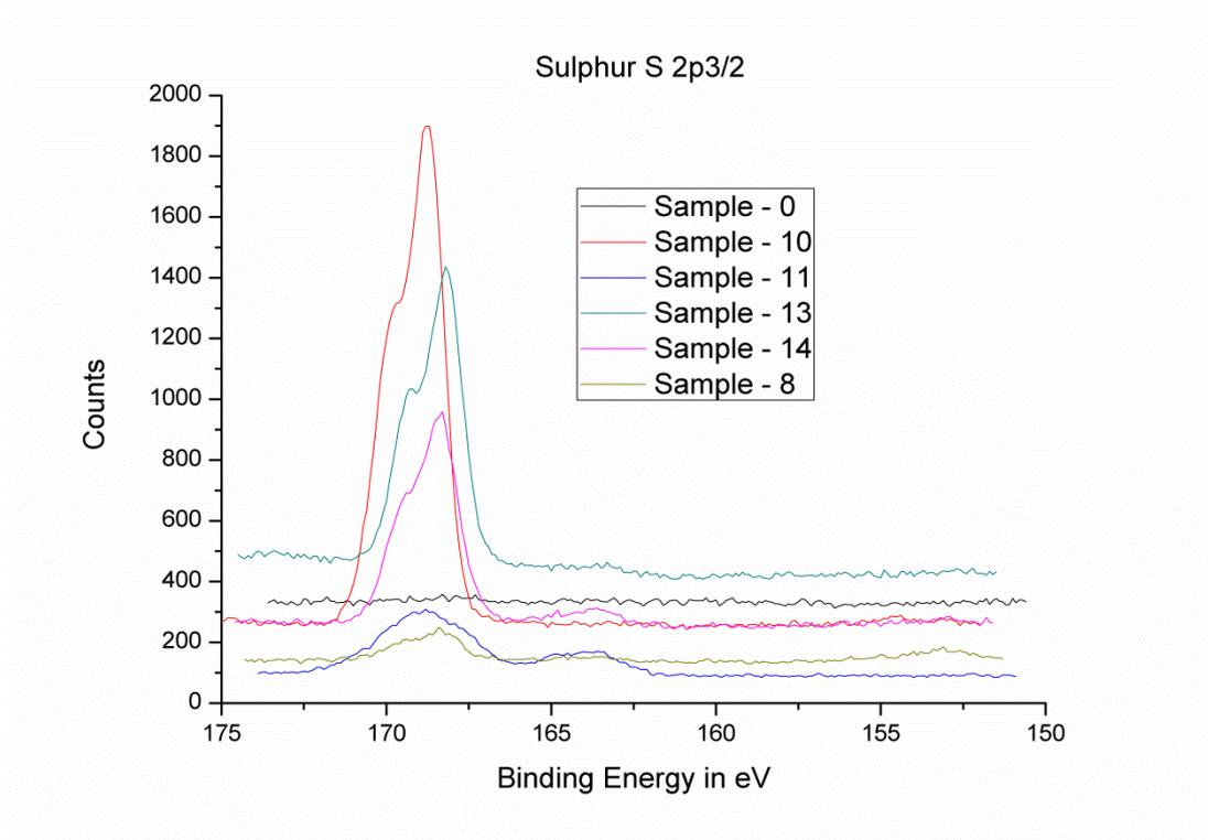
**Figure 7.39: S2p3/2 XPS spectra for all cylinder liner wear scars**
