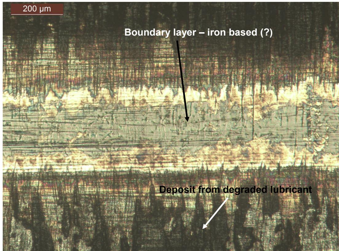
**Figure 7.11: Piston ring wear scar, test 21, lubricated with SN600 from 80 to 340 °C**
