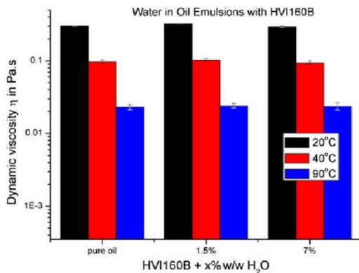
Fig. 7 Viscosity of pure and emulsified API Group I base oil HVI160B with water as dispersed phase. Applied shear rate was 200–700 s<sup>-1</sup>
