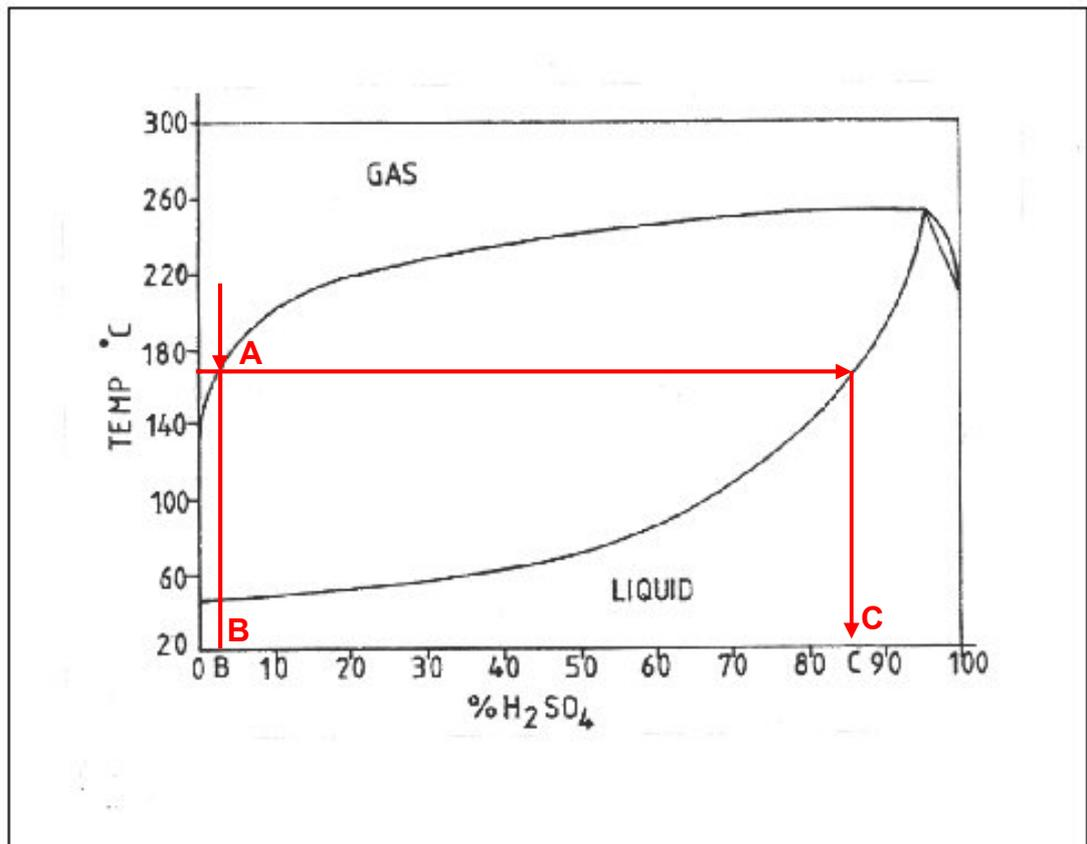
Figure 1.10: The phase diagram for vapour of  $\text{H}_2\text{SO}_4$  and water for a combined partial pressures of  $\sim 0.1$  bar (Land, 1977)
