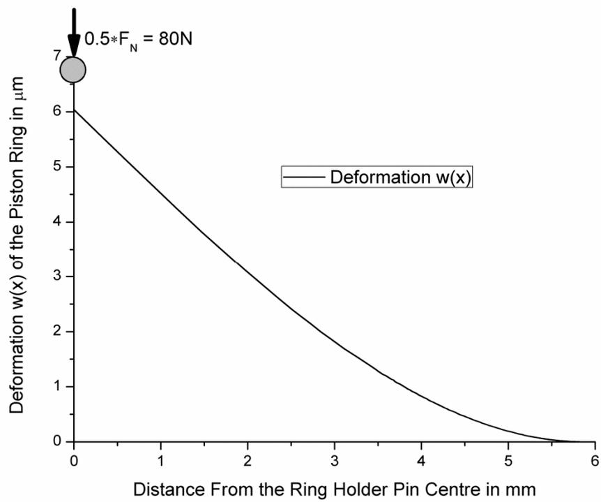
Figure 6.24: Results for deformation  $w(x)$  of the piston ring segment in the TE77 piston ring holder
