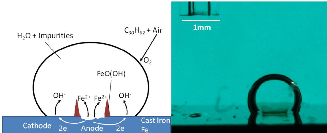
**Figure 5.6: Observation of corrosion on grey cast iron with pure water and the correlation to Ewan's water drop experiment (Schreiter, 2010)**
