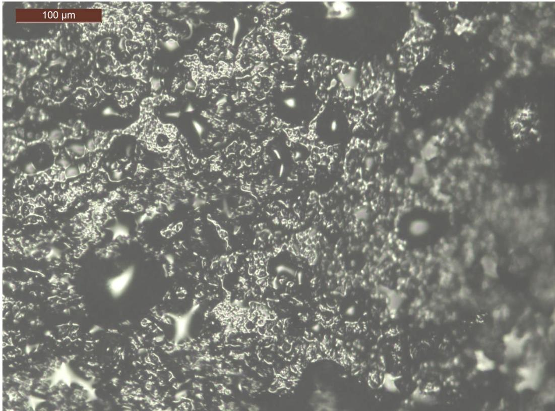
**Figure 3.9: Deposit formed during viscosity measurements at 150 °C on bitumen created between 98 %w/w  $H_2SO_4$  and HVI160B. 100x**
