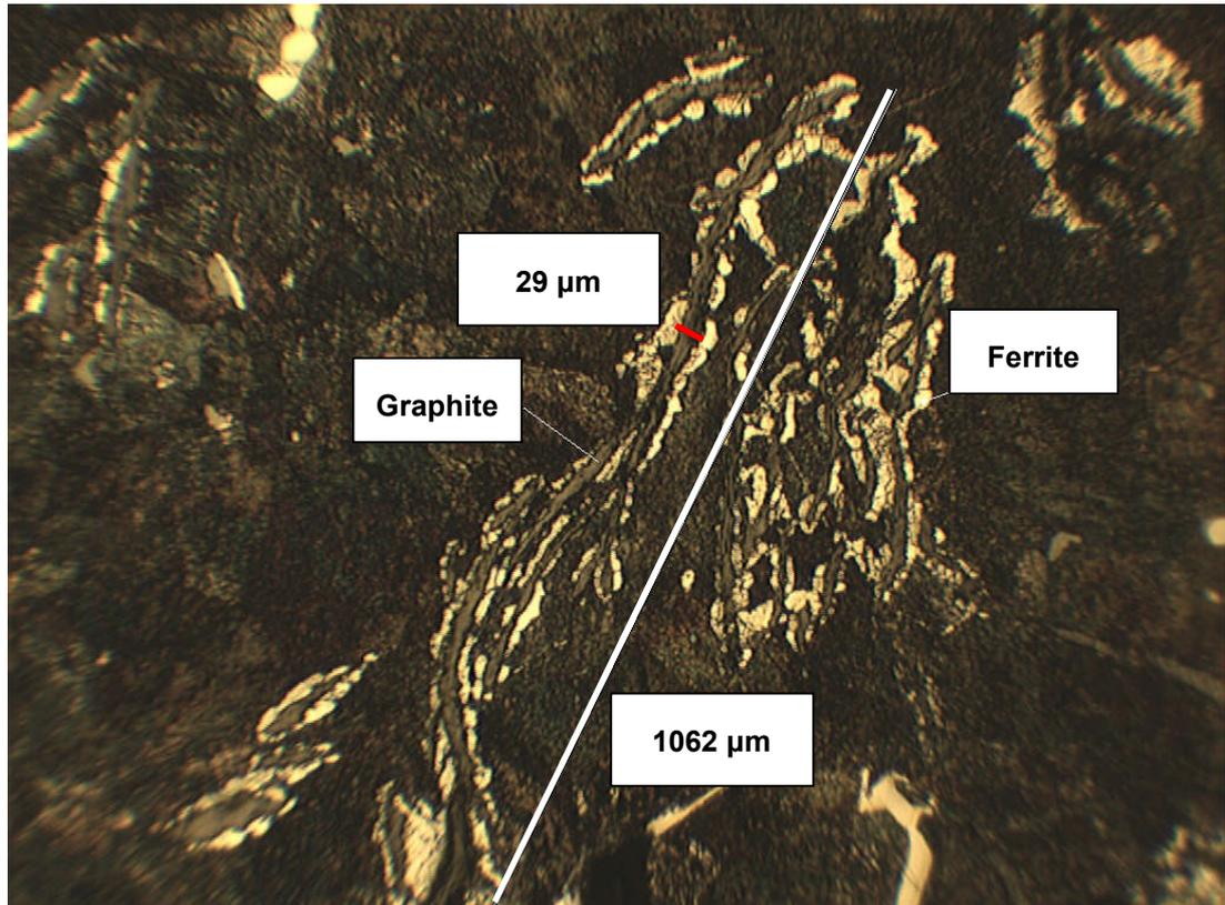
**Figure 6.3: Graphite lamella of a grey cast iron marine cylinder liner**
