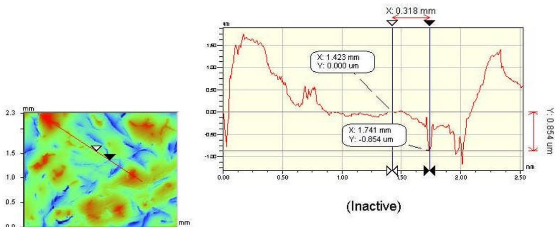
Figure 8.4: Distance between pearlitic matrix and graphite lamella at 300 °C
