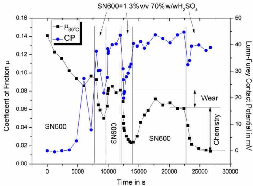
Figure 6: Shuttle test between pure SN600 and SN600+70% $H_2SO_4$  at 80 °C
