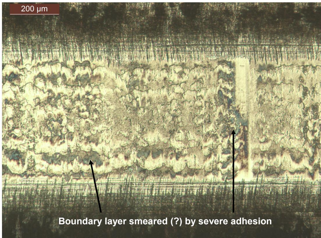
Figure 7.10: Piston ring wear scar, test 13, lubricated with SN600 at 170 °C
