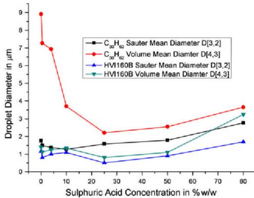
Fig. 6 Statistic evaluation of the droplet size distribution for dispersed H<sub>2</sub>SO<sub>4</sub> in C<sub>30</sub>H<sub>62</sub> and HVI160B; volume and surface rated
