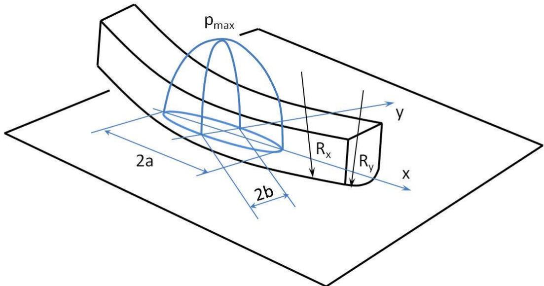
**Figure 6.25: Equivalent elastic piston ring on a rigid plane “cylinder liner” and the resulting semi-elliptical Hertzian contact pressure distribution**
