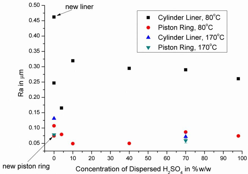
Figure 7.47: Arithmetic average deviation from the mean line,  $R_a$ , for piston ring and cylinder liner
