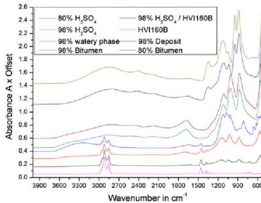
**Fig. 19** FTIR-ATR analysis of reaction products and starting material
