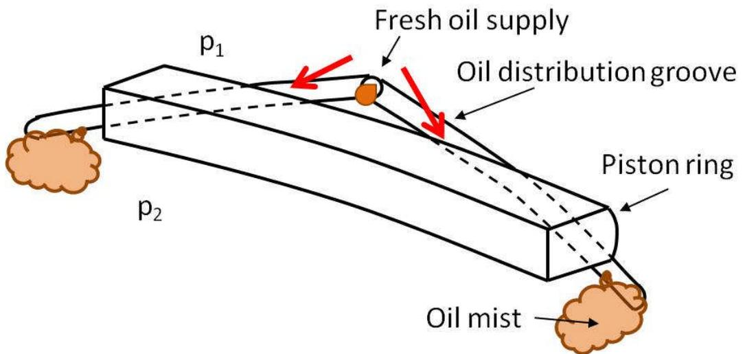
**Figure 1.9: Functionality of the oil distribution groove, shown in Figure 1.8, when gas pressure  $p_1 > p_2$**
