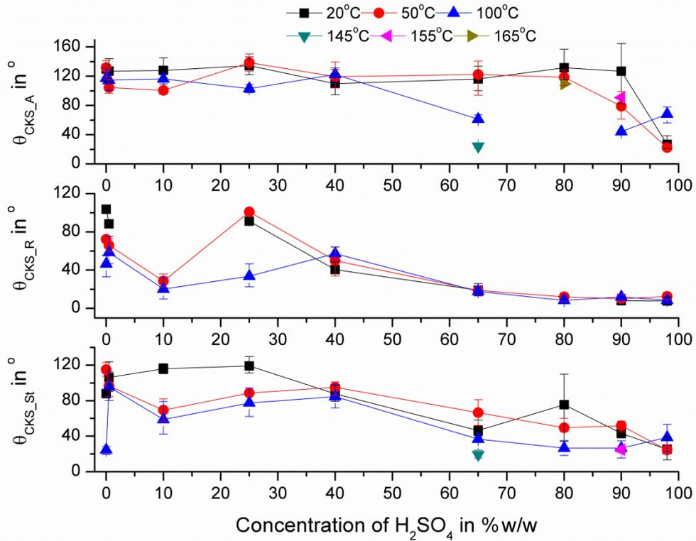
**Figure 5.3: Contact angle measurement results for piston ring chrome coating, CKS, over H<sub>2</sub>SO<sub>4</sub> concentration and at various temperatures**
