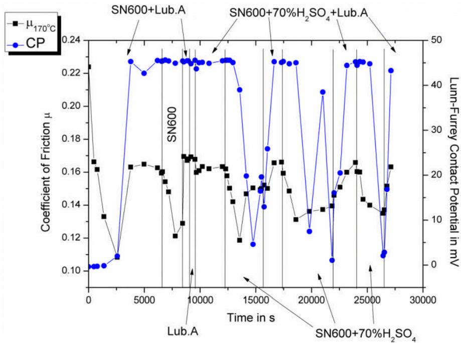
Figure 9: Shuttle test between SN600, lubricant A and 70 %w/w H<sub>2</sub>SO<sub>4</sub>, dispersed in SN600
