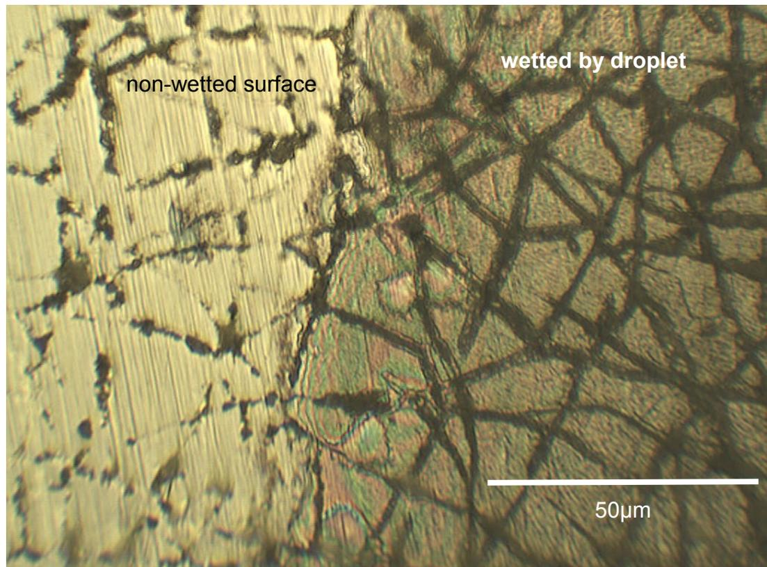
**Figure 5.5: 500x enlargement of CKS coating in contact with 25 %w/w H<sub>2</sub>SO<sub>4</sub> at 100 °C**
