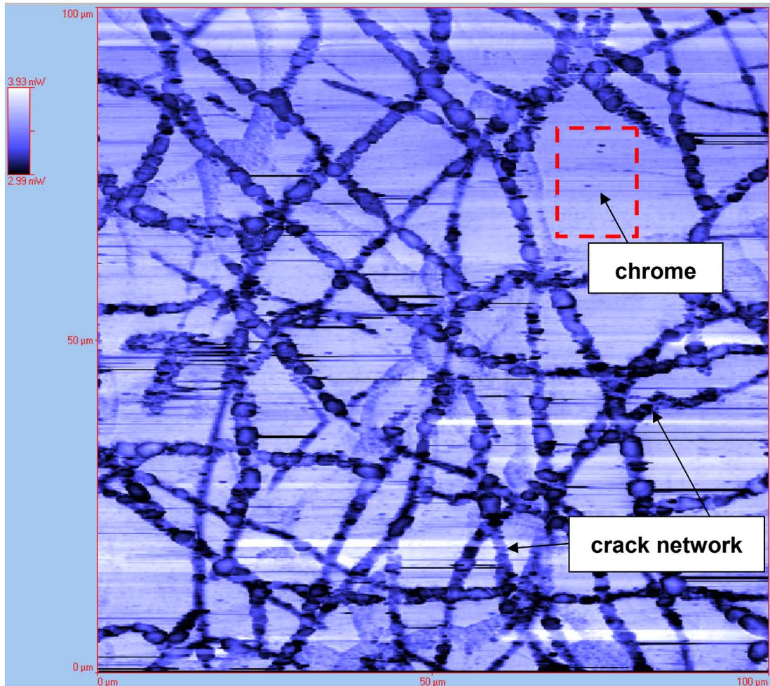
**Figure 8.10: Conductivity contrast picture of electro plated piston ring chrome coating by SThM.**
