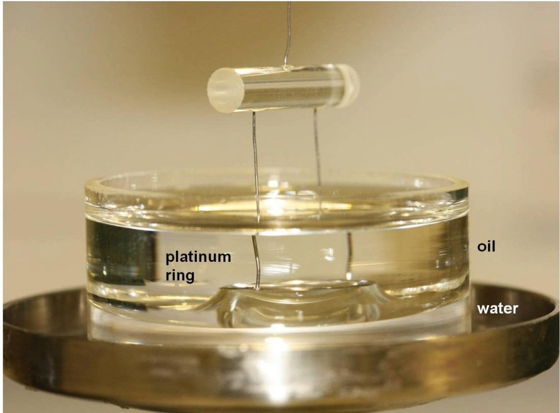
Figure 4.5: Interface between water and squalane during interfacial tension measurement with the Du-Noüy platinum ring
