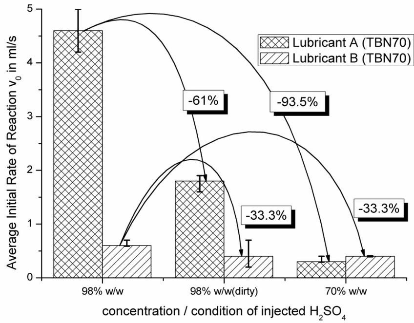
Figure 3.23: Reduction in neutralisation efficiency under varying test conditions
