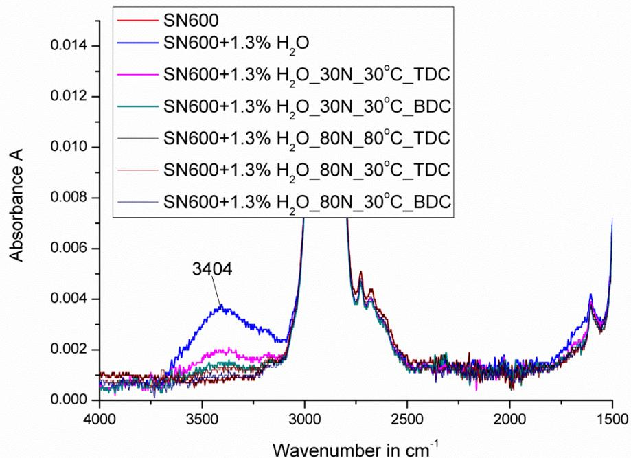
**Figure 7.17: FTIR-ATR spectra of SN600+1.3%v/vH<sub>2</sub>O, fresh and sampled during the friction test at 80 and 30 °C. Test no. 3.**
