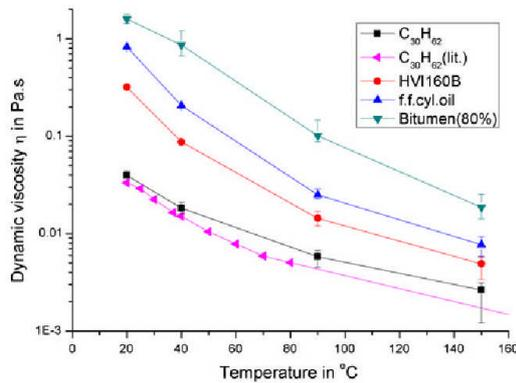
**Fig. 10** Measured viscosity of  $C_{30}H_{62}$  and values found in literature [21], a fully formulated cylinder lubricant, the corresponding base oil HVI160B and the bitumen formed between HVI160B and 80 %w/w  $H_2SO_4$
