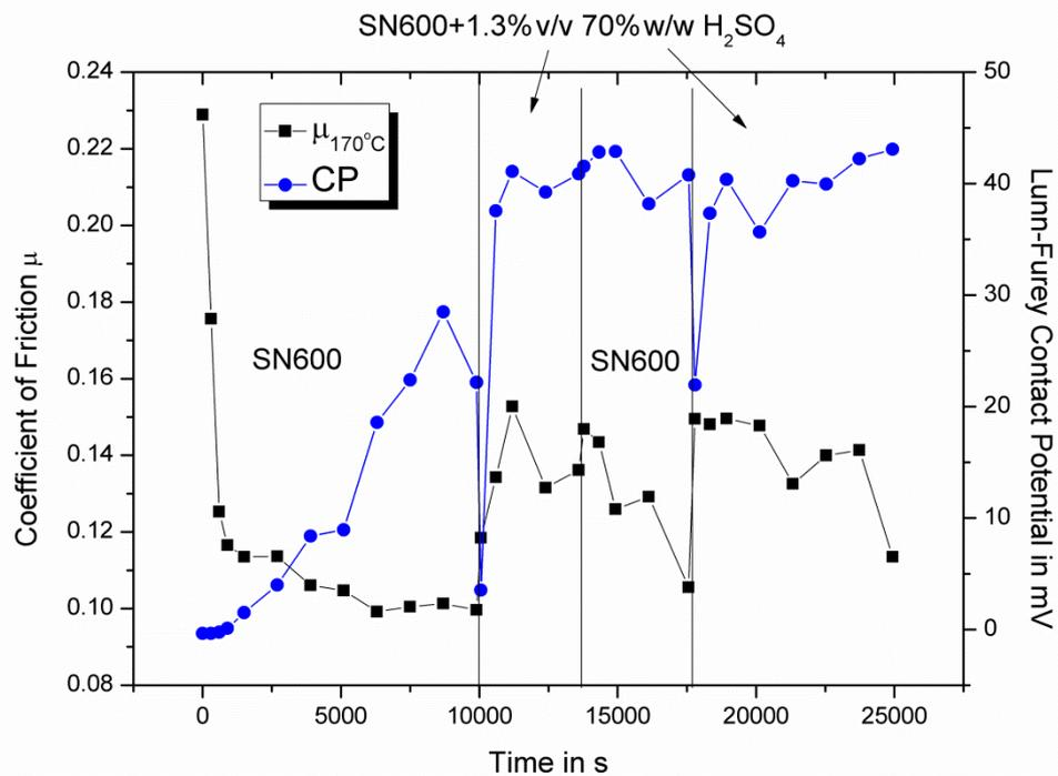
**Figure 7.6: Shuttle test between pure SN600 and SN600 + 70 % H<sub>2</sub>SO<sub>4</sub> at 170 °C showing higher friction due to lubricant degradation**
