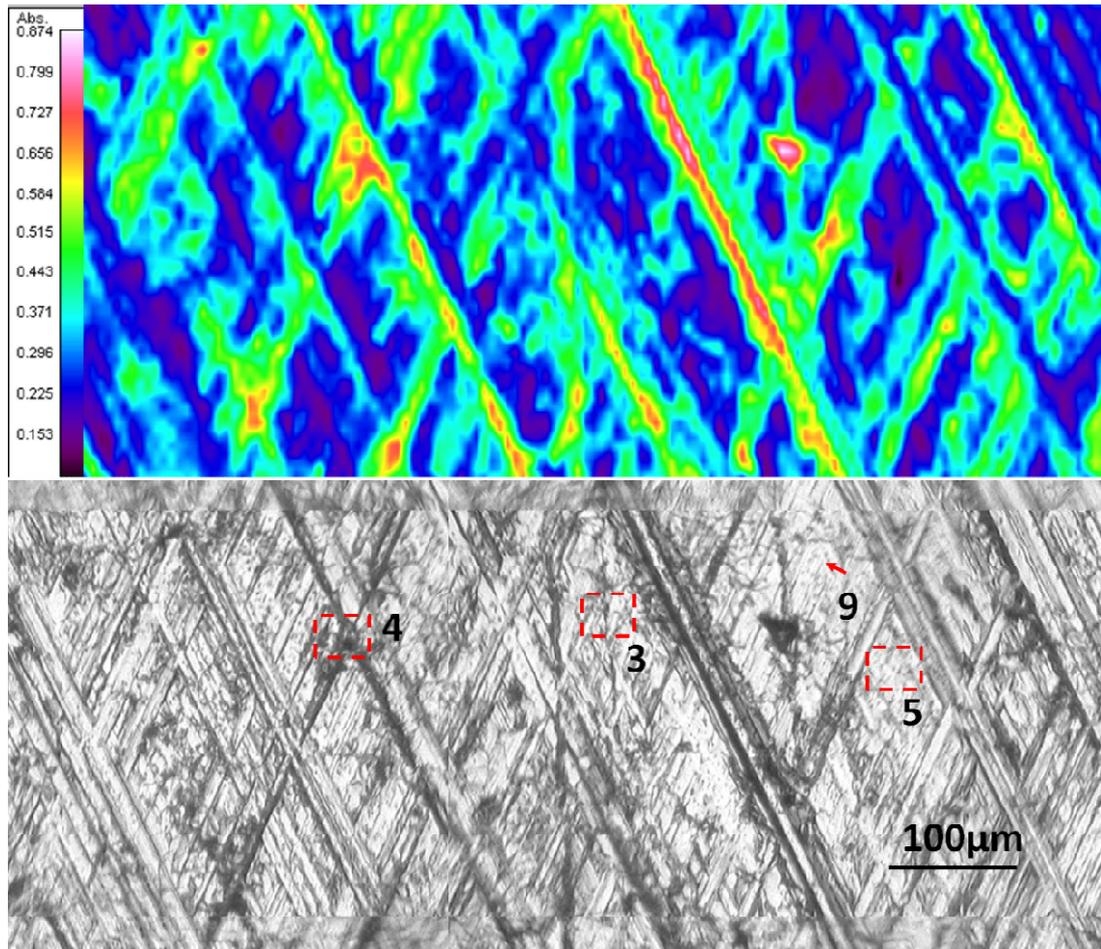
**Figure 7.25: FTIR-scan and visual image on “sample 0”, the unused liner surface**
