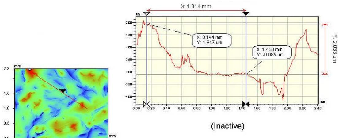
**Figure 8.1: Distance between embossed hard phase and pearlitic matrix at 20 °C**
