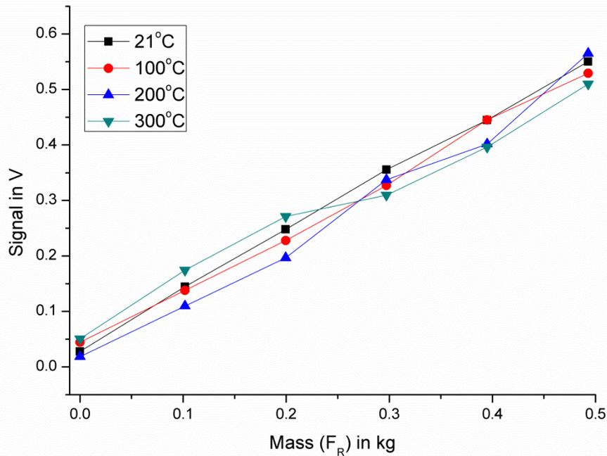
**Figure 6.14: Influence of temperature on the stability of signals from the force transducer**
