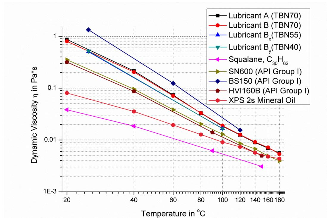
**Figure A.1: Temperature dependent dynamic viscosity,  $\eta$ , for all used lubricants. Measured with cone on plate 1/50 at  $800 \text{ s}^{-1}$  at ambient pressure**
