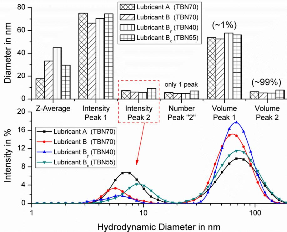
**Figure 3.29: Particle size distribution in fully formulated lubricants by dynamic light scattering**
