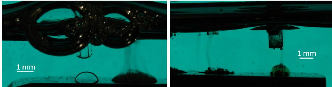
**Figure 5.2: Examples for the contact angle measurements under corrosive conditions. Left: 40 %w/w  $H_2SO_4$  on chrome coating. Right: 80 %w/w  $H_2SO_4$  on grey cast iron**
