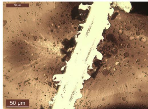
**Fig. 22** Deposit formed at 300 °C with bitumen created with 98 %w/w H<sub>2</sub>SO<sub>4</sub>. Magnification: ×200
