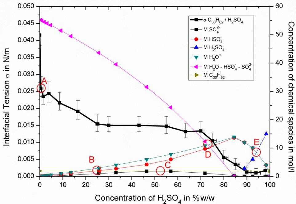
**Figure 4.9: Results of interfacial tension measurements between squalane and sulphuric acid ( $\sigma_{C_{30}H_{62}/H_2SO_4}$ ) at 21 °C in comparison to molecular concentration of species in the acid phase, according to (Young, et al., 1959)**
