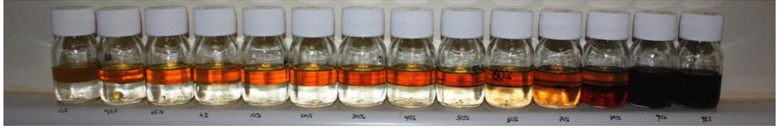
Figure 3.36: API Group I base oil HVI160B in contact with various concentrations of aqueous  $H_2SO_4$ , rising from 0 to 98 %w/w. From left: 0, 0.5, 1.5, 4, 10, 20, 30, 40, 50, 60, 70, 80, 90 & 98 %w/w
