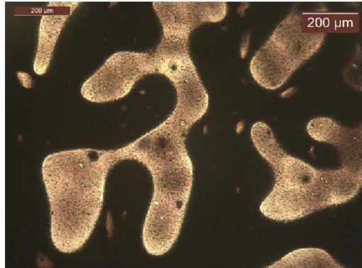
**Fig. 18** Microscopic view on bituminous matter formed between 98 %w/w H<sub>2</sub>SO<sub>4</sub> and HVI160B after separating from oil phase in water. Squeezed between glass slides. Magnification: ×50
