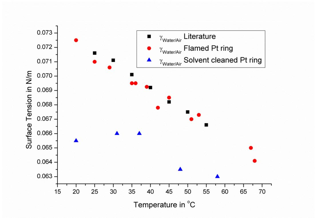
Figure 4.6: Impact of cleaning procedure on the accuracy of interfacial tension measurements with the Du-Noüy ring method on the example of water to air
