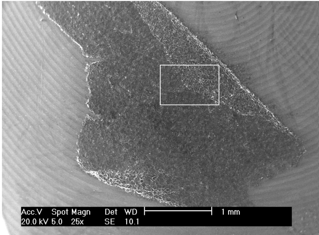
**Figure 3.10: SEM picture; overview of solid reaction product created between 80 %w/w  $\text{H}_2\text{SO}_4$  and  $\text{C}_{30}\text{H}_{62}$  at 165 °C**
