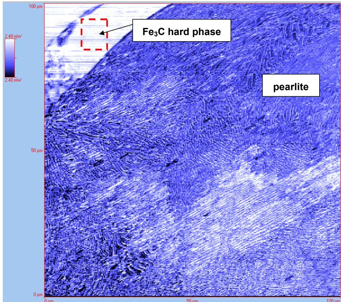
**Figure 8.11: Conductivity contrast picture of highly polished and etched grey cast iron cylinder liner material including a hard phase and pearlitic matrix by SThM.**
