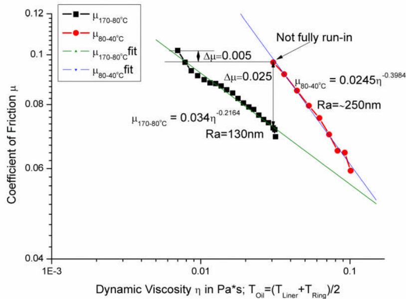
**Figure 3: Influence of viscosity on the COF, measured by dropping the temperature on a run-in surface.**
