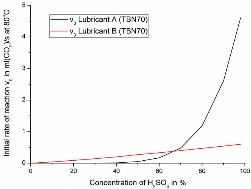
Figure 3.26: H<sub>2</sub>SO<sub>4</sub> concentration dependent initial rate of reaction
