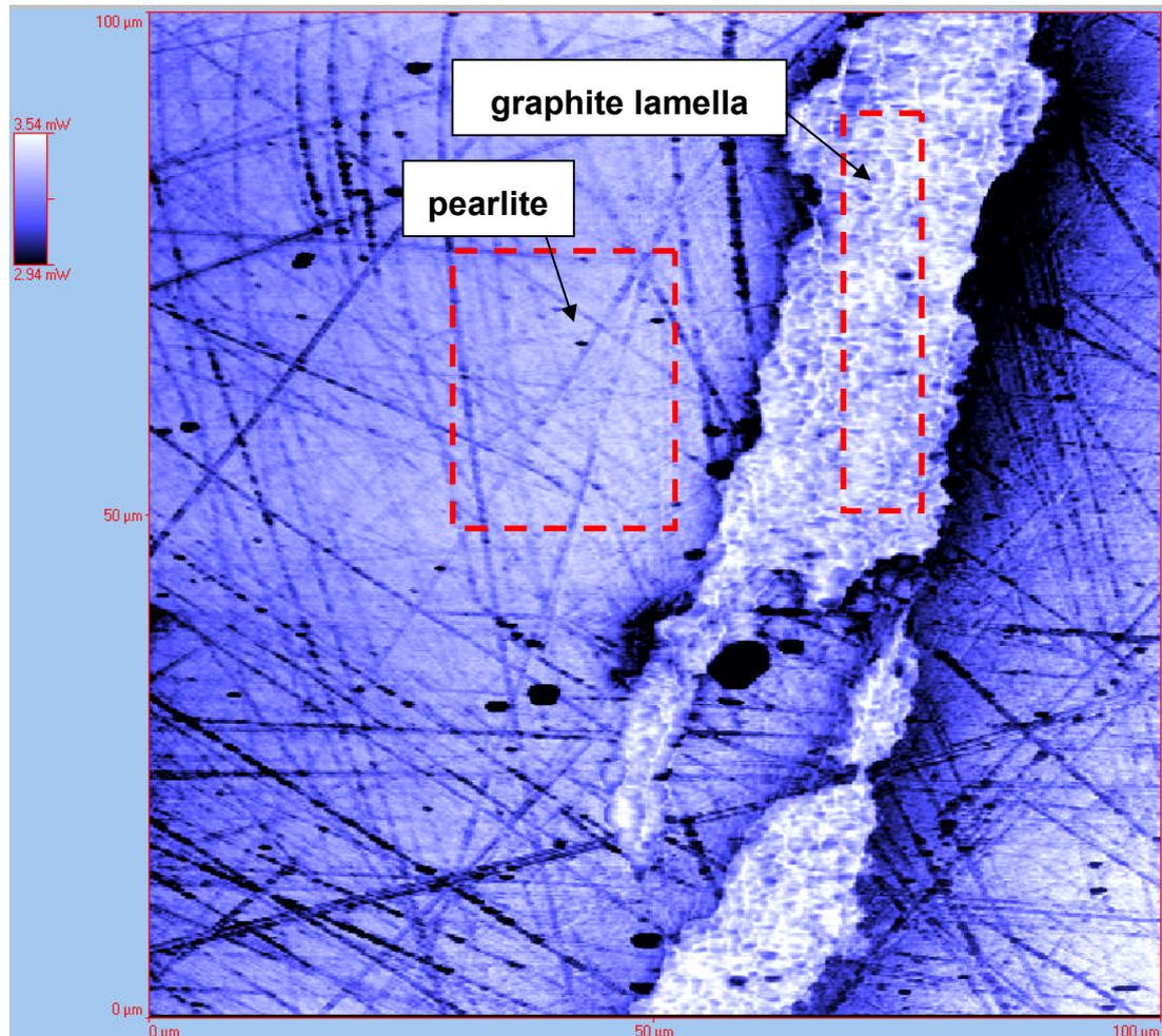
**Figure 8.13: Conductivity contrast picture of polished grey cast iron cylinder liner material including a graphite lamella by SThM.**
