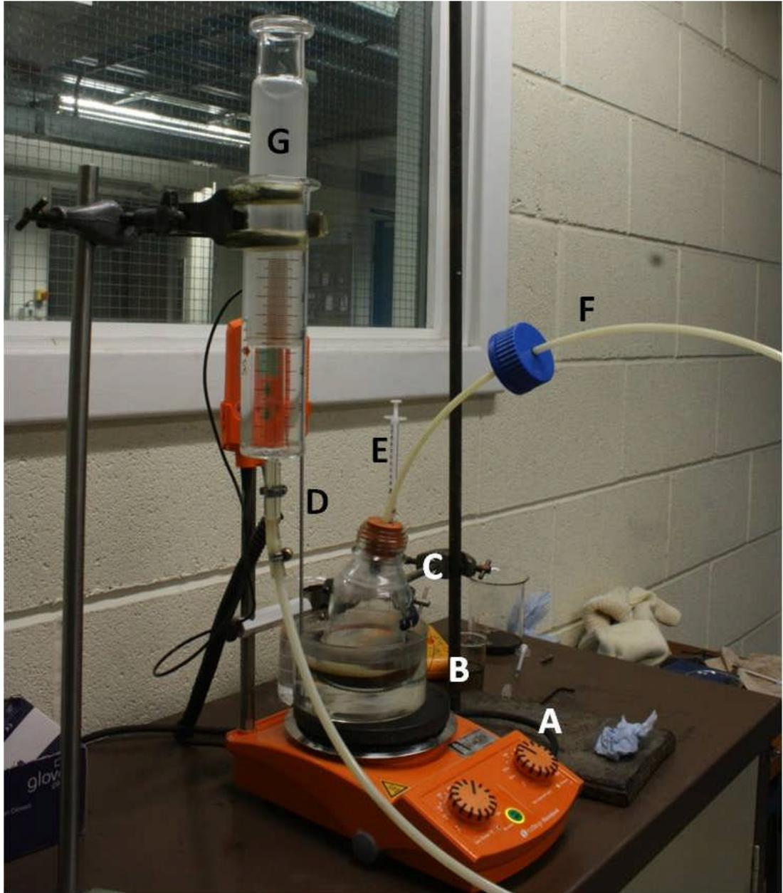
**Figure 3.2: Neutralisation efficiency, volumetric measurement arrangement**
