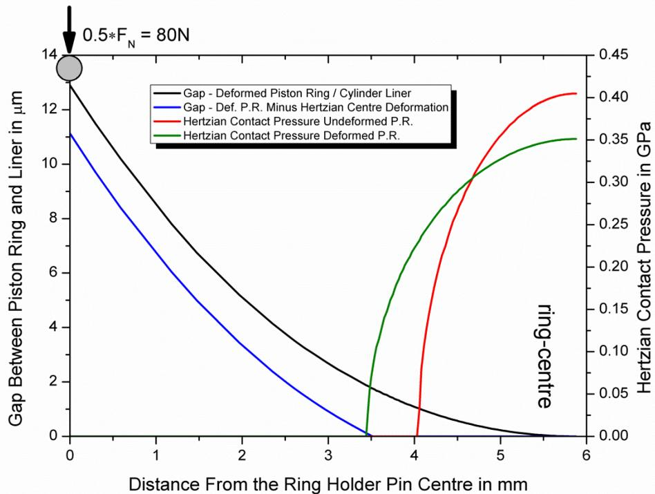
**Figure 6.26: Influence of piston ring deformation on the Hertzian contact pressure and conformity of the parts in unworn condition on the TE77 test bed**
