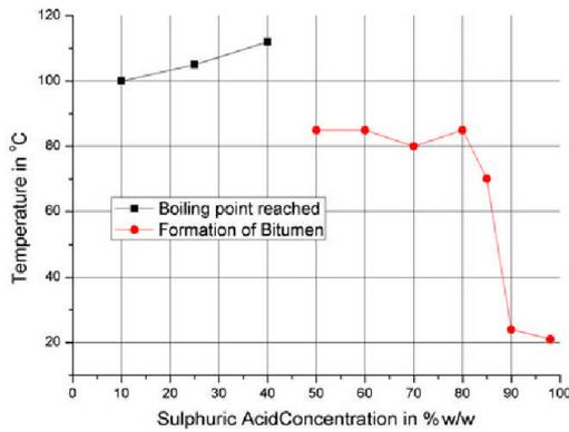
**Fig. 15** Fast heating of API Group I base oil HVI160B in contact with various concentrations of aqueous H<sub>2</sub>SO<sub>4</sub> until bitumen is formed
