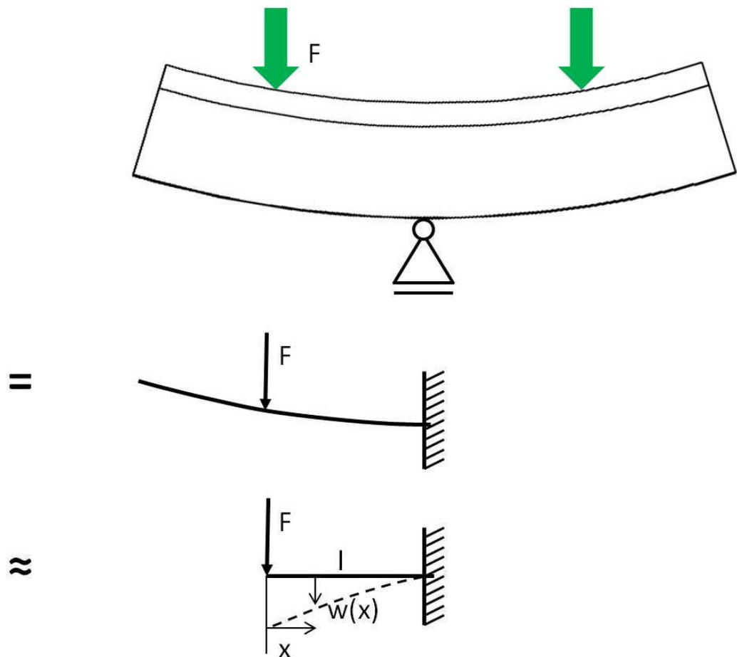
**Figure 6.22: Deformation model of the piston ring in the TE77 holder**
