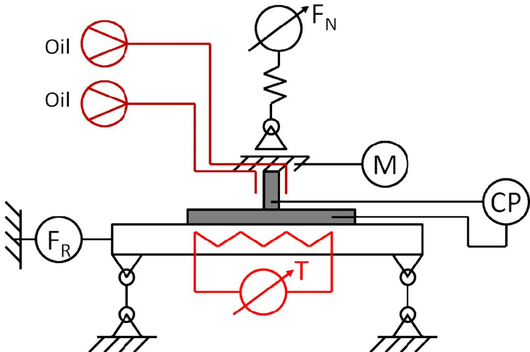
Figure 6.9: Block diagram of the TE77 friction testing machine
