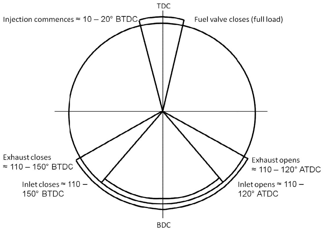
**Figure 1.4: Timing of the 2-stroke cycle (Woodyard, 2004)**
