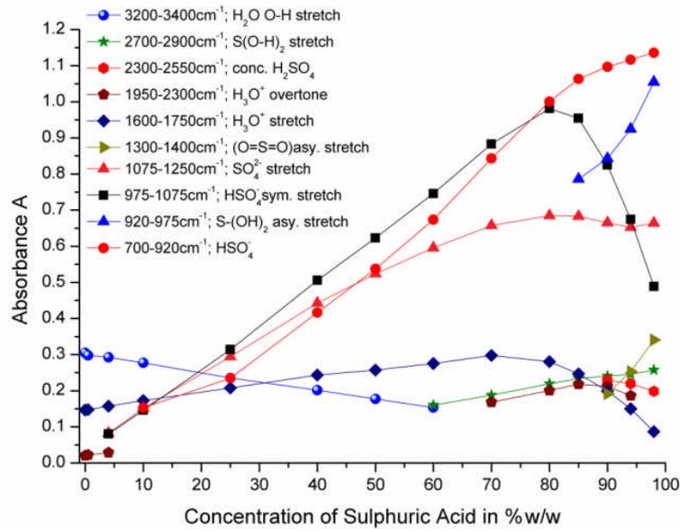
Figure 2: FTIR-ATR absorbance in correlation to the concentration of  $H_2SO_4$
