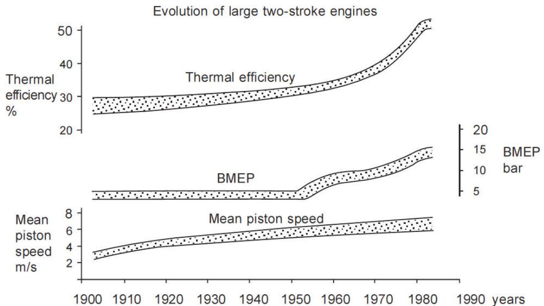
**Figure 1.1: Evolution of large 2-stroke engines, (Woodyard, 2004)**
