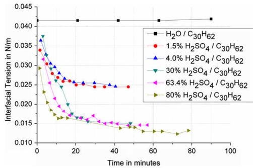
Fig. 1. Time dependent development of interfacial tension between aqueous concentrations (% w/w) of  $\text{H}_2\text{SO}_4$  and  $\text{C}_{30}\text{H}_{62}$ .
