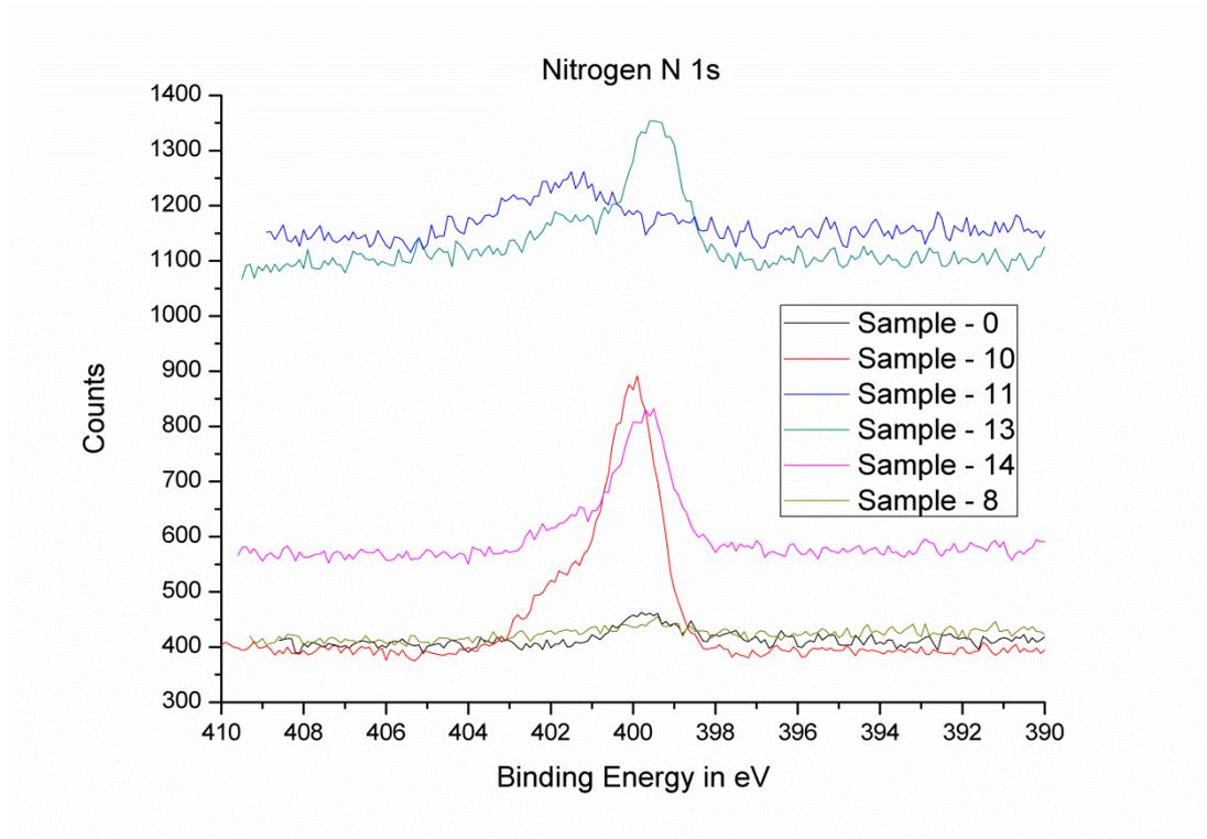
**Figure 7.41: N1s XPS spectra for all cylinder liner wear scars**
