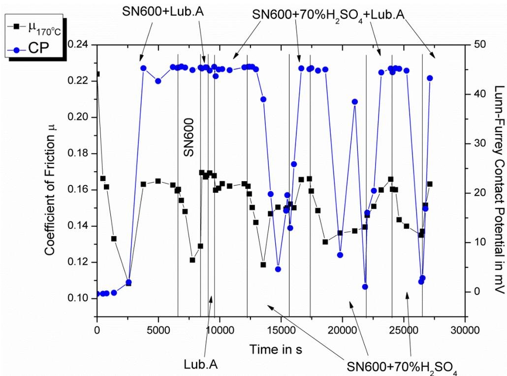
**Figure 7.8: Shuttle test between SN600, lubricant A and 70 %w/w  $\text{H}_2\text{SO}_4$  dispersed in SN600 at 170 °C revealing the influence of lubricant additive on friction.**
