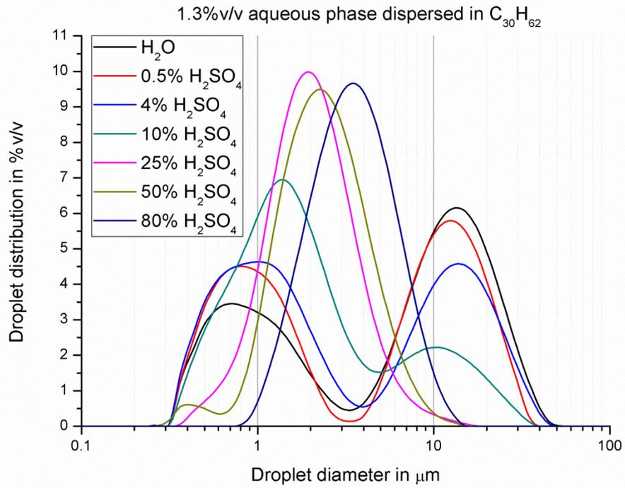
**Figure 3.18: Droplet size distribution of 1.3 %v/v aqueous H<sub>2</sub>SO<sub>4</sub> dispersed in C<sub>30</sub>H<sub>62</sub>**
