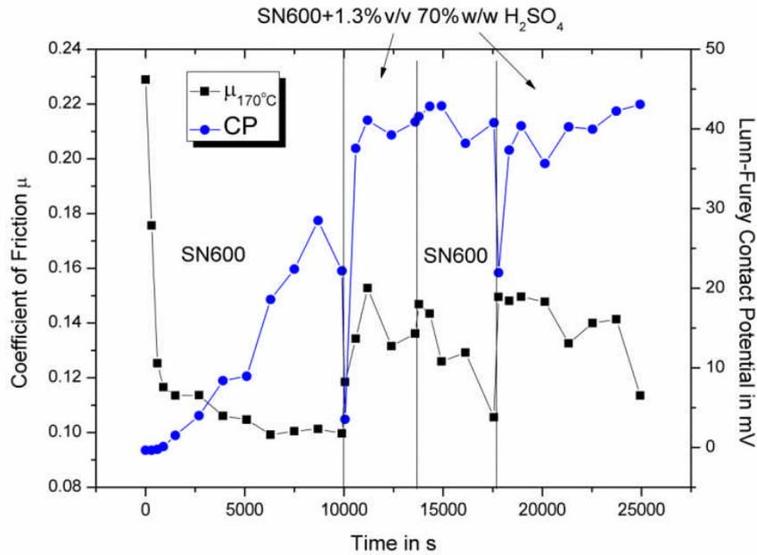
Figure 7: Shuttle test between pure SN600 and SN600+70% $H_2SO_4$  at 170 °C
