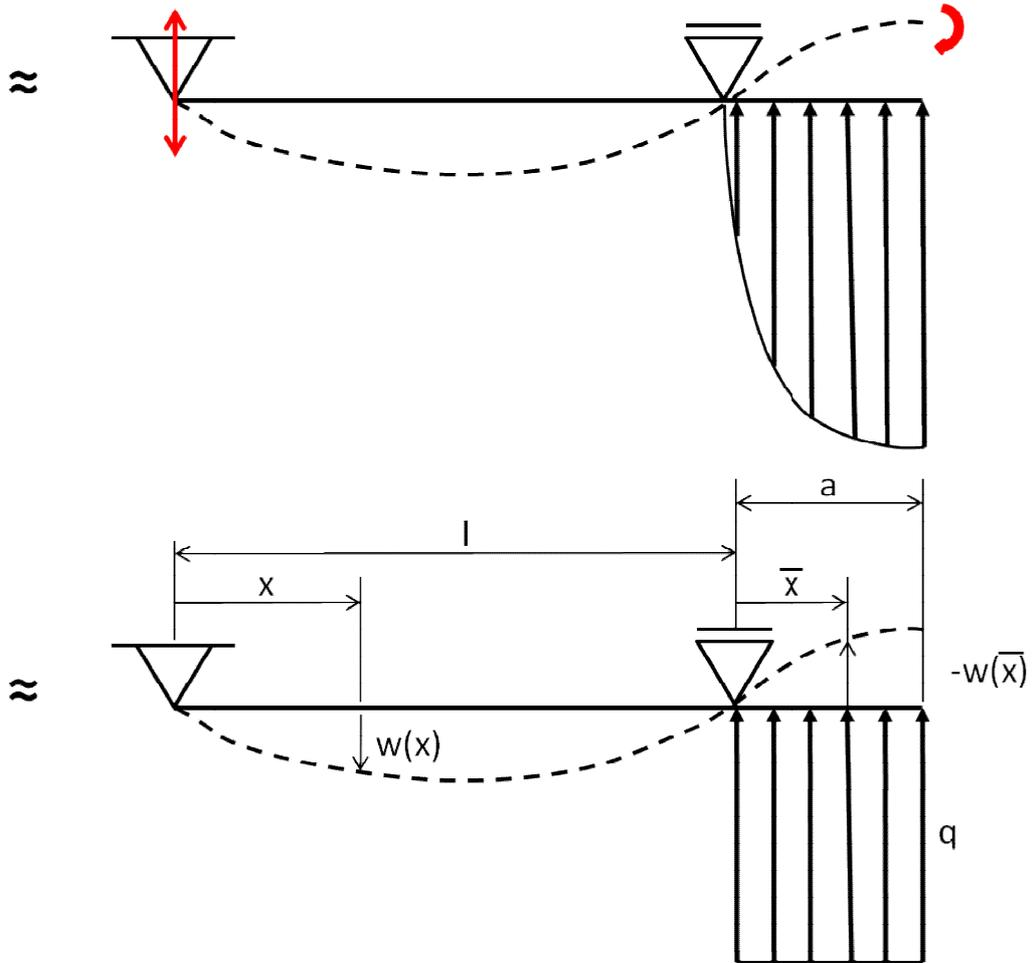
Figure 6.27: First approach to piston ring deformation with Hertzian contact pressure
