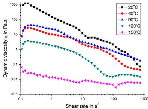
**Fig. 11** Viscosity of bitumen formed between HVI160B and 98 %w/w  $H_2SO_4$ . See text for encountered difficulties
