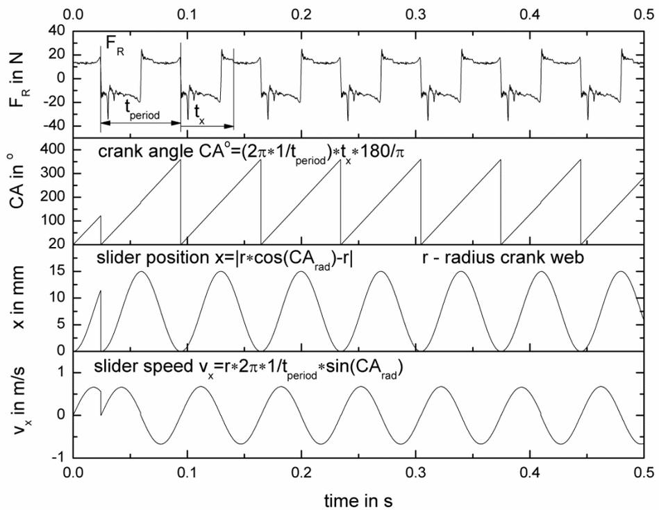
**Figure 6.19: Use of the signal from the force transducer to establish the kinetics of the measurement**
