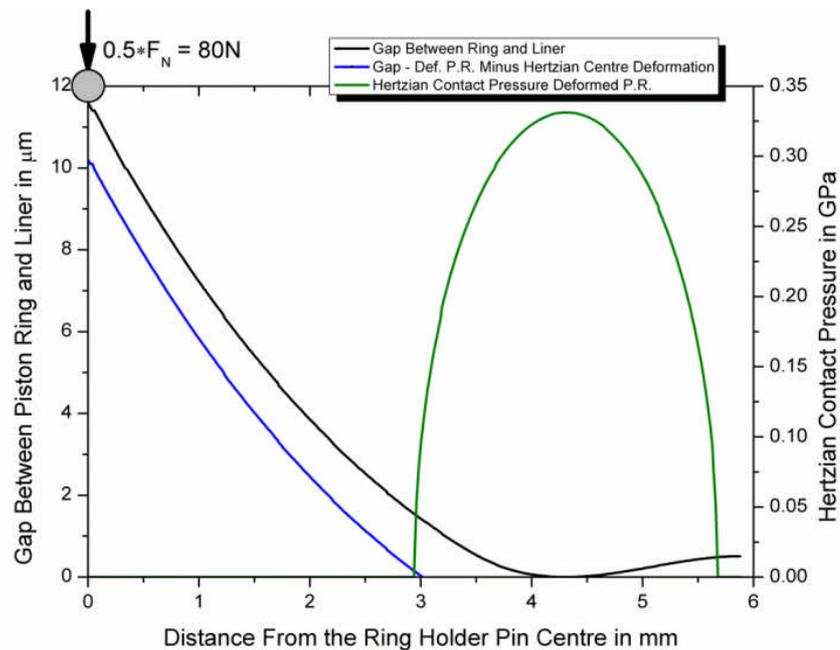
**Figure 1: Influence of piston ring deformation on the Hertzian contact pressure and conformity of the parts in unworn condition on the TE77 test bed.**
