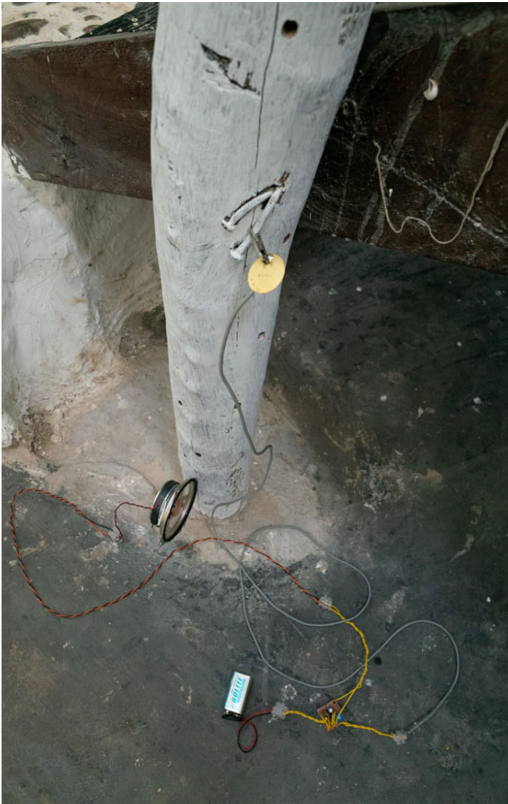
Figure 24 Wood beetle. Piezo contact microphone clipped to metal nail. Battery powered self-made audio amplifier. Audio loudspeaker. Doi Saket, Thailand 2013
