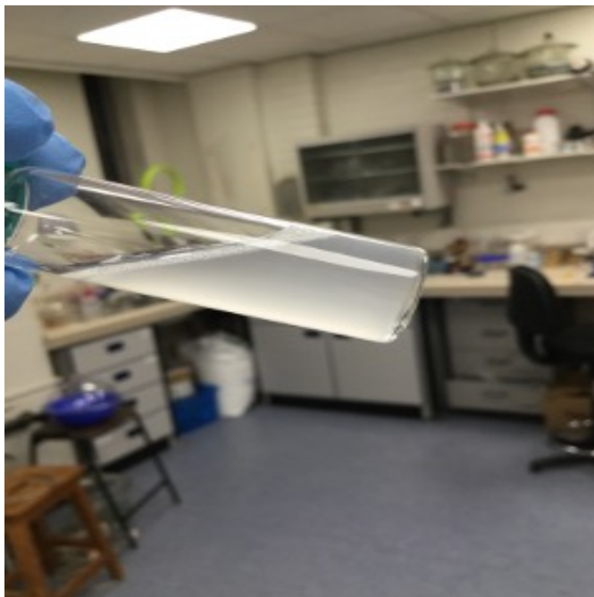
Figure 3.2: Aggregates forming in a a mixed solution of PDMS and PFPE-PEO in THF
