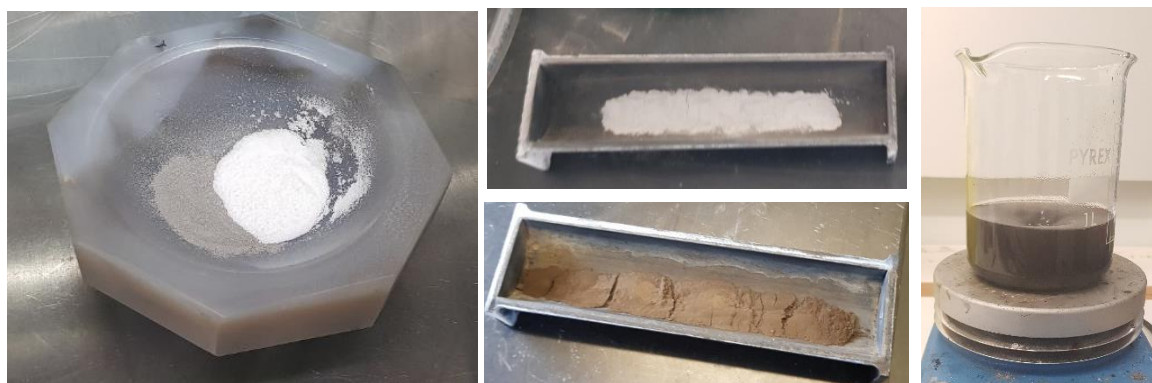
Figure 3.1: A) Magnesium and silica powders in an agate mortar. Stainless steel crucible containing B) magnesium and silica before heating, and C) after heat treatment. D) Sample in 1M HCl after heat treatment.
