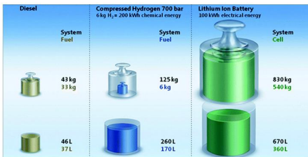
Figure 1.3: The diagram illustrates the difference in energy densities of different energy storage medium in vehicles. Image taken from ref 4 .
