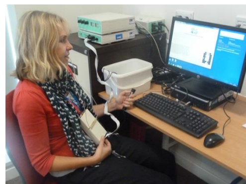
Therapist using the EPG system with EPG plate in her mouth
