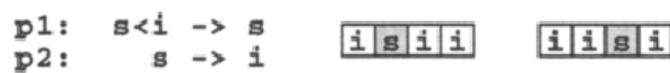
Figure 2.18.: Productions used to obtain signal propagation, along with their CA interpretation. taken from, [75, fig.6, p. 201].
