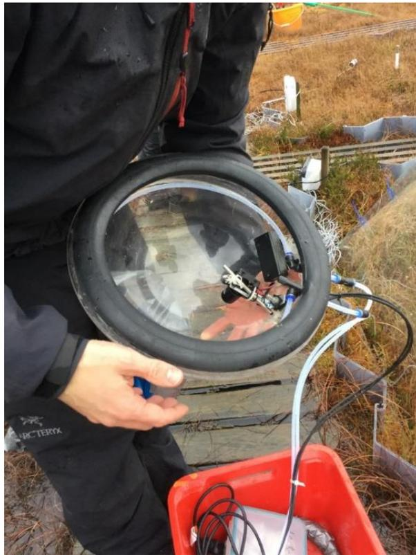
**Figure 2.7.** Photograph of inside of flux chamber used when measuring greenhouse gas fluxes.
