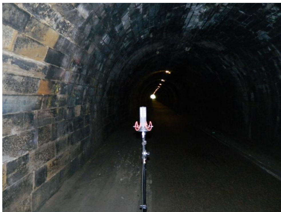
FIGURE 2.2: A Practical Example of Recording an Impulse Response of the Innocent Railway Tunnel [7]
