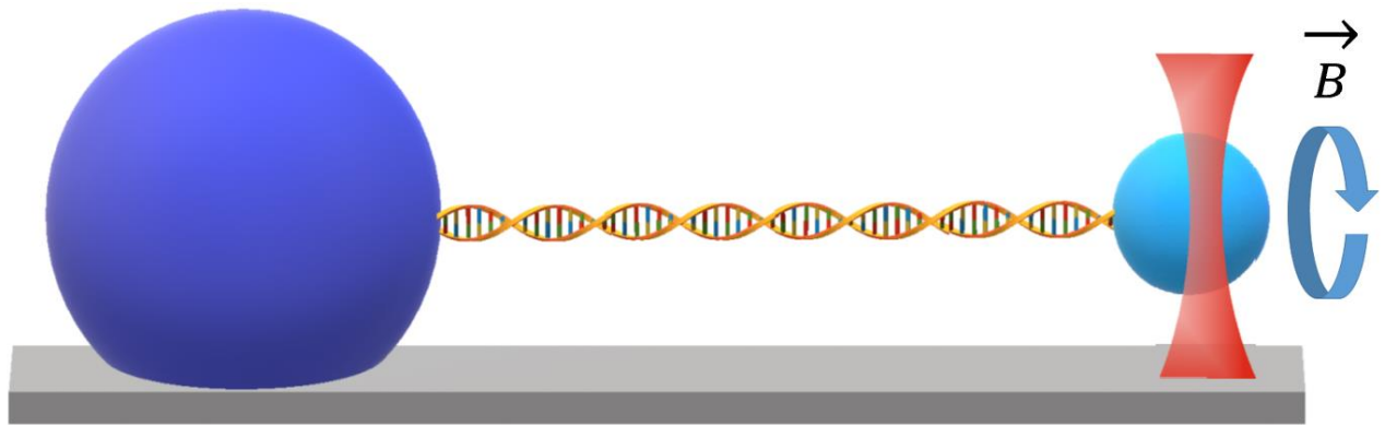
Figure 20: Cartoon of the magneto-optical tweezers experiment configuration. The AntiDig-covered anchor bead in dark blue, magnetic trapped bead in light blue, dsDNA tether in between. The optical trap is symbolized in red, and the Rotating blue arrow symbolizes the oscillating magnetic tweezers.
