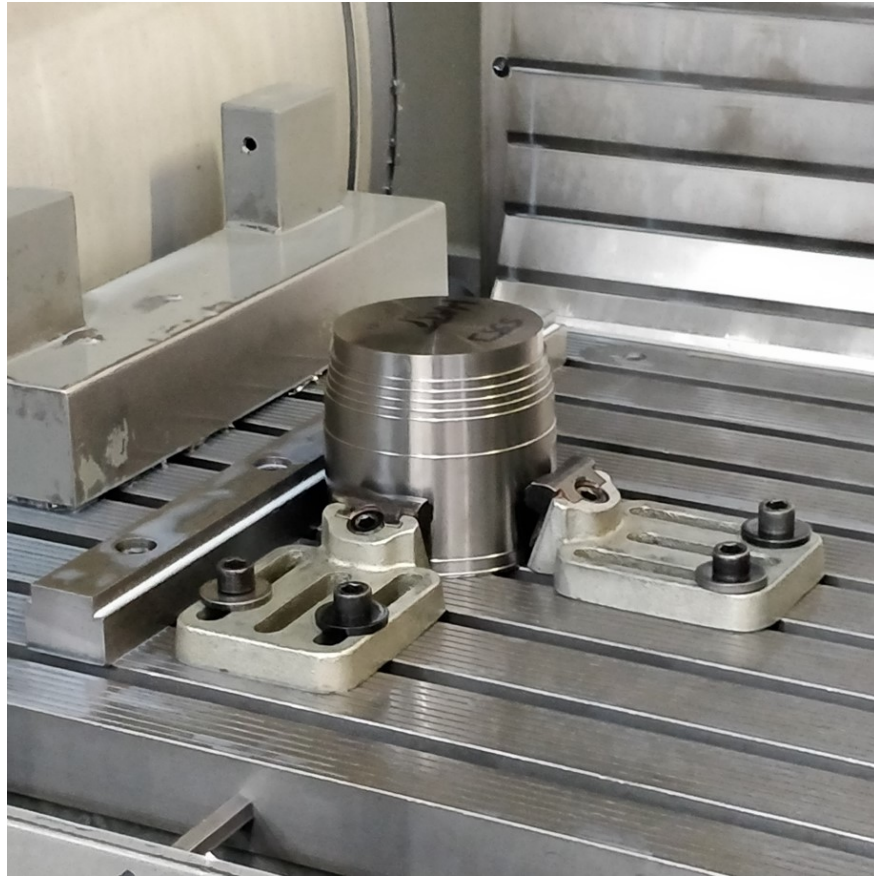
Figure 4.9: Photograph of Ti-5553 billet clamped within the DMU 100 monoBLOCK machining centre before drilling.
