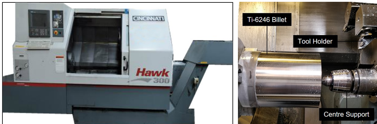
Figure 4.1: A photograph of the Hawk-SL 300 lathe including the Ti-6246 workpiece, centre support, tool holder and insert.
