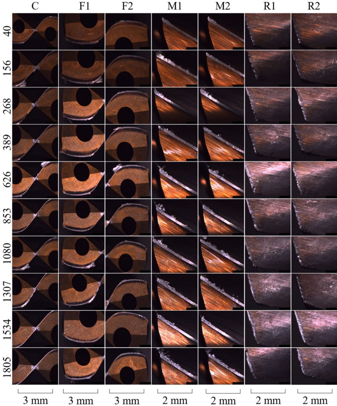
Figure 6.4: Photographs showing the tool wear at the corresponding hole number (on the left), for the chisel (C), flank 1 (F1) and flank 2 (F2), margin 1 (M1) and margin 2 (M2), rake 1 and rake 2 (R1 and R2).
